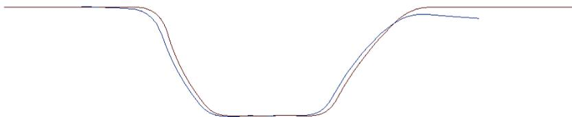
**Figure 4** Section 1, desired shape of the sheet and shape after first springback iteration
