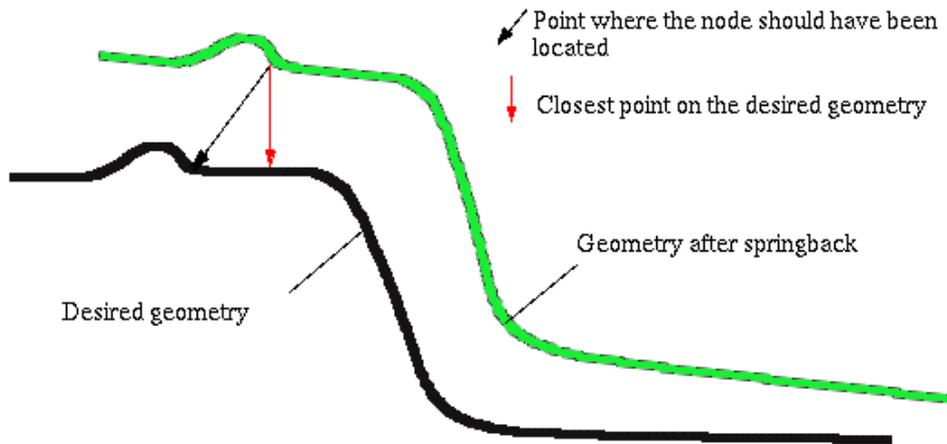
**Figure 1** Problem with measuring deviation between different geometries
