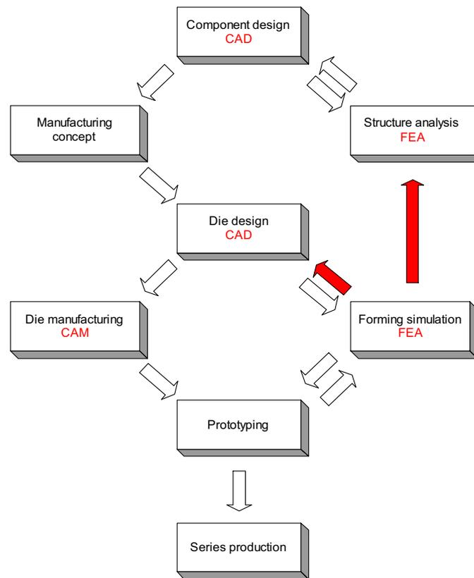
**Figure 1** A diagrammatic representation of the process chain of the development of a component
