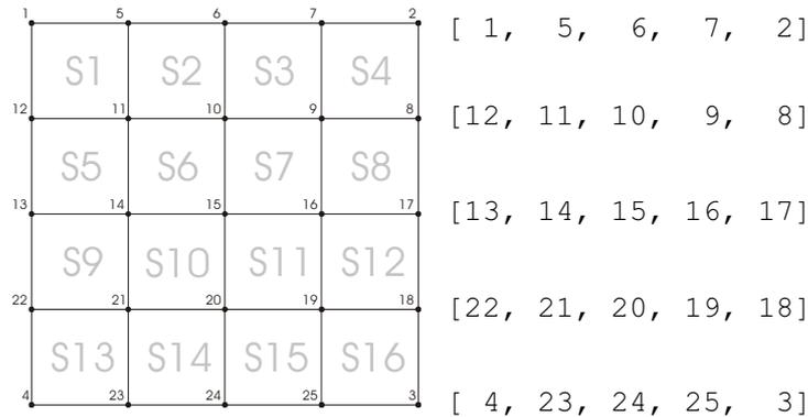
**Figure 3** The determination of the point rows (where S' = element number)
