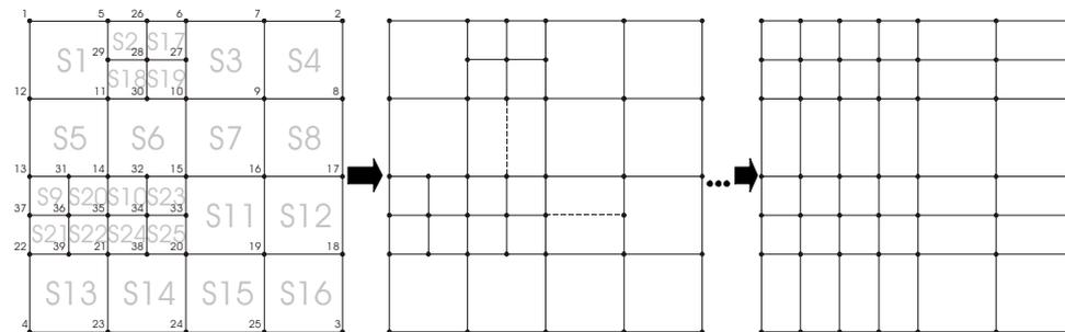
**Figure 4** The stages in the generation of a uniform mesh
