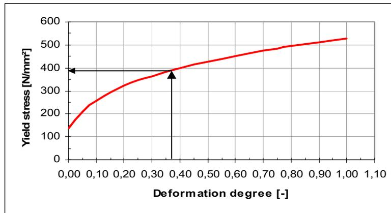
**Figure 10:** Determination of the new yield strength
