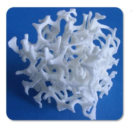
Auxetic Material Negative Poisson's ratio Contracts compression/expands tension Example application: filters
