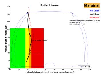
Fig. 14: B-pillar Intrusion Plot
