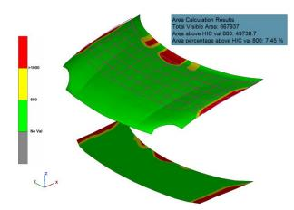
Fig. 5: HIC values interpolated on the bonnet. Raster area projected on Z = 0. Area calculation for HIC values above a threshold.
