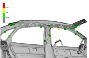
Fig. 10: Circular annotations with HIC values on Target Points
