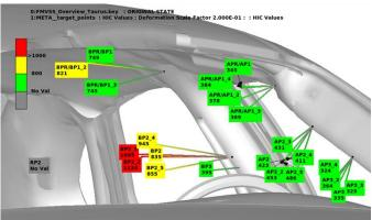
Fig. 11: Lines presenting each hit's trajectory. HIC values displayed in annotations
