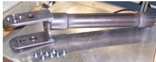
Lower leg bone (hollow inside) + screw 2.0048 kg.
