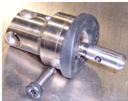
Ankle assembly +screw: 0.771 kg.
