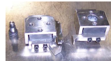
Knee slider assembly + screw 0.4808 kg.
