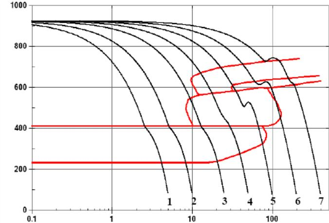
recalculated CCT diagramm
