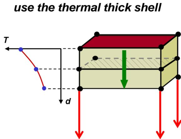
*and add an artificial heat flux to the backside*
