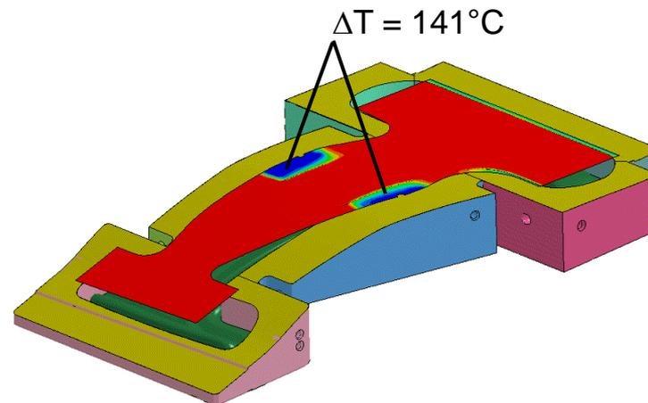
**Tool surface temperature directly affects the heat flux from blank to the die**
