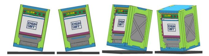
Fig.4: Impact sequence – right, left, rear and front, respectively.
