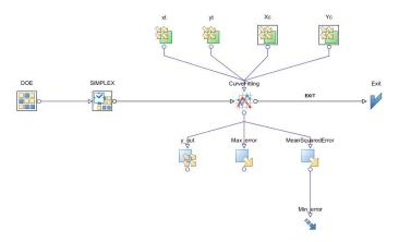
Fig.3: Example of modeFRONTIER workflow used to perform the material calibration
