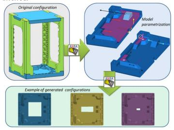
Fig.5: Parametric model of packaging base
