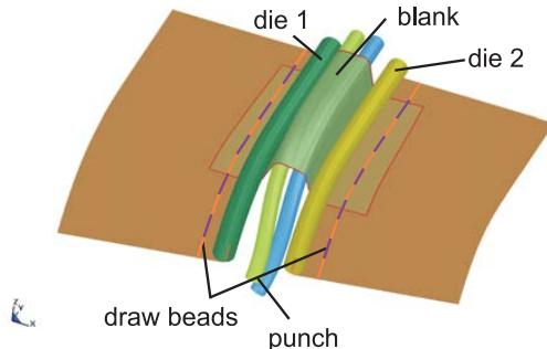
Figure 4: Model of deep drawing process
