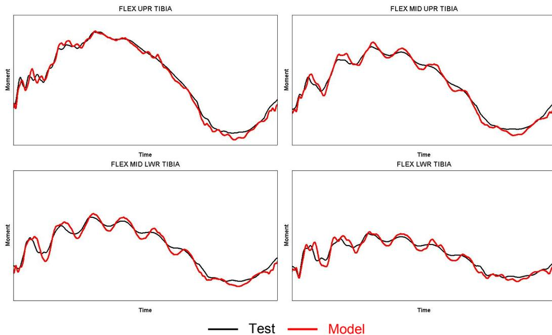
Figure 9: Assembly dynamic calibration tibia moment results
