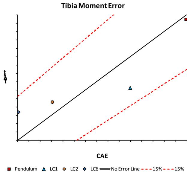
Figure 15: Peak of highest tibia moment error in CAE simulation compared to test values
