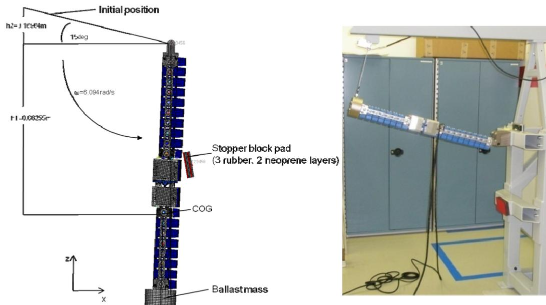
Figure 7: Assembly dynamic calibration setup
