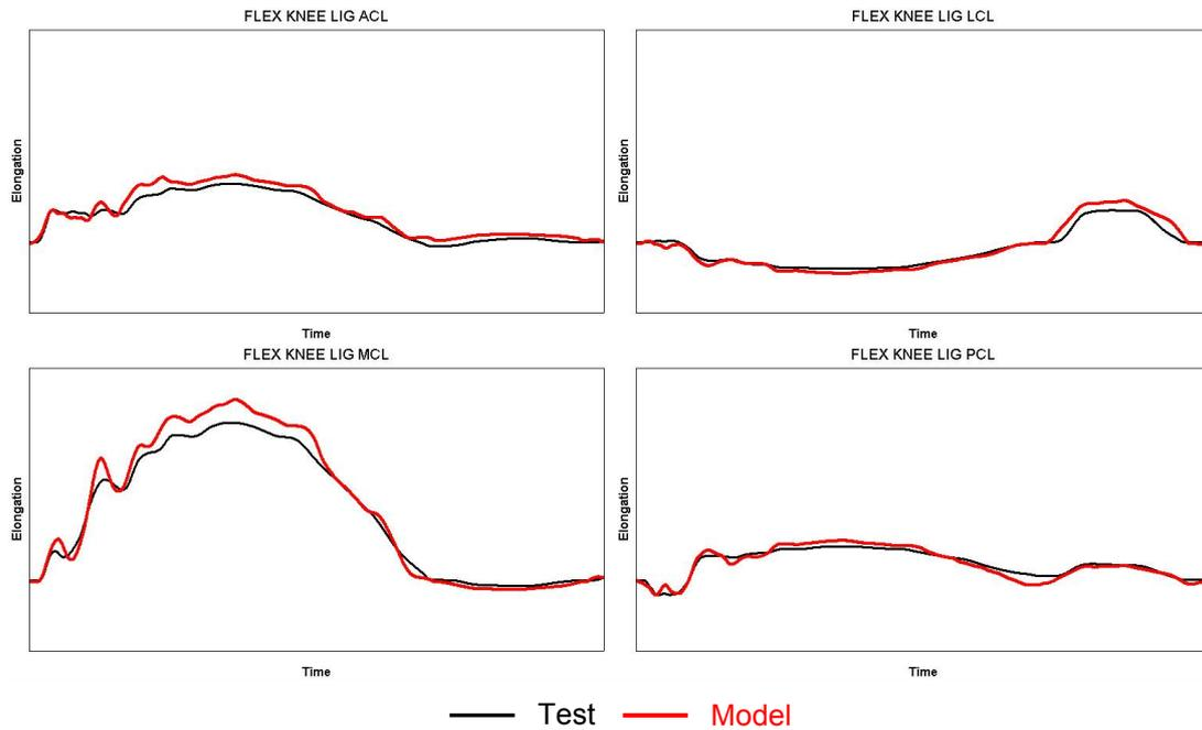
Figure 10: Assembly dynamic calibration knee ligament elongation results
