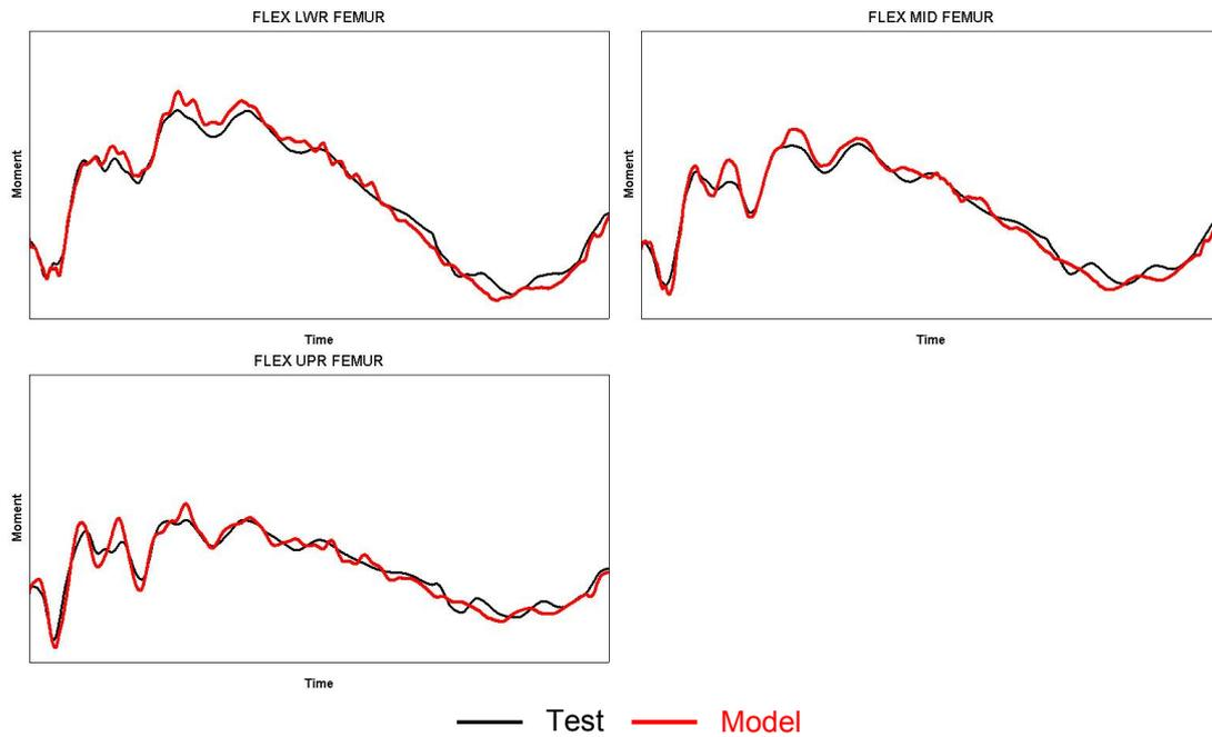
Figure 8: Assembly dynamic calibration femur moment results
