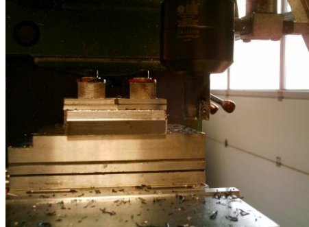
Fig. 2 b) Face milling set-up: workpiece (XC38-Afnor) mounted on Kistler dynamometer, mill tool with two indexable inserts.
