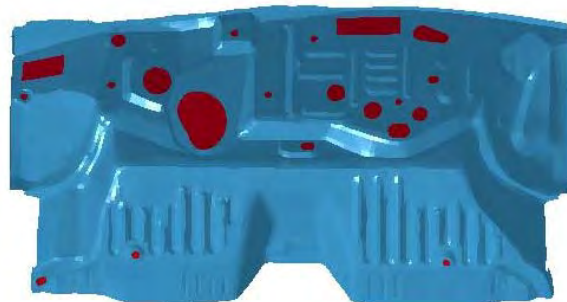
Figure 4 Sheet Thickness Prediction ( t_0=0.75\text{mm} )
