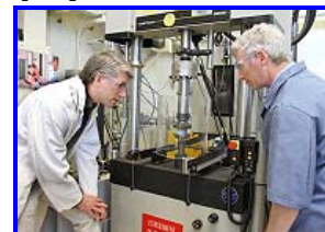
compression test helmet pad
