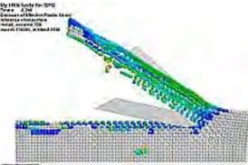
[Metal cutting in LS-DYNA with SPG: Effective plastic strain](#)
