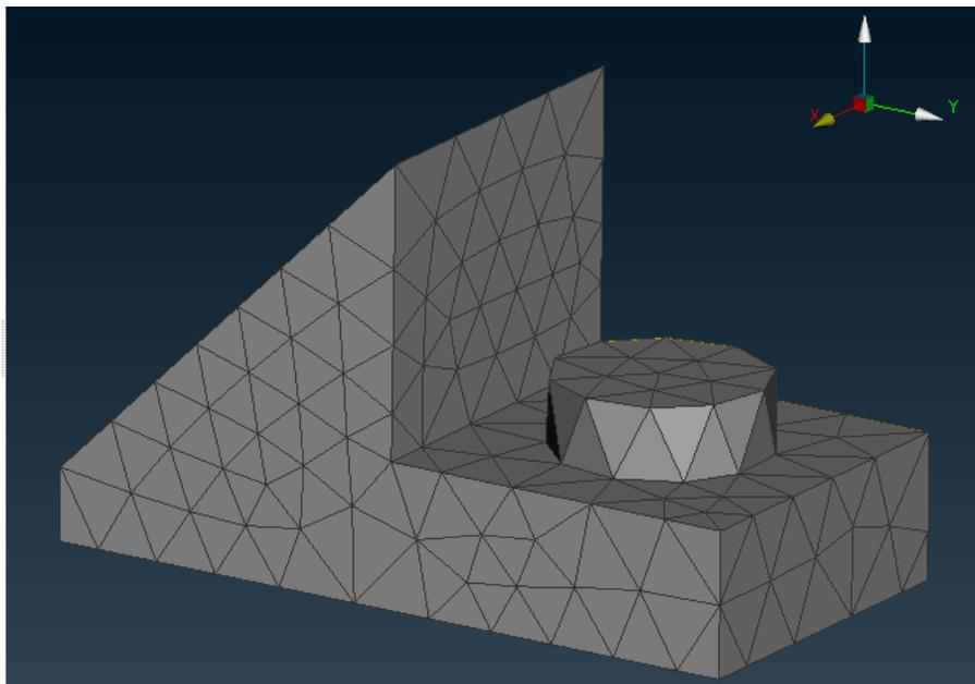
Figure 8: 1mm mesh for brick with ldraw ID:92946
