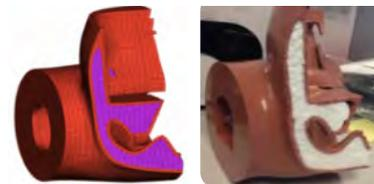
*Comparison of Simulation model and physical prototype of a Humanetics'*
