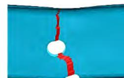
Ductile cracking in shell
