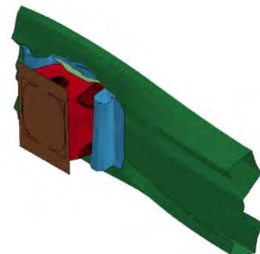
Deformation of crash box and bumper at t = 0 ms (left) and t = 30 ms (right)
