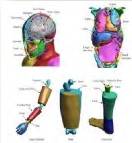
The Total Human Model for Safety, or THUMS®, is a joint development of Toyota Motor Corporation and Toyota Central R&D Labs. Unlike dummy models, which are simplified representation of humans, THUMS represents actual humans in detail, including the outer shape, but also bones, muscles, ligaments, tendons, and internal organs. Therefore, THUMS can be used in automotive crash simulations to identify safety problems and find their solutions.
