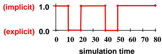
3. Enter the load curve ID as a negative number using the first parameter on the keyword `*CONTROL_IMPLICIT_GENERAL: IMFLAG = (-lcid)`. You may also include any other `*CONTROL_IMPLICIT` keywords that you would like to use during the implicit phases of the simulation.
