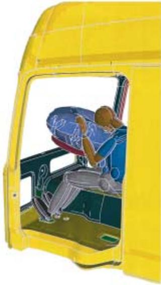
Actros passenger simulation (with **belt and belt-tightener**) for optimal airbag passenger protection.
