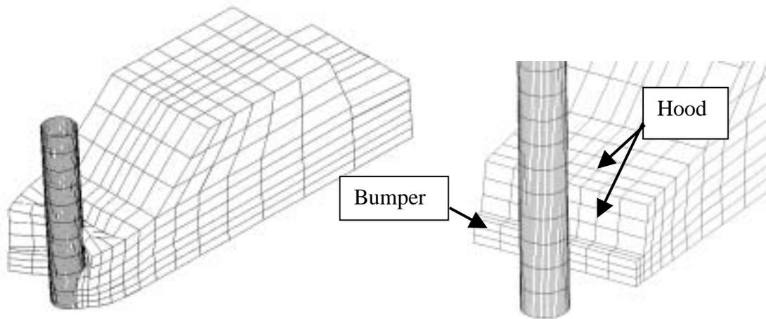
Figure 3 – Small car crash: geometry of deformed (50ms) and undeformed shape
