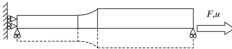
Figure 4 – Quarter symmetric model of test specimen
