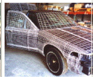
Figure 2 - Vehicle Discretization Phase II of Digitization.
