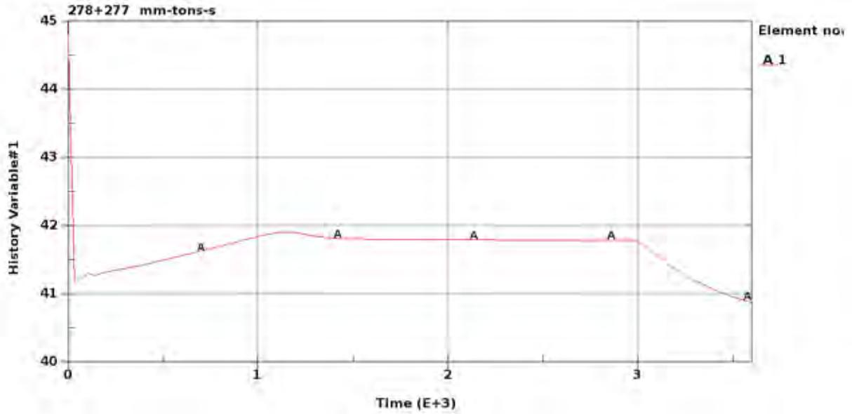
Figure 6 The braid angle of fiber during tension and curing test
