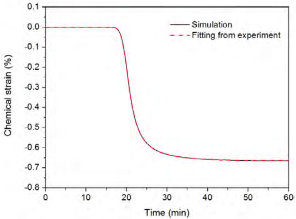
Figure 3 Chemical strain of MAT277 single element test
