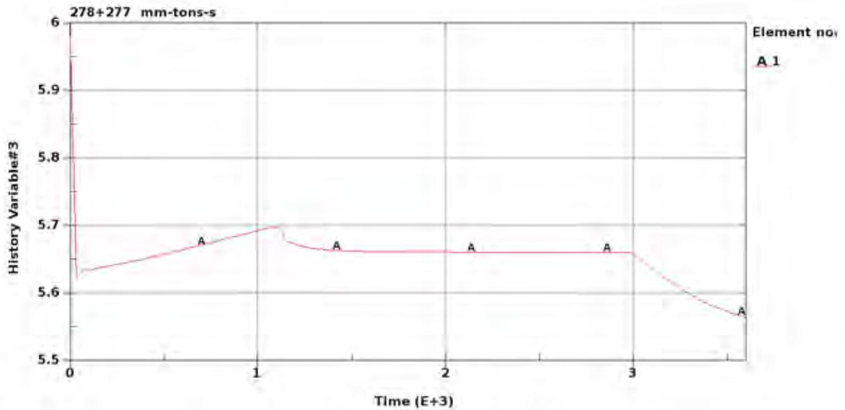
Figure 7 The undulation angle during tension and curing test
