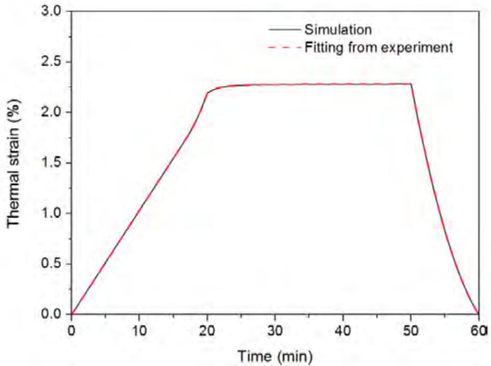
Figure 2 Thermal strain of the MAT277 single element test
