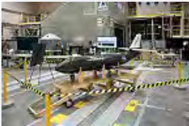
The objectives of testing on PTERA include the development of tools and vetting of system integration, evaluation of vehicle control law, and analysis of SAW airworthiness to examine benefits to in-flight efficiency. Credits: NASA
