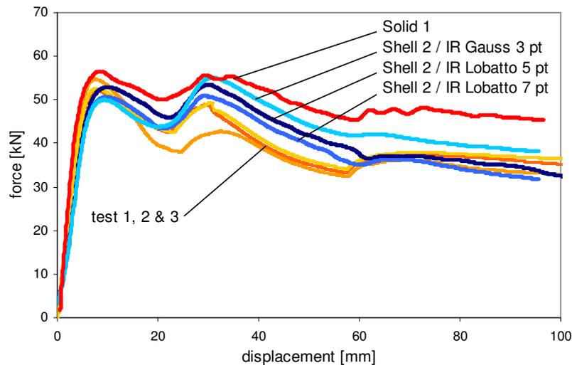
Figure 9: Comparison of the force vs. displacement curves of the experimental test results and simulations with different element formulations.
