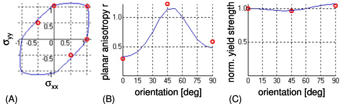
Figure 2: Yield locus (A) and direction dependence of planar anisotropy (B) and normalized uniaxial tensile yield stress (C) of the EN-AW 6082 T6 aluminum extrusion for a plastic strain of 0.05 showing the approximation with the Dell 2006 criterion in comparison with the experiments
