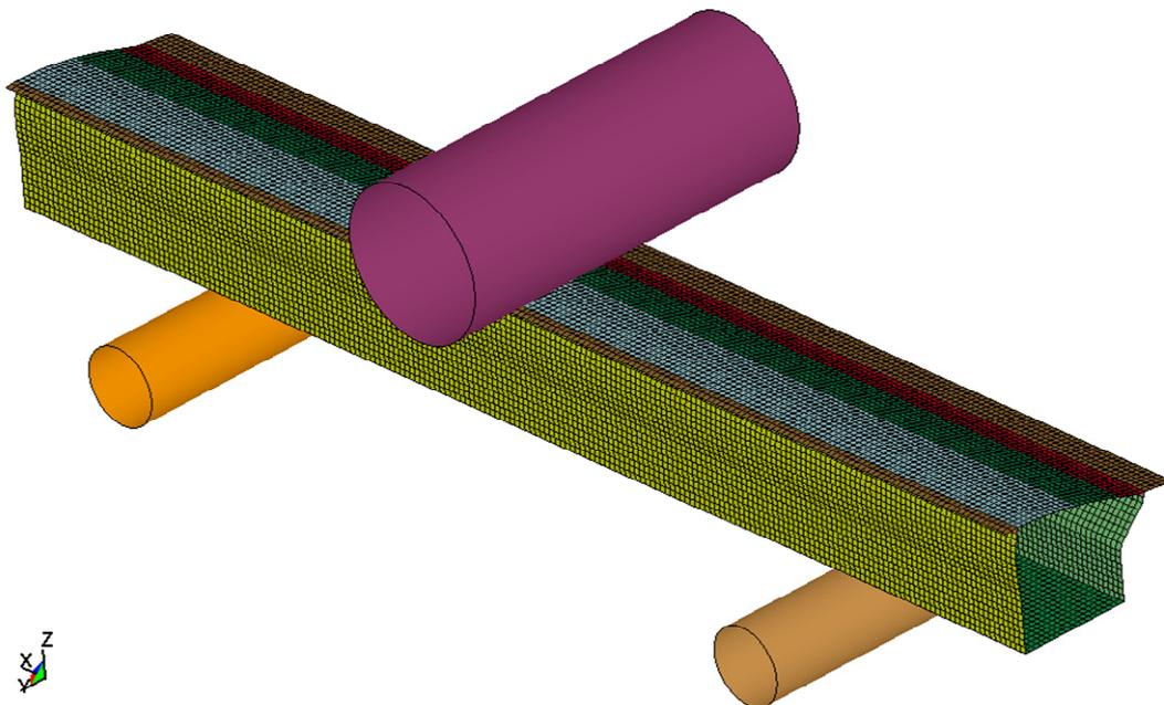
Figure 6: Finite element discretization of the 3-point bending test with shell elements
