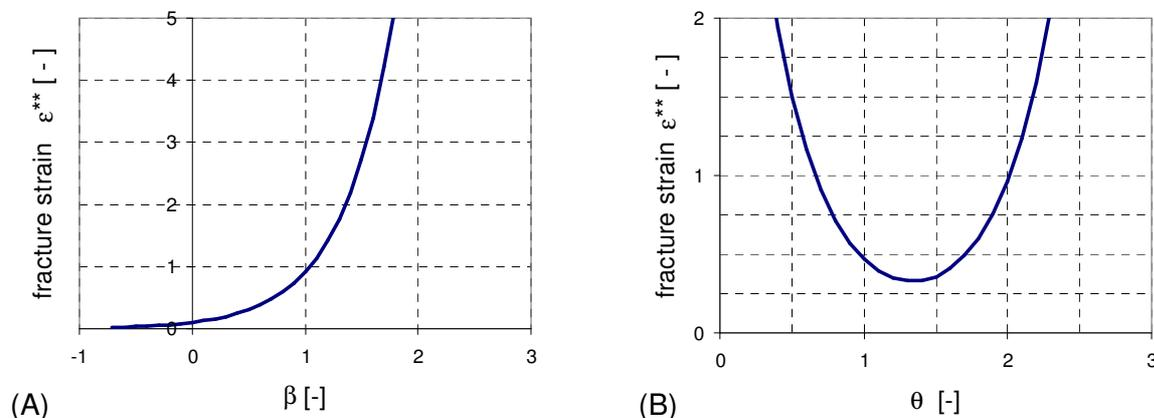
Figure 3: Quasi-static normal fracture curve  $\varepsilon^{**}(\beta)$  and shear fracture curve  $\varepsilon^{**}(\theta)$  of the EN-AW 6082 T6 extrusion profile
