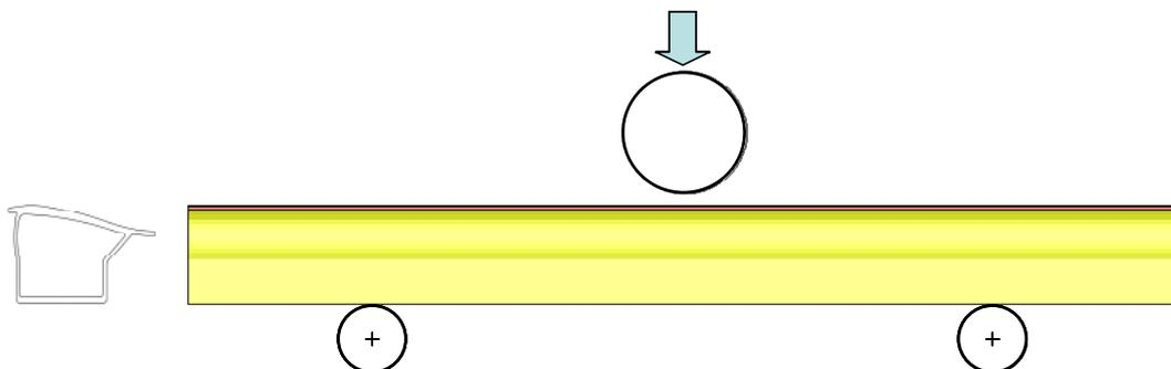
Figure 5: 3-point bending test used to validate the fracture model for the bumper profiles
