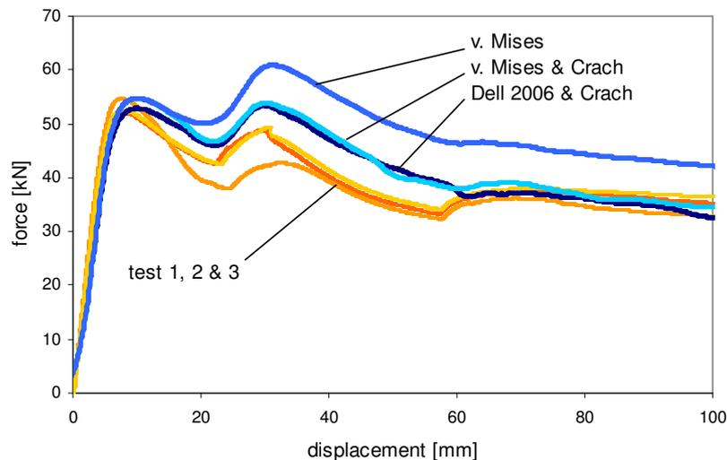
Figure 8: Comparison of the force vs. displacement curves of the experimental test results and simulations with shell elements using different material models.
