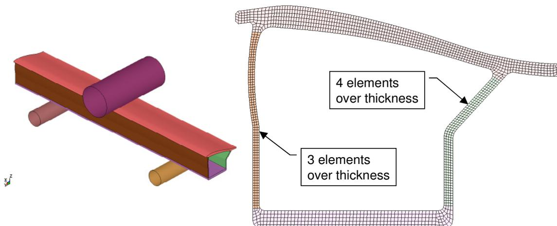
Figure 7: Finite element discretization of the 3-point bending test with solid elements
