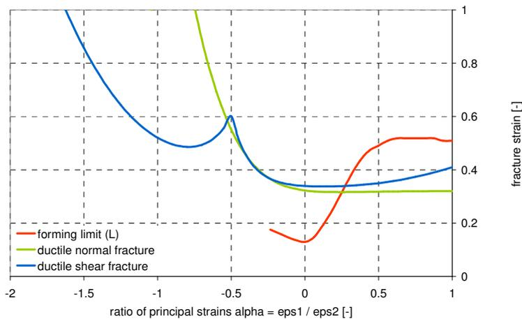
Figure 4: Ductile normal fracture, ductile shear fracture and forming limit due to membrane instability of the extrusion EN-AW 6082 T6 plotted as fracture or failure strain as a function of the ratio of principal strain rates for the special case of plane-stress conditions
