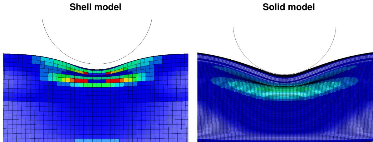
Figure 11: Comparison of the maximum failure risk distribution briefly after fracture initiation – correct prediction with shell model (left) still subcritical risk of fracture in solid model (right)
