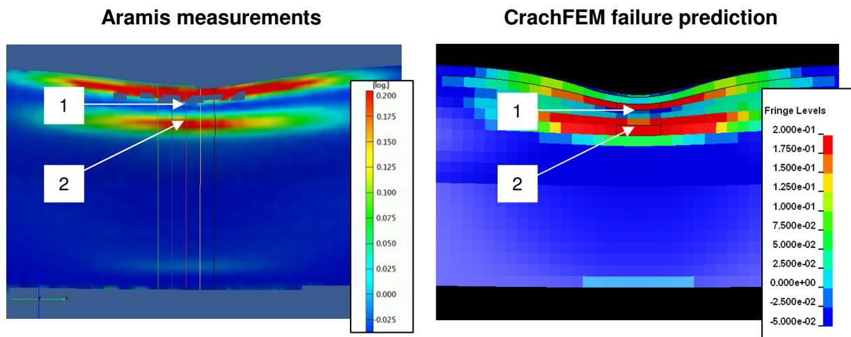
Figure 10: Maximum principal strain at the outer surface after initiation of fracture – Aramis optical strain measurements (left) and simulation with shell discretization and MF GenYld + CrachFEM (right)
