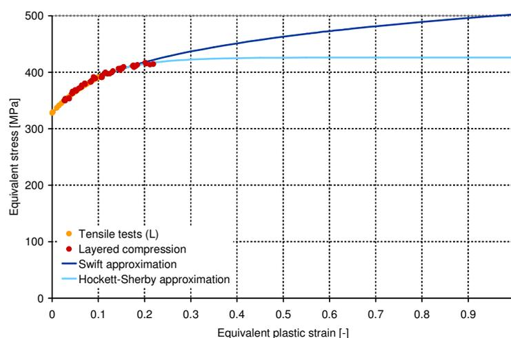
Figure 1: Hardening of the EN-AW 6082 T6 aluminum extrusion – tensile tests in extrusion direction, layered compression tests and approximations with the Swift and the Hockett-Sherby hardening laws
