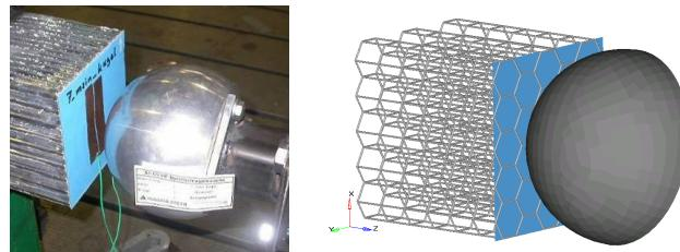
Figure 12: Initial state of sphere loaded specimen – test and FE model
