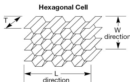
Figure 1: Principle directions of hexagonal honeycomb structure
