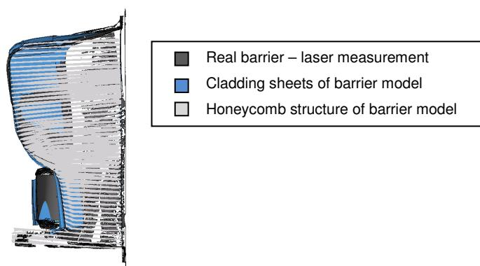
Figure 17: Overlay of deformed shape of real barrier with barrier model (vertical central cut)
