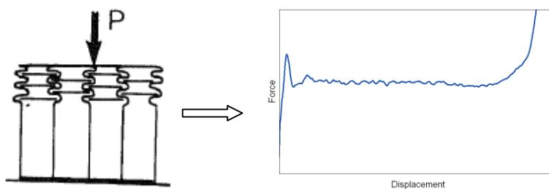
Figure 2: Buckling and force-deflection behaviour of T-directional loaded honeycomb structure [3]
