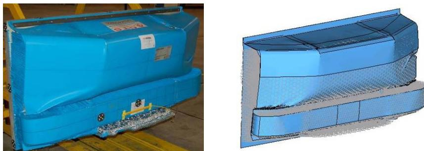
Figure 16: Comparison of deformation behaviour – test and FE model
