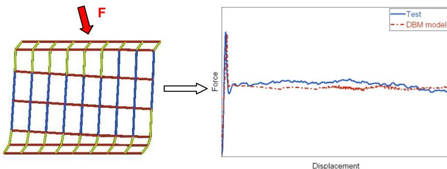
Figure 11: Deformation of TW15° loaded DBM model and validation of force-displacement curve
