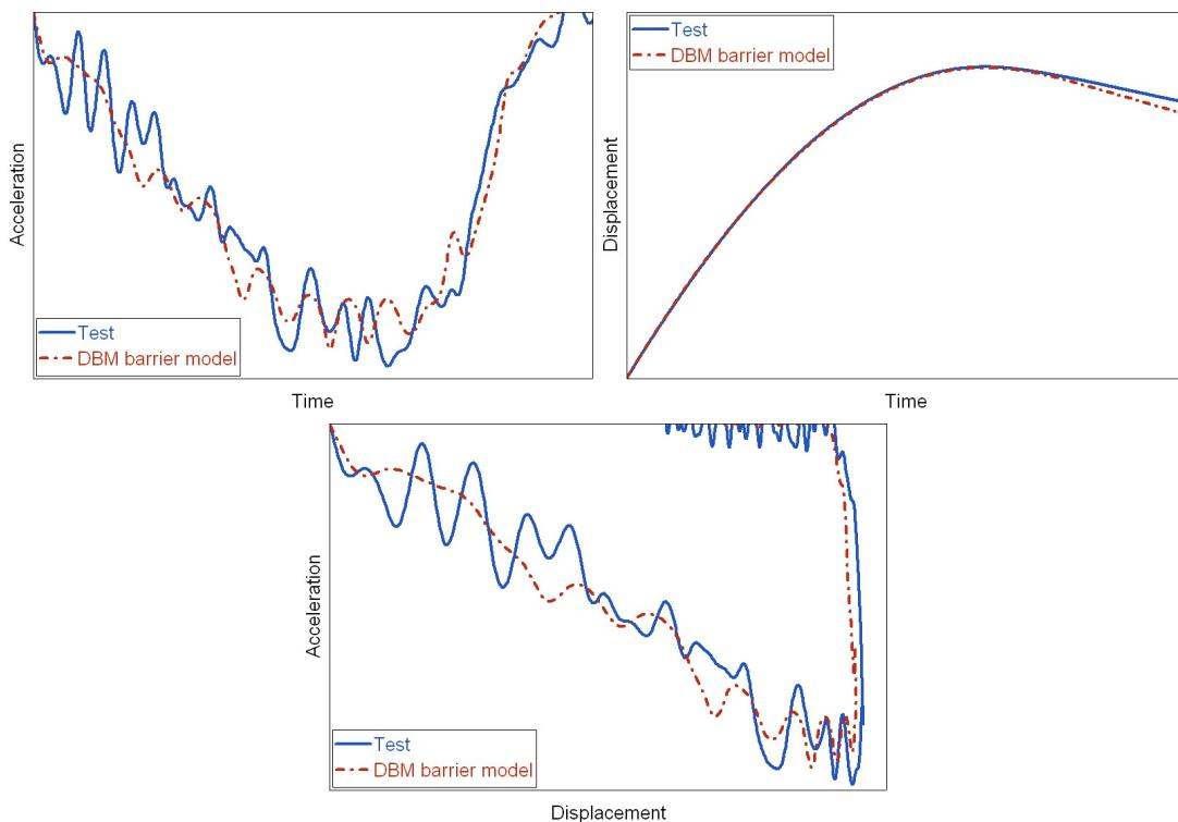
Figure 19: Validation of acceleration-time, displacement-time and acceleration-displacement curve
