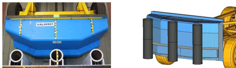
Figure 18: Initial state of load case 'three poles': test and FE model
