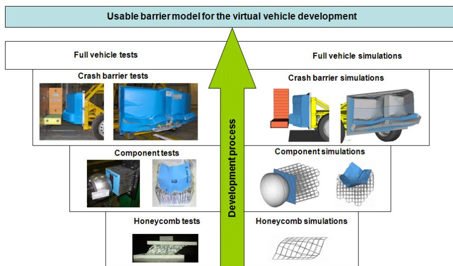
Figure 9: Development process of IIHS crash barrier model based on DBM
