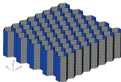
Figure 5: FE model of honeycomb structure based on shell elements
