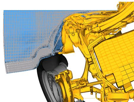
Figure 22: Vertical cut of ODB and front end
