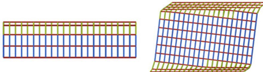
Figure 7: Characteristic deformation behaviour of T- and mixed directional loaded honeycomb model
