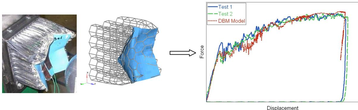
Figure 13: Validation of deformation behaviour and force-displacement curve
