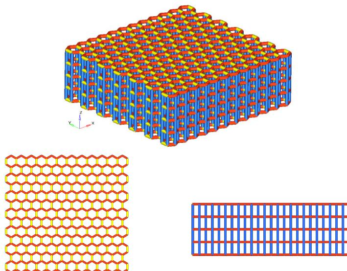
Figure 6: Iso, top and side view of honeycomb model based on DBM
