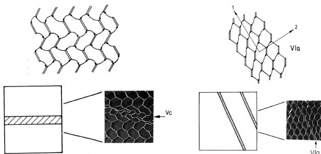
*Figure 4: Principle deformation behaviour of transversely loaded honeycomb structure [5]*
