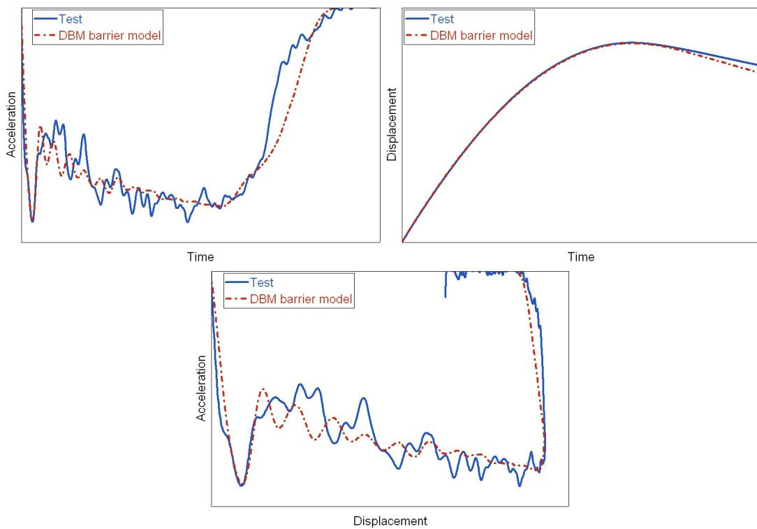
Figure 15: Validation of acceleration-time, displacement-time and acceleration-displacement curve
