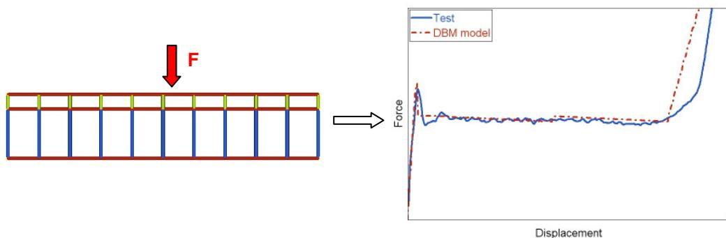
Figure 10: Deformation of T-directional loaded DBM model and validation of force-displacement curve
