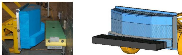
Figure 14: Initial state of load case 'rigid rocker': test and FE model
