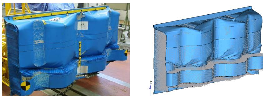
Figure 20: Comparison of deformation behaviour – test and FE model
