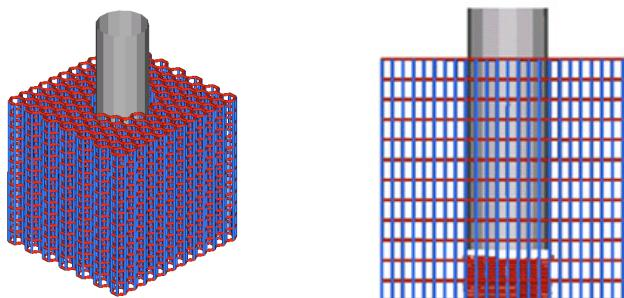
Figure 8: Characteristic deformation behaviour of T-directional locally loaded honeycomb model
