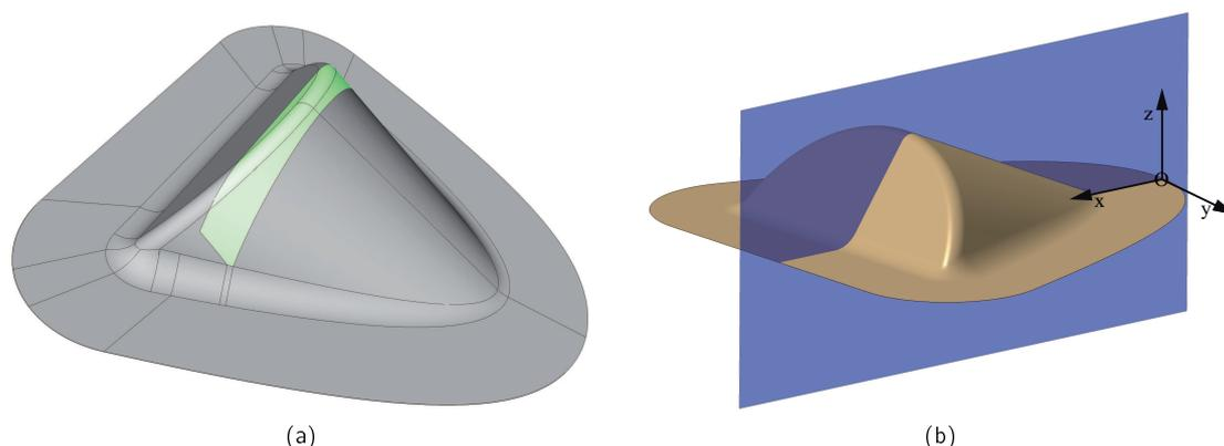
Figure 9: CAD model of the benchmark part. Green marked regions represent the supported area by the partial die for the ISF forming process (Fig. 9a)
