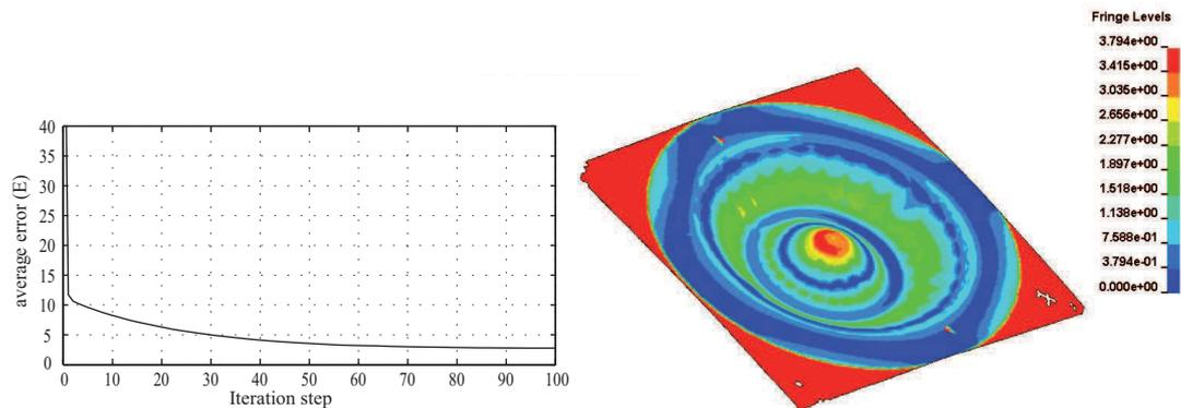
Figure 3: Average Error in relation to the „Best Fit“ iteration steps (left) and resulting overall error in [mm] of the „Best Fit“ positioning for an example part with more weights on the boundary (right)
