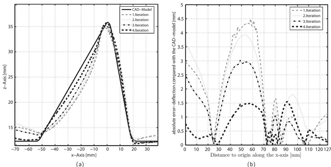
Figure 10: Cross section cut along the X-axis (Fig. 10a) and the absolute error deflection in each iteration (Fig. 10b)
