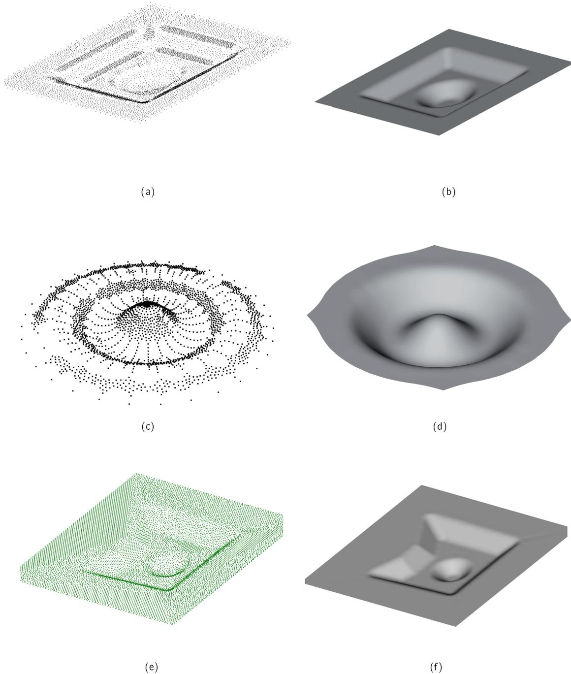
Figure 8: *Approximating B-Spline-Surface (b,d,f) and the related 3D surface mesh (a,c,e)*
