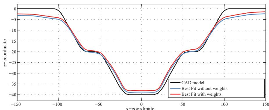
Figure 2: Cut through a CAD geometry compared to two „Best Fit“ formed geometries with and without weights on the boundary of the geometry
