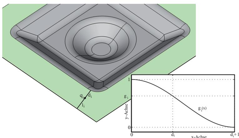
Figure 4: Weighting function which vanishes towards the boundary
