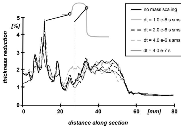
Fig. 6: Thickness reduction for different time step sizes with selective mass scaling (sms)
