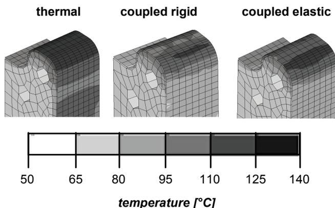
Fig. 8: Punch surface temperature after 1 s for different tool modelling approaches
