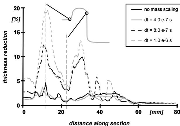
Fig. 5: Thickness reduction for different time step sizes
