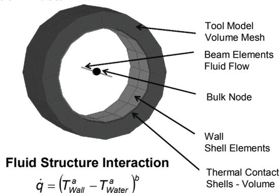
Fig. 9: Representation of cooling passages
