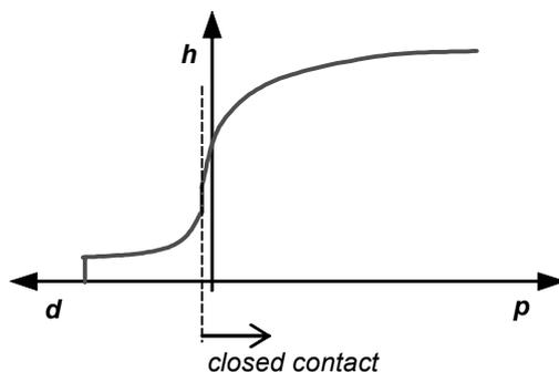
Fig. 3: Contact heat transfer coefficient  $h$  as a function of contact gap  $d$  and contact pressure  $p$
