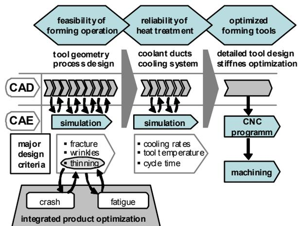
Fig. 1: Process and product optimization workflow in hotforming
