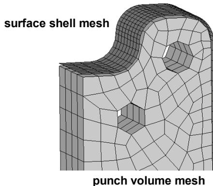
Fig. 7: Tool model with surface shell mesh
