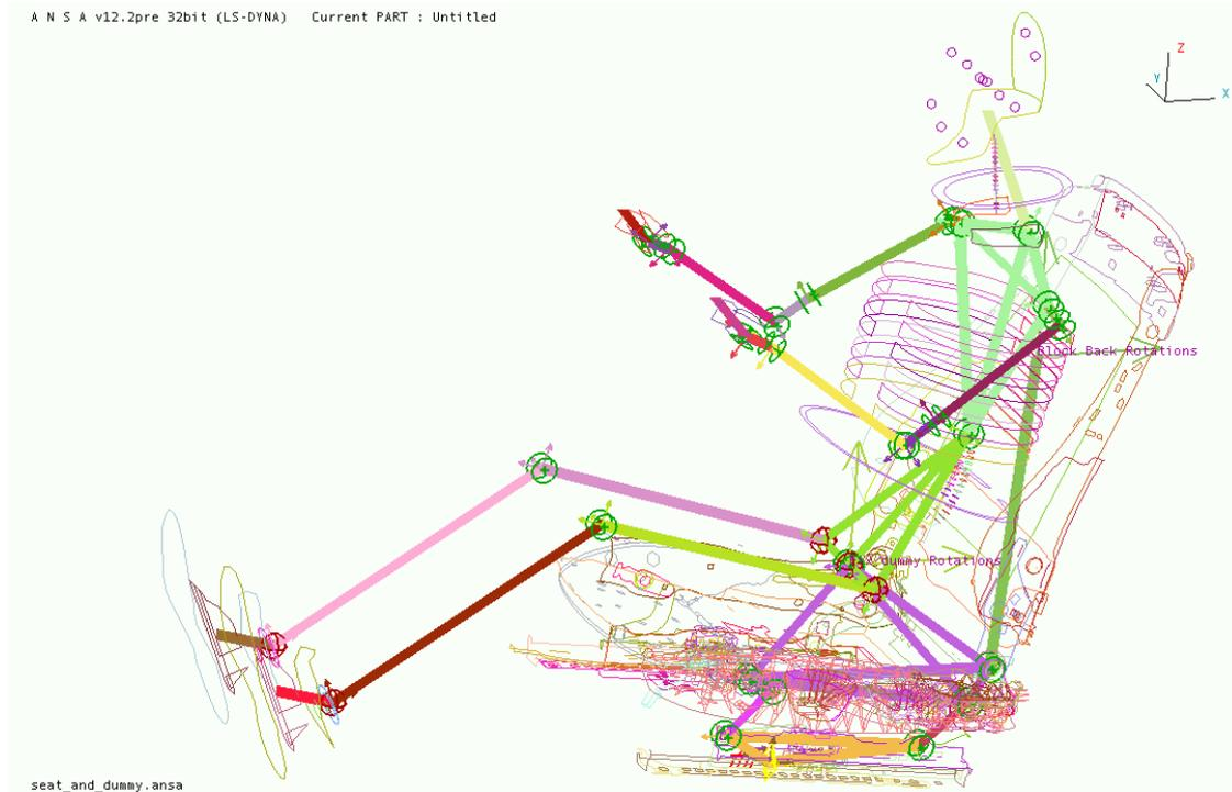
Fig. 3: A complete seat and dummy kinematic model
