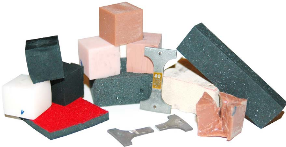
Figure 18: Material test samples of WorldSID
