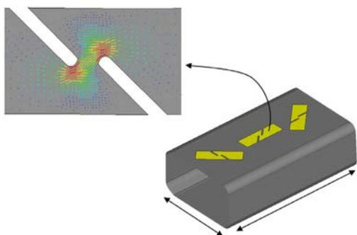
absorption under crash loadings. However, such materials exhibit a highly orthotropic behavior both in plasticity and in failure for which an orientation-dependent damage accumulation is necessary for accurate results. Polymers are a further example of materials that, under certain circumstances, require a more advanced treatment of the damage modeling than the typically applied scalar damage models.
