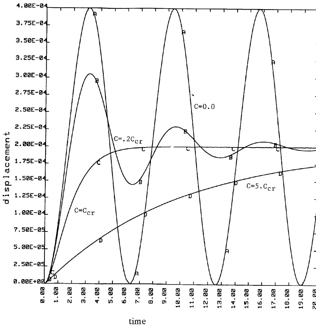
Figure 64.1 Displacement versus time curves with a variety of damping coefficients applied to a one degree-of-freedom oscillator.
