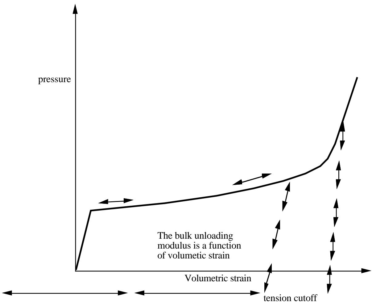
Figure 3.32. Pressure versus volumetric strain curve for equation-of-state Form 8 with compaction. In the compacted states the bulk unloading modulus depends on the peak volumetric strain.
