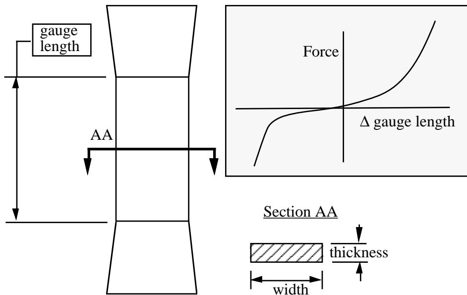
Figure 3.12. Uniaxial specimen for experimental data.
