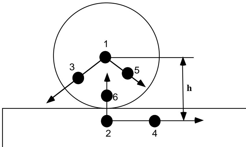
Figure 39.5 Rack and pinion joint. Nodal pair (1,3) defines an axes that is orthogonal to the gear. Nodal pair (1,5) is a vector in the plane of the gear. The value  $h$  is specified.
