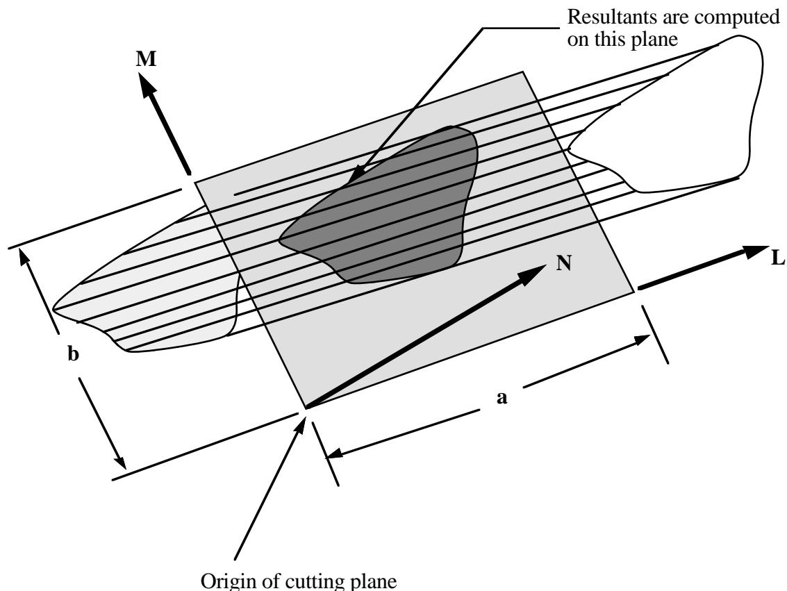
Figure 22.1. Definition of cutting plane for automatic definition of interface for cross-sectional forces. The automatic definition does not check for springs and dampers in the section. For best results the cutting plane should cleanly pass through the middle of the elements, distributing them equally on either side.
