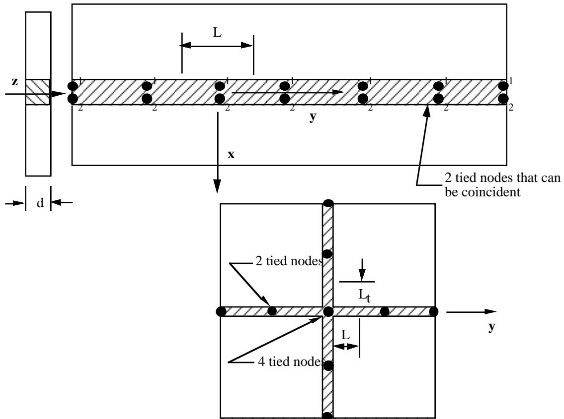
Figure 37.3. Orientation of the local coordinate system and nodal ordering is shown for butt weld failure.
