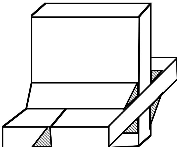
Figure 37.5. A general weld is a mixture of fillet and butt welds.
