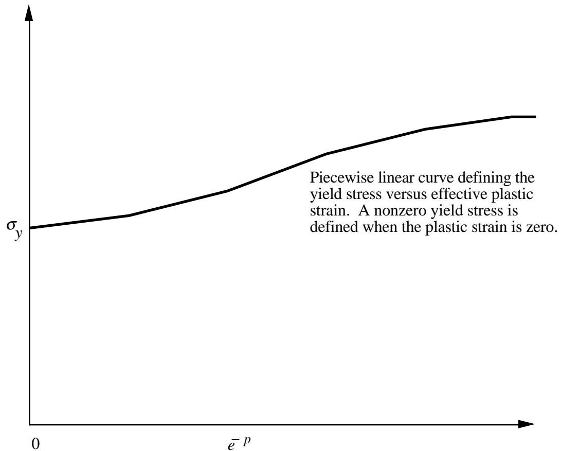
Figure 3.8. Effective stress versus effective plastic strain curve.
