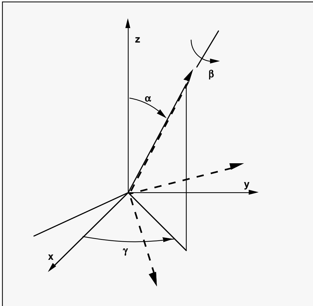
Figure 39.11 Flexion-torsion joint angles.
