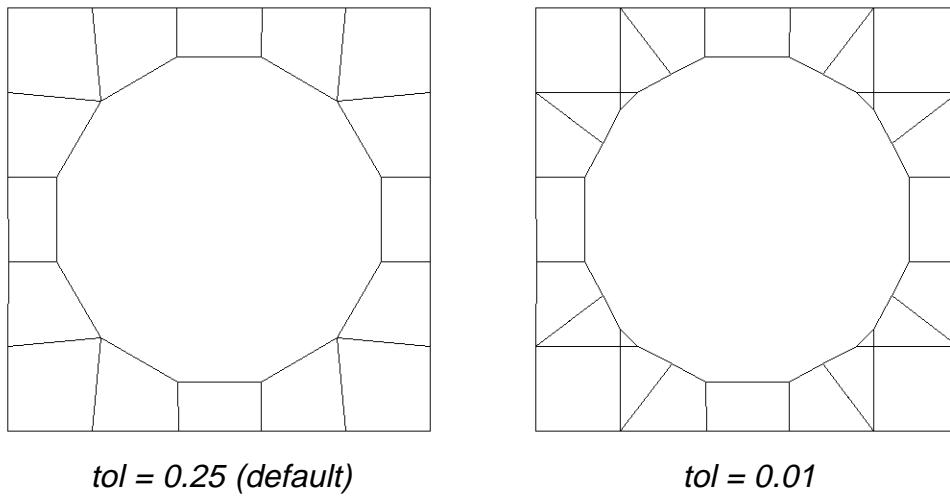
**Figure 69.2 - Trimming Tolerance.** The tolerance limits the size of the small elements generated during trimming. The default tolerance (left) produces large elements. Using a tolerance of 0.01 (right) allows smaller elements, and more detail in the trim line.
