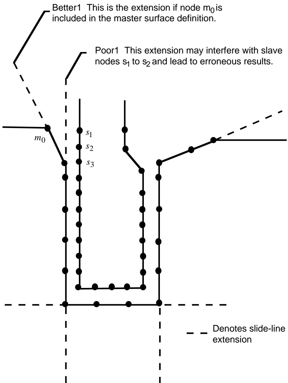
Figure 57.2. Master surface extensions defined automatically by DYNA (extensions are updated every time step to remain tangent to ends of master sides of slidelines unless angle of extension is defined in input).
