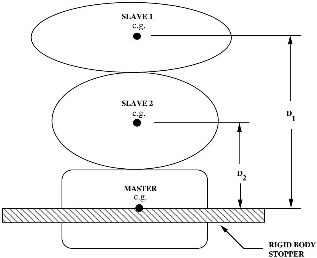
Figure 60.1. When the master rigid body reaches the rigid body stopper, the velocity component into the stopper is set to zero. Slave rigid bodies 1 and 2 also stop if the distance between their mass centers and the master rigid body is less than or equal to the input values  $D_1$  and  $D_2$ , respectively.
