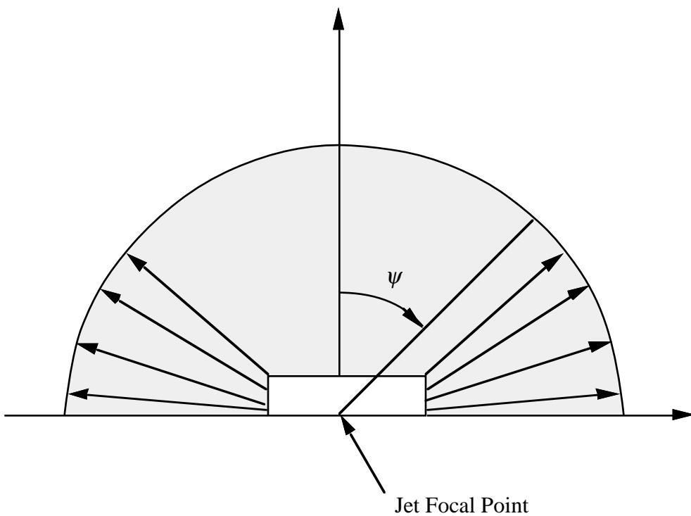
Figure 58.2. Multiple jet model for the drivers side airbag.
