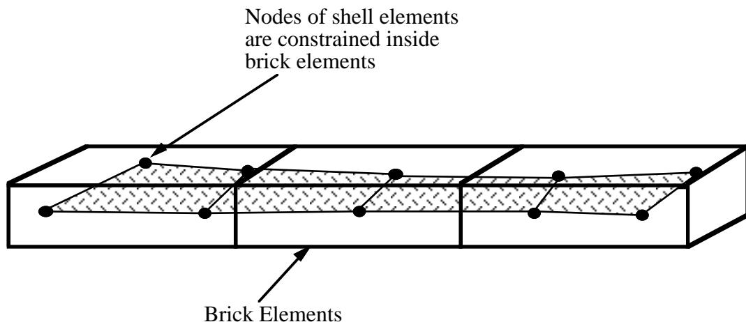
Figure 75.1. Nodes of Lagrange elements are constrained to move with the material points of the solid elements. The slave elements may be either Lagrangian shells, beams or bricks.
