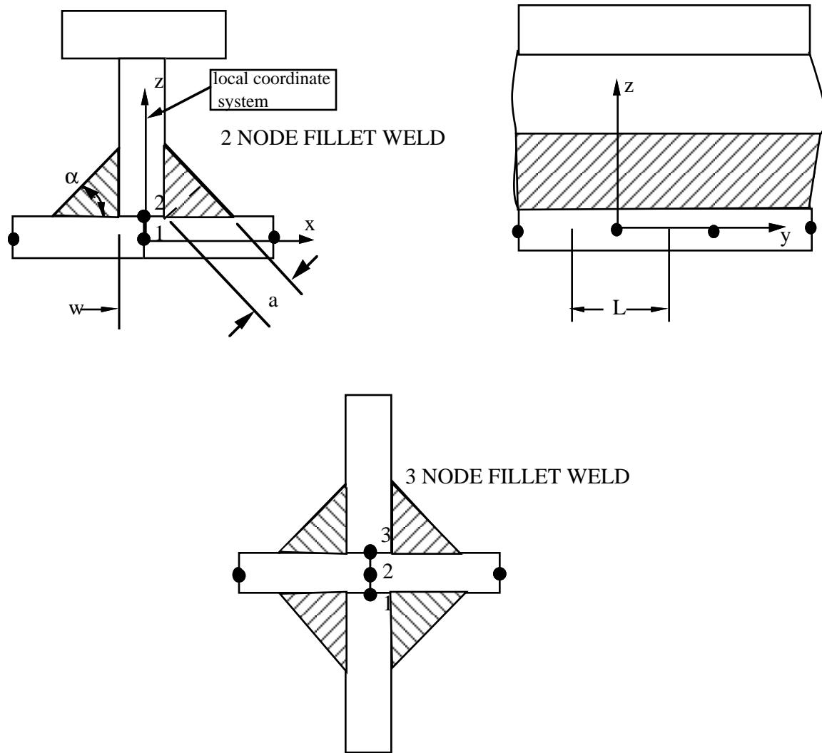
Figure 37.2. Nodal ordering and orientation of the local coordinate system is shown for fillet weld failure.
