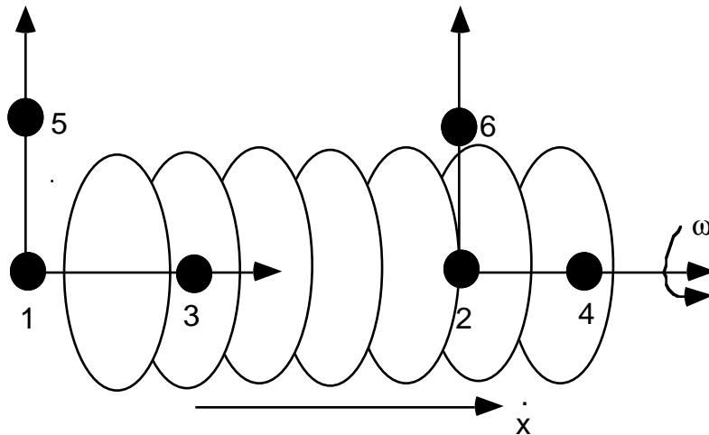
Figure 39.8. Screw joint. Nodal pairs (1,3) and (2,4) lie along the same axis and nodal pairs (1,5) and (2,6) are orthogonal vectors. The helix ratio,  $\frac{\dot{x}}{\omega}$ , is specified.
