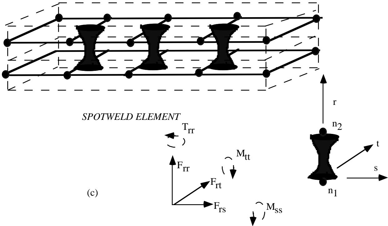
Figure 3.2. LS-DYNA beam elements: (a) 2-noded beam element, (b) discrete beam element, and (c) spot weld element. The beam spot weld elements must originate at the shell mid-surface for automatic tying with type 7 constraint contact. If the spot weld cross section is circular the orientation node is optional though necessary if the s and t directions are important. Attachments of the spot weld elements to rigid body nodes are permitted but not with type 7 constraint contact.
