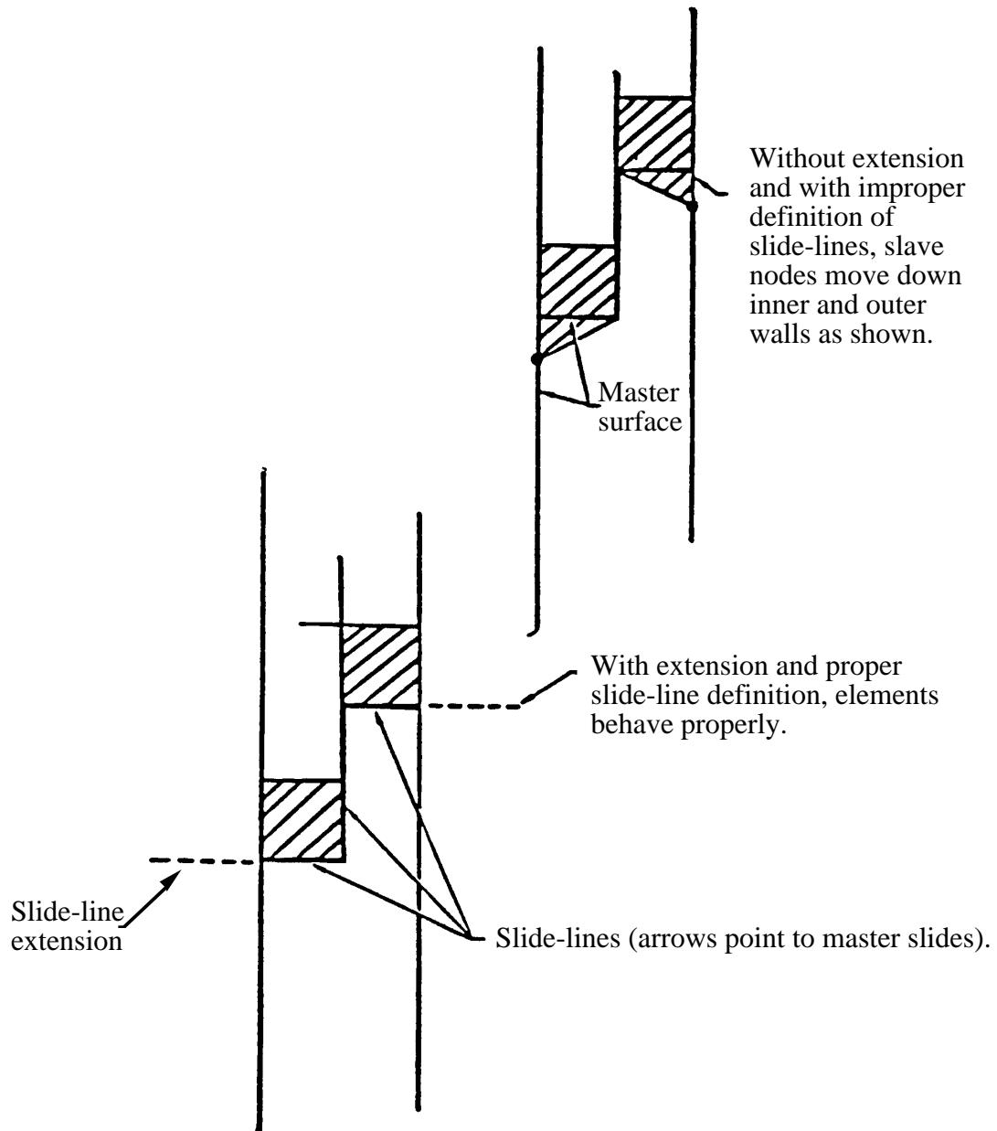
Figure 57.3. Example of slideline extensions helping to provide realistic response.
