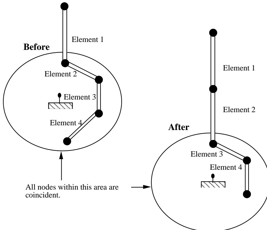
Figure 52.2. Elements in a retractor.
