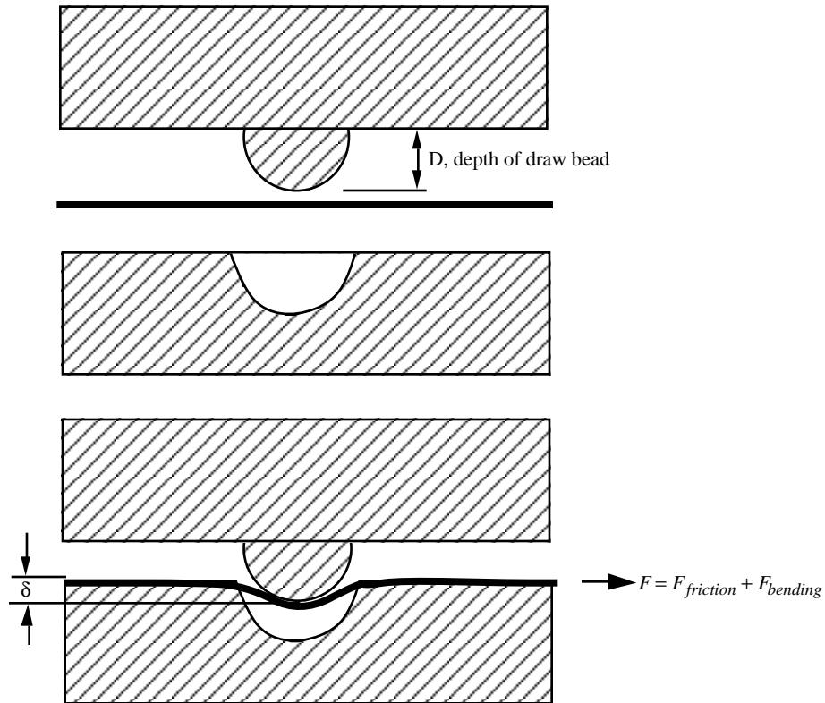
Figure 32.1. Draw bead contact model defines a resisting force as a function of draw bead displacement.
