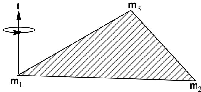
Figure 24.1. Follower force and moment acting on a plane defined by nodes  $m_1$ ,  $m_2$ , and  $m_3$ . In this case, the load is applied to node  $m_1$ ; i.e.,  $m=m_1$ . A positive force acts in the positive  $t$  direction, and a positive moment puts a counterclockwise torque about the normal vector.
