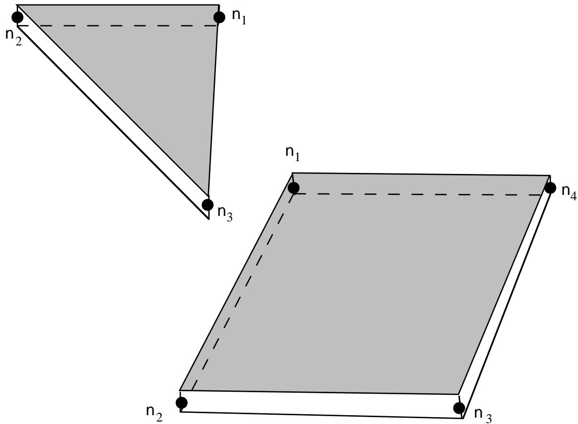
Figure 3.4. LS-DYNA shell elements. Counterclockwise node numbering determines the top surface.
