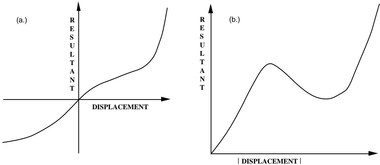
Figure 3.19. The resultant forces and moments are determined by a table lookup. If the origin of the load curve is at [0,0] as in (b.) and tension and compression responses are symmetric.
