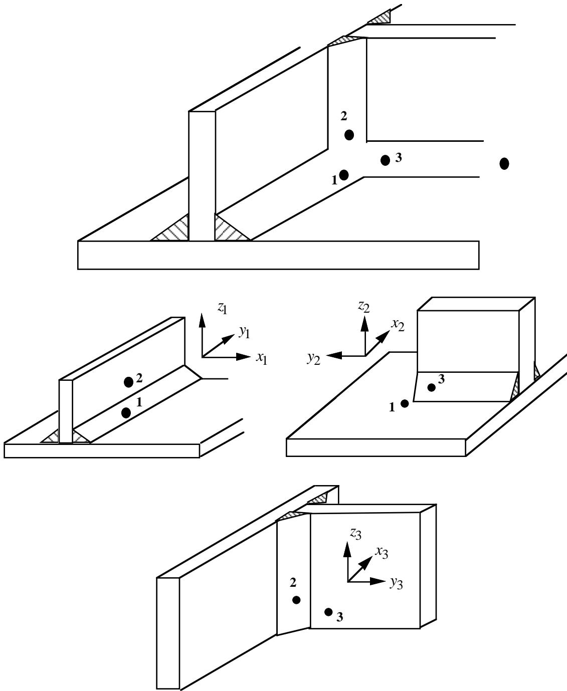
Figure 37.4. A simple cross fillet weld illustrates the required input. Here NFW=3 with nodal pairs ( $A=2, B=1$ ), ( $A=3, B=1$ ), and ( $A=3, B=2$ ). The local coordinate axes are shown. These axes are fixed in the rigid body and are referenced to the local rigid body coordinate system which tracks the rigid body rotation.
