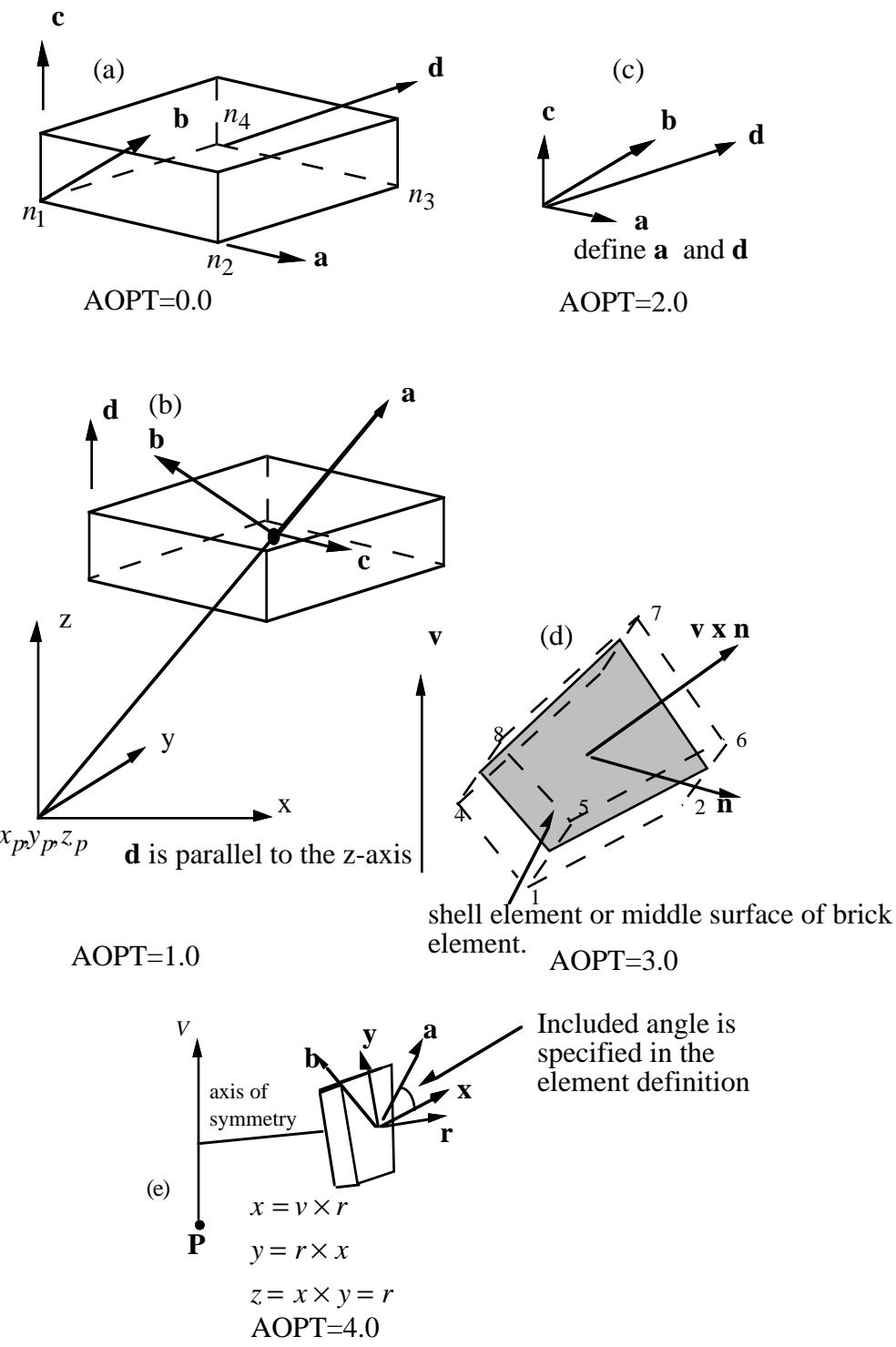
Figure 3.5. Options for determining principal material axes: (a) AOPT = 0.0, (b) AOPT = 1.0, (c) AOPT = 2.0. Note that  $\underline{c} = \underline{a} \times \underline{d}$  and that  $\underline{b} = \underline{c} \times \underline{a}$ , (d) AOPT = 3.0, and (e) AOPT=4.0 for brick elements.
