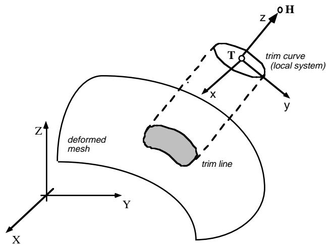
**Figure 69.1 - Trimming Orientation Vector.** The tail (**T**) and head (**H**) points define a local coordinate system (x,y,z). The local x-direction is constructed in the Xz-plane. Trim curve data is input in the x-y plane, and projected in the z-direction onto the deformed mesh to obtain the trim line.
