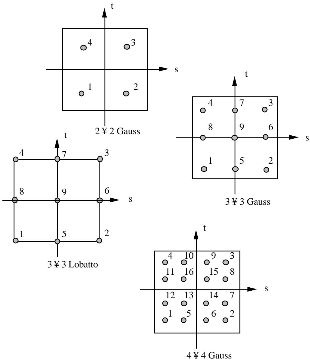
Figure 3.1. Location of the integration points in the Hughes-Liu beam element.
