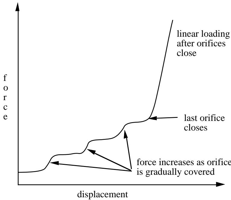
Figure 3.22. Force versus displacement as orifices are covered at a constant relative velocity. Only the linear velocity term is active.
