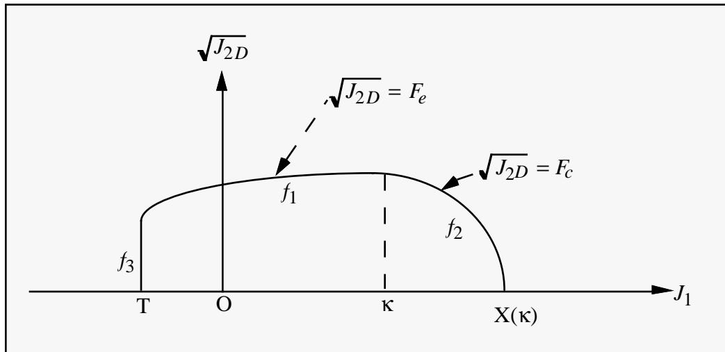
Figure 3.10. The yield surface of the two-invariant cap model in pressure  $\sqrt{J_{2D}} - J_1$  space. Surface  $f_1$  is the failure envelope,  $f_2$  is the cap surface, and  $f_3$  is the tension cutoff.
