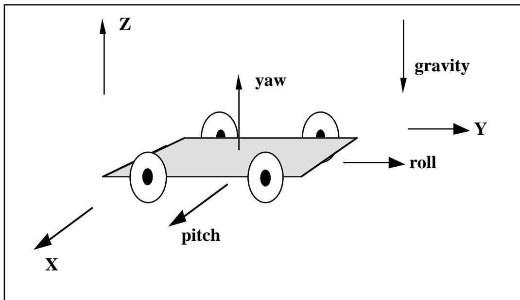
Figure 15.1. The vehicle pictured is to be oriented with a successive rotation sequence about the yaw, pitch, and roll axes, respectively. Accordingly, AAXIS=3, BAXIS=1 and CAXIS=2. The direction of gravity is given by IGRAV=-3.
