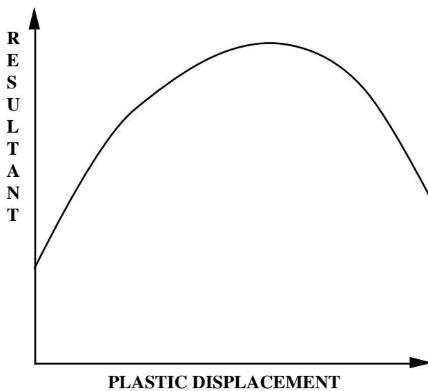
Figure 3.20. The resultant forces and moments are limited by the yield definition. The initial yield point corresponds to a plastic displacement of zero.
