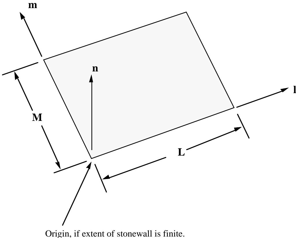
Figure 28.1. Vector **n** is normal to the stonewall. An optional vector **I** can be defined such that  $\mathbf{m} = \mathbf{n} \times \mathbf{I}$ . The extent of the stonewall is limited by defining **L** and **M**. A zero value for either of these lengths indicates that the stonewall is infinite in that direction.
