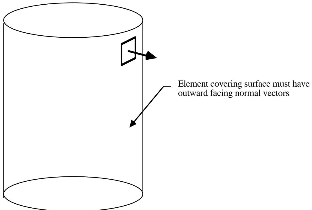
Figure 87.1. The shell elements interacting with the fluid must be numbered such that their outward normal vector points into the fluid media.
