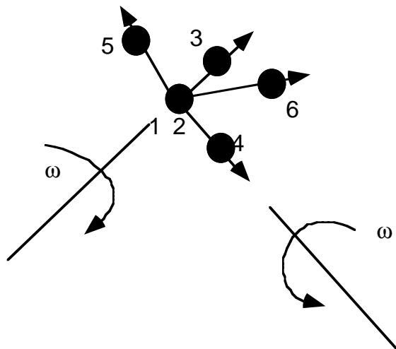
Figure 39.6 Constant velocity joint. Nodal pairs (1,3) and (2,4) define an axes for the constant angular velocity, and nodal pairs (1,5) are orthogonal vectors. Here nodal points 1 and 2 must be coincident.
