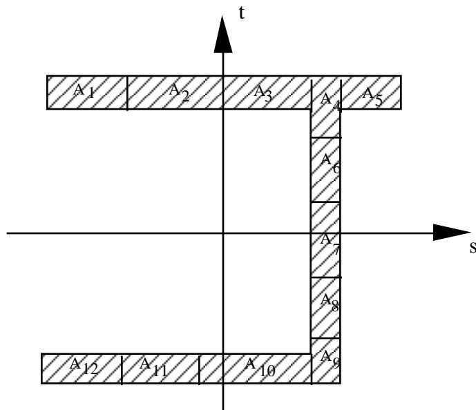
Figure 4.2. Definition of integration points for user defined integration rule.
