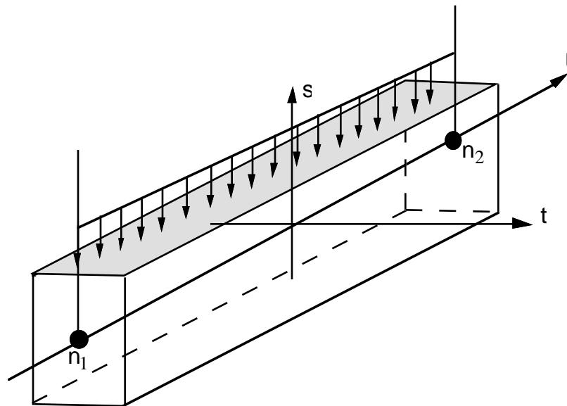
Figure 26.1. Applied traction loads are given in force per unit length.
