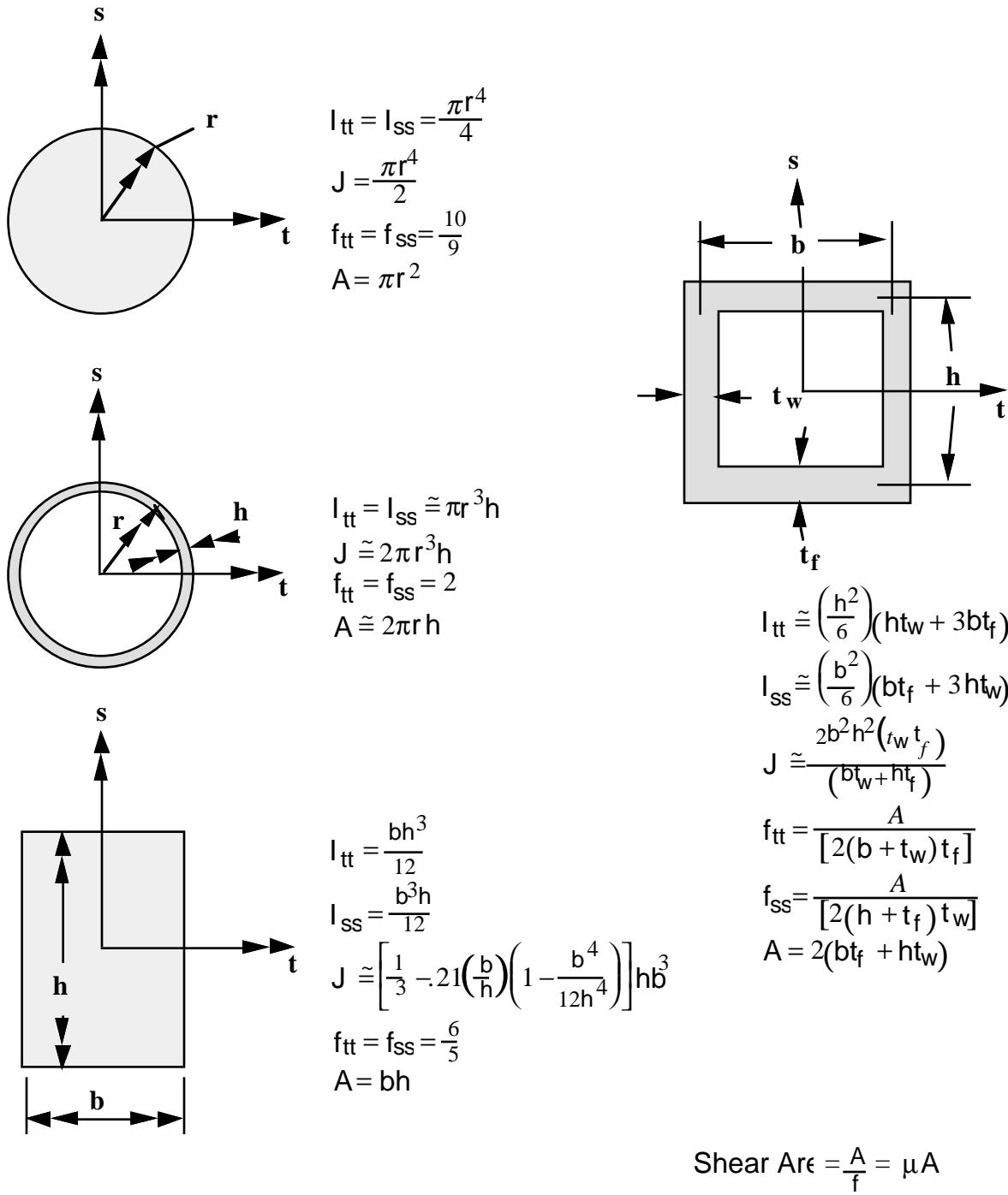
Figure 3.3. Properties of beam cross section for several common cross sections.
