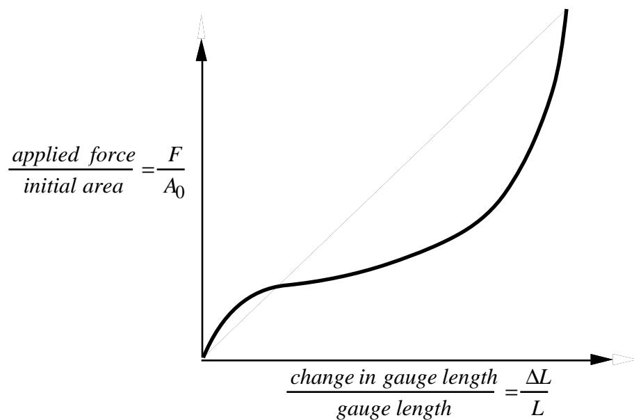
Figure 3.13. The stress versus strain curve can be used instead of the force versus the change in the gauge length by setting the gauge length, thickness, and width to unity (1.0) and defining the engineering strain in place of the change in gauge length and the nominal (engineering) stress in place of the force.
