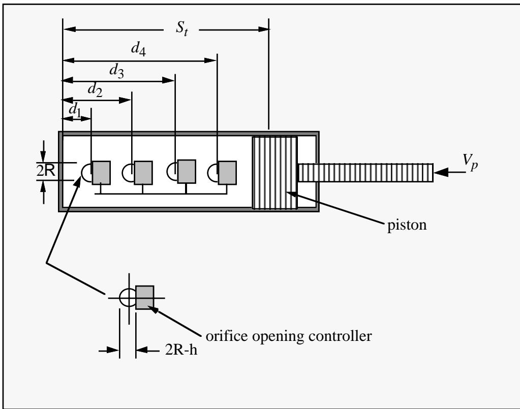
Figure 3.21. Mathematical model for the Side Impact Dummy damper.
