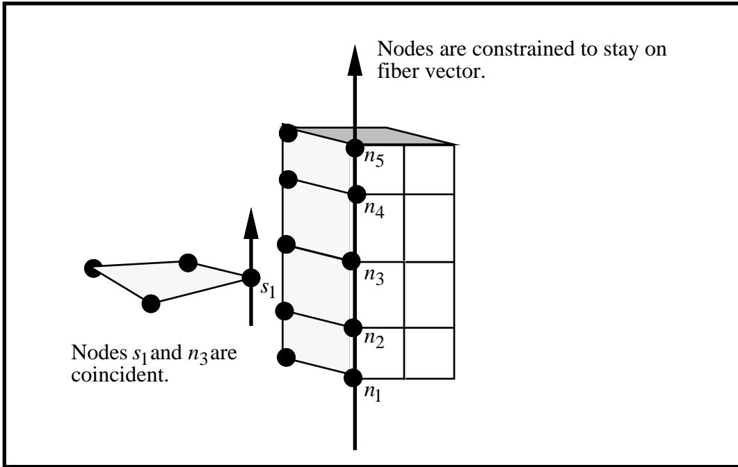
Figure 50.1. The interface between shell elements and solids ties shell node  $s_1$  to a line of nodes on the solid elements  $n_1-n_5$ . It is very important for the nodes to be aligned.
