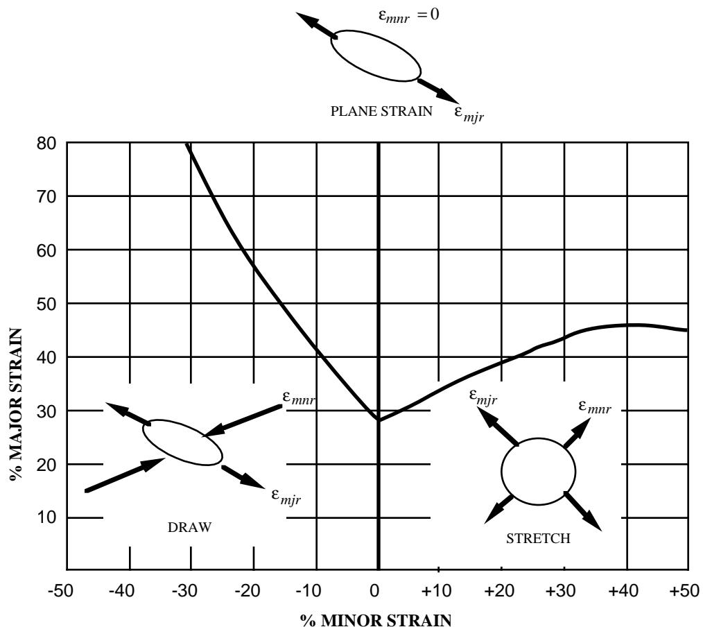
Figure 3.15. Flow limit diagram.
