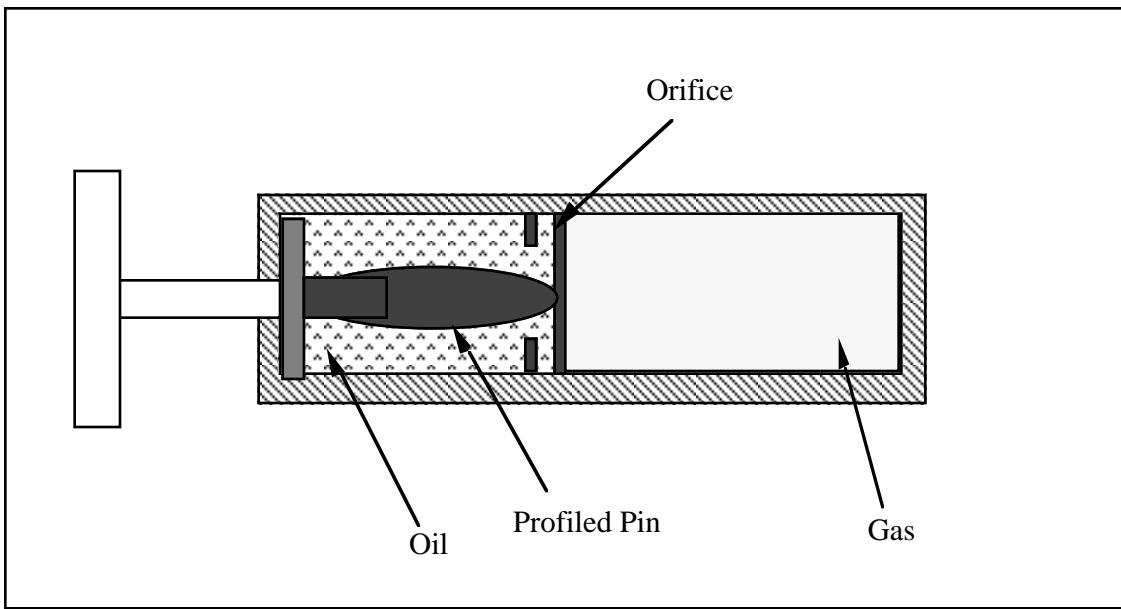
Figure 3.23. Schematic of Hydraulic/Gas damper.
