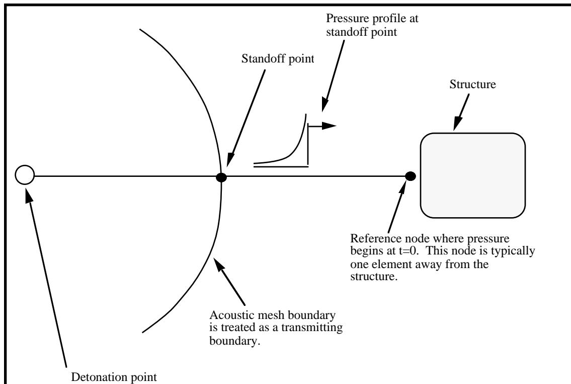
Figure 49.1 Initialization of the initial pressures due to an explosive disturbance is performed in the acoustic media. LS-DYNA automatically determines the acoustic mesh boundary and applies the pressure time history to the boundary. This option is only applicable to the acoustic element formulation.
