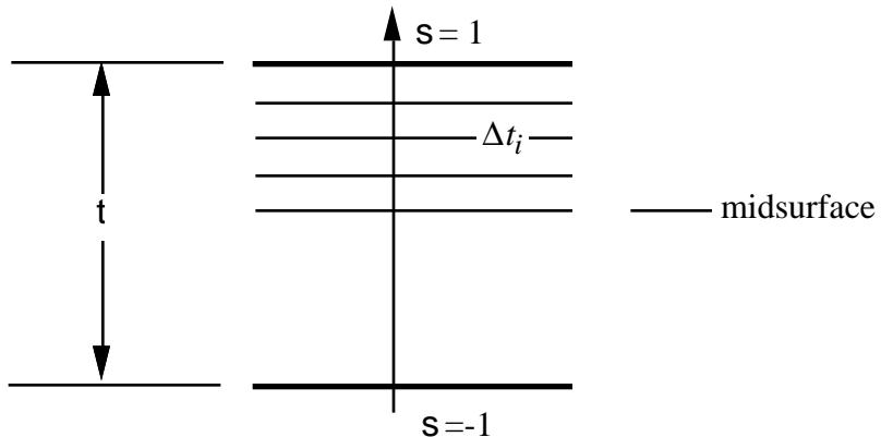
Figure 5.1. In the user defined shell integration rule the ordering of the integration points is arbitrary.
