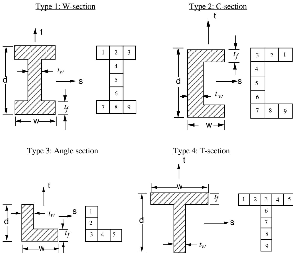
Figure 4.3a. Standard beam cross sections.
