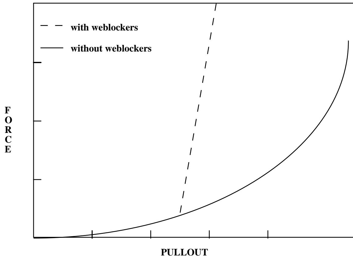
Figure 52.3 Retractor force pull characteristics.
