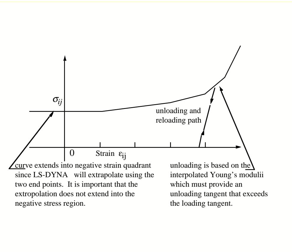
Figure 3.31. Stress quantity versus strain. Note that the “yield stress” at a strain of zero is nonzero. In the load curve definition the “time” value is the directional strain and the “function” value is the yield stress.
