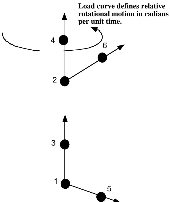
Figure 39.3. Rotational motor joint. This joint can be used in combination with other joints such as the revolute or cylindrical.
