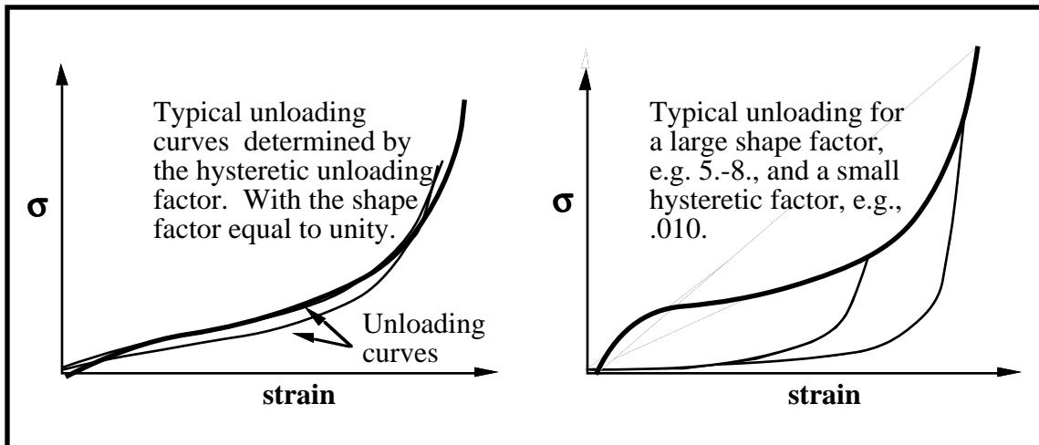
Figure 3.16. Behavior of the low density urethane foam model.
