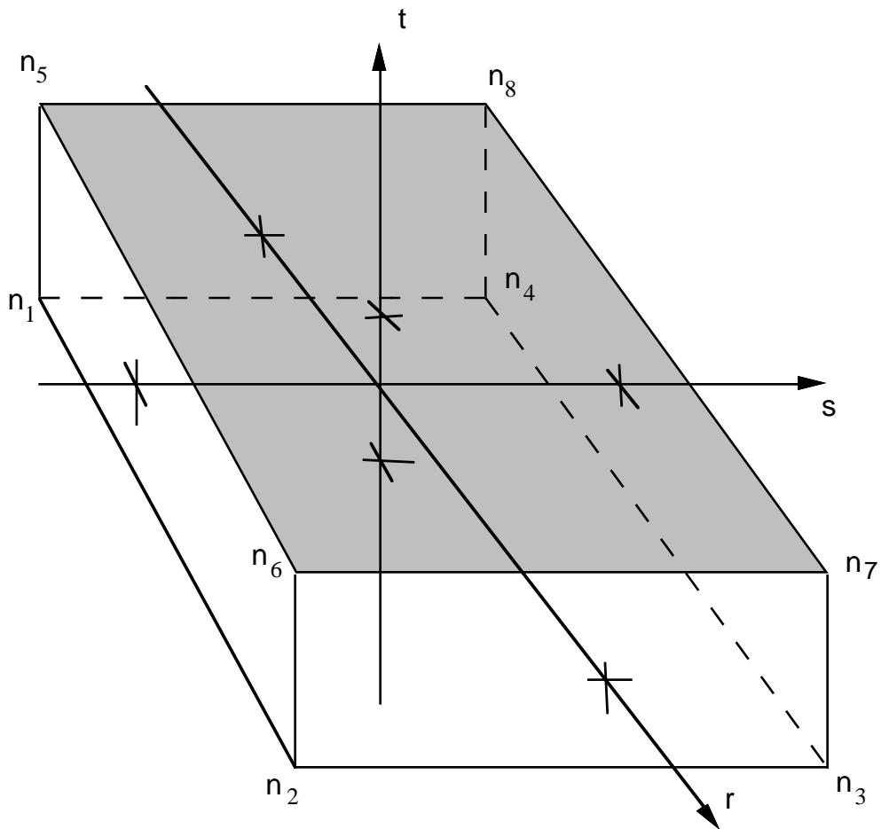
Figure 10.1. Solid 8-node Shell Element.
