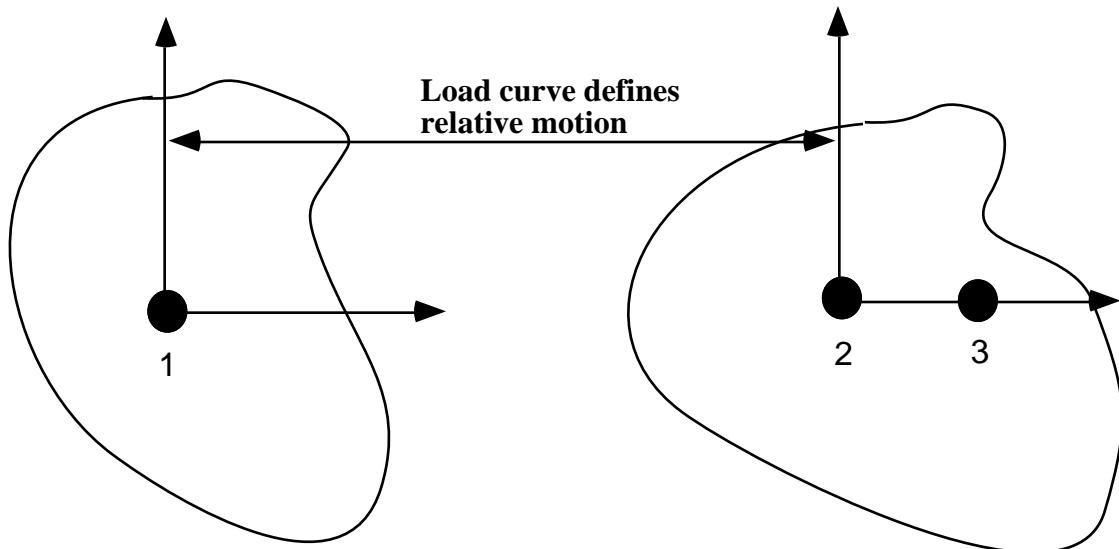
Figure 39.2. Translational motor joint. This joint can be used in combination with the translational or the cylindrical joint.
