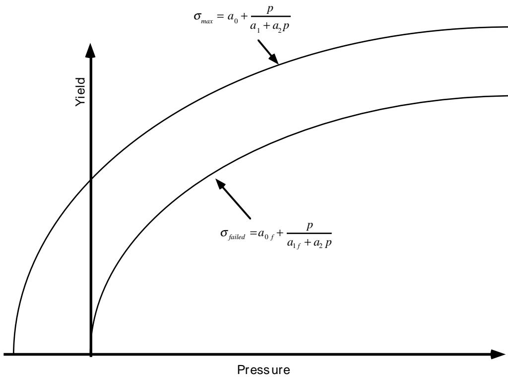
Figure 3.10. Two-curve concrete model with damage and failure.
