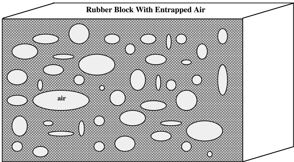
Figure 3.30. Cellular rubber with entrapped air. By setting the initial air pressure to zero, an open cell, cellular rubber can be simulated.
