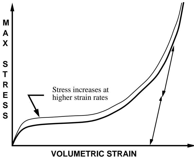
Figure 3.18. Behavior of strainrate sensitive crushable foam. Unloading is elastic to the tension cutoff. Subsequent reloading follows the unloading curve.
