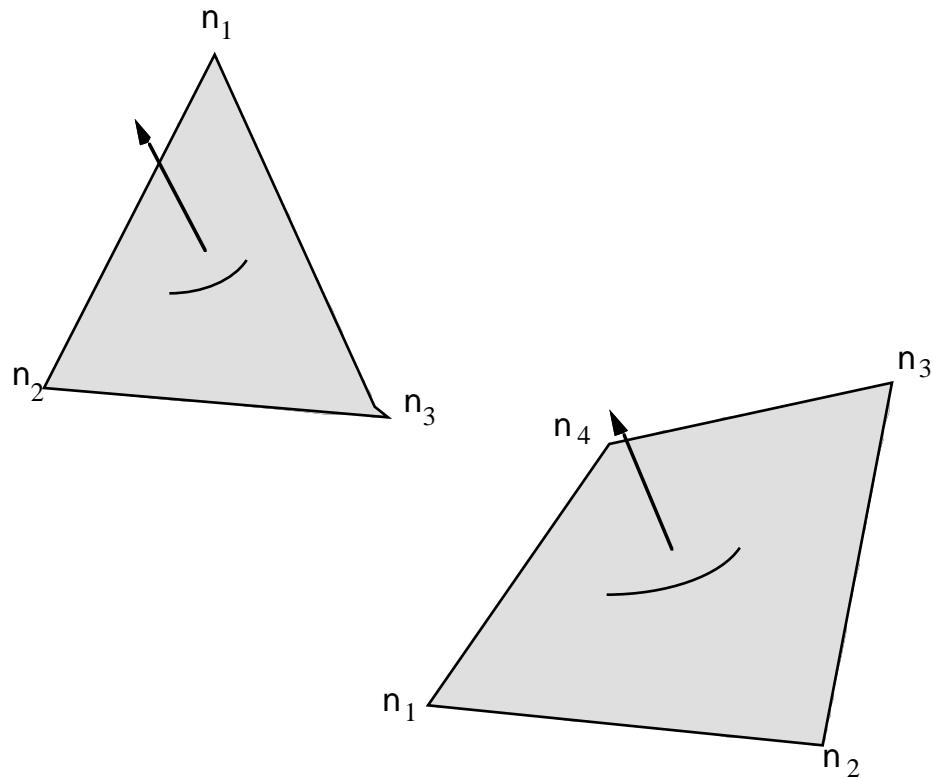
Figure 32.2. Numbering of slave and master segments. The ordering of the numbers determines the outward normal.
