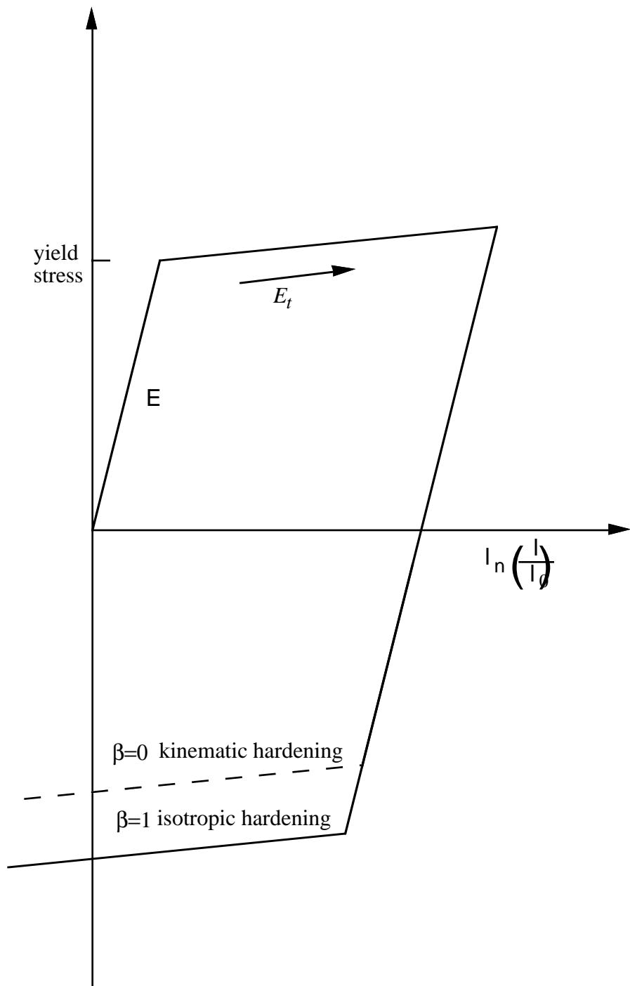
Figure 3.6. Elastic-plastic behavior with kinematic and isotropic hardening where  $l_0$  and  $l$  are undeformed and deformed lengths of uniaxial tension specimen.
