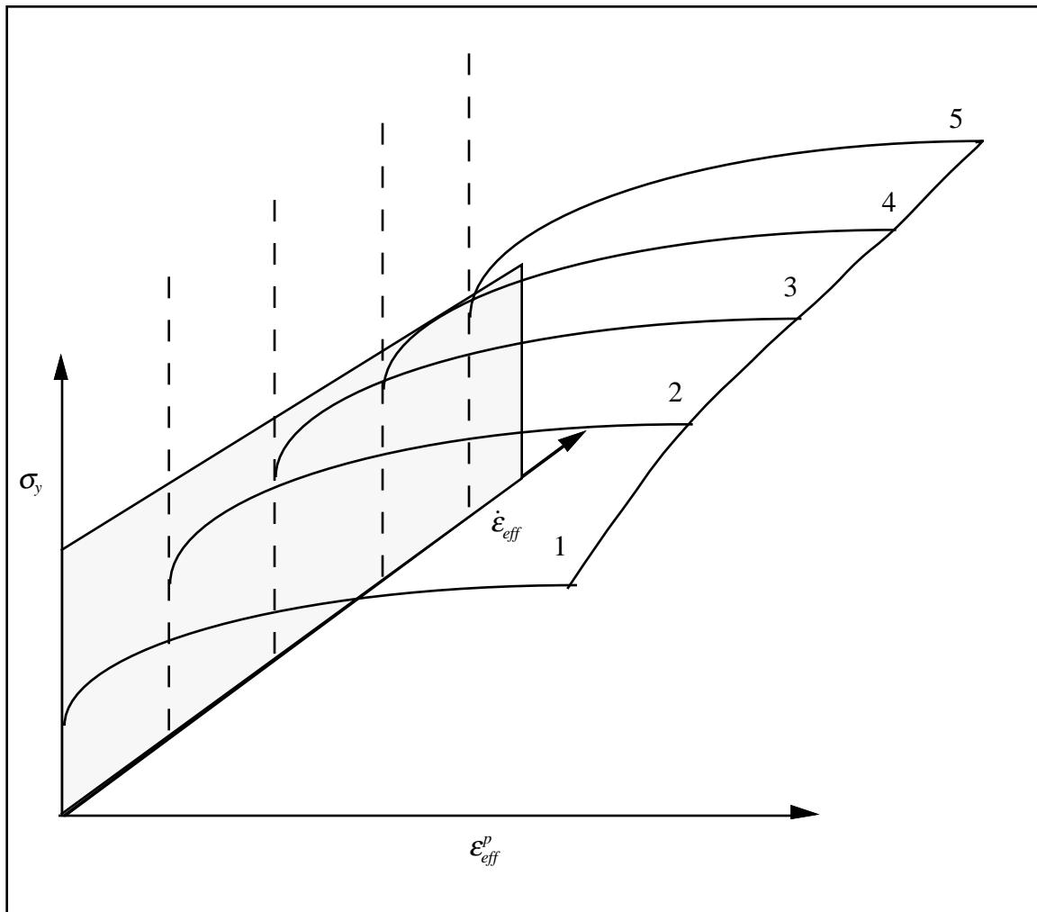
Figure 3.9. Rate effects may be accounted for by defining a table of curves. If a table ID is specified a curve ID is given for each strain rate, see Section 22. Intermediate values are found by interpolating between curves. Effective plastic strain versus yield stress is expected.
