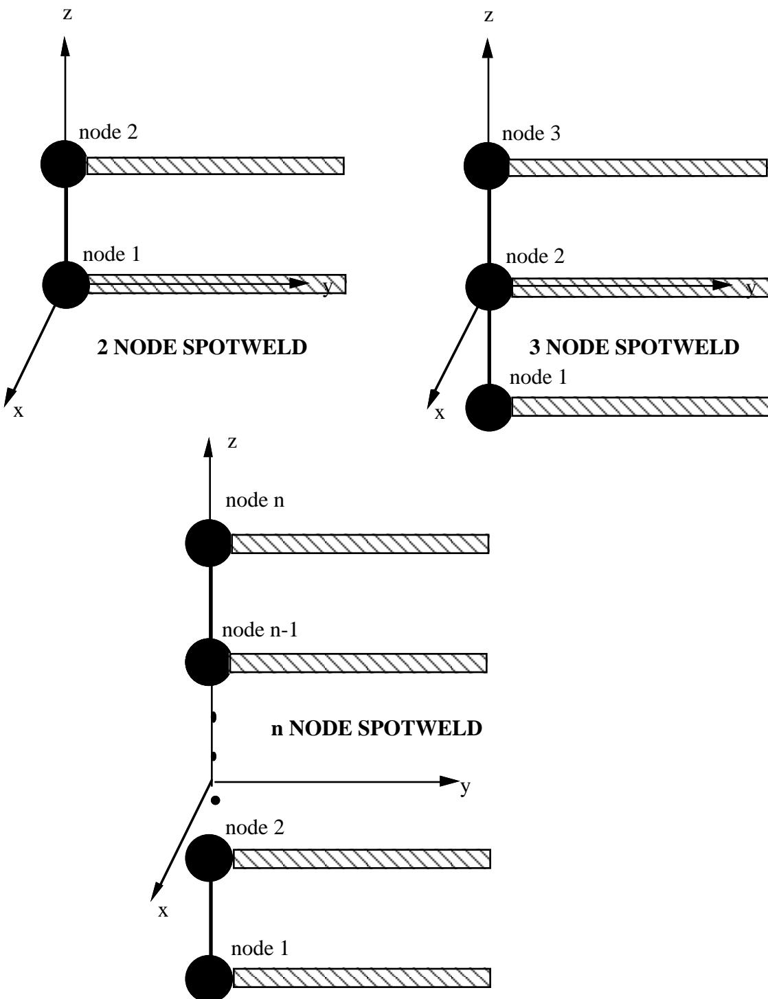
Figure 37.1. Nodal ordering and orientation of the local coordinate system is important for determining spotweld failure.
