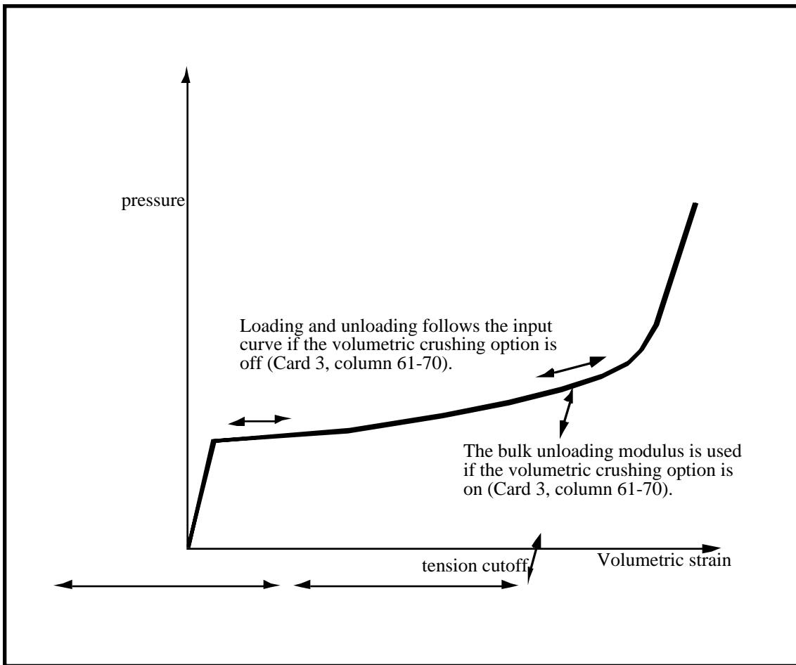
Figure 3.7. Pressure versus volumetric strain curve for soil and crushable foam model. The volumetric strain is given by the natural logarithm of the relative volume,  $V$ .
