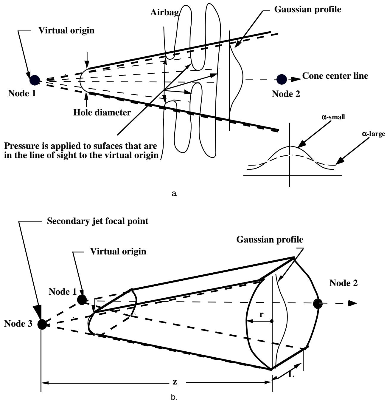
Figure 58.1 Jetting configuration for (a.) driver's side airbag (pressure applied only if centroid of surface is in line-of-sight) and (b.) the passenger's side bag.
