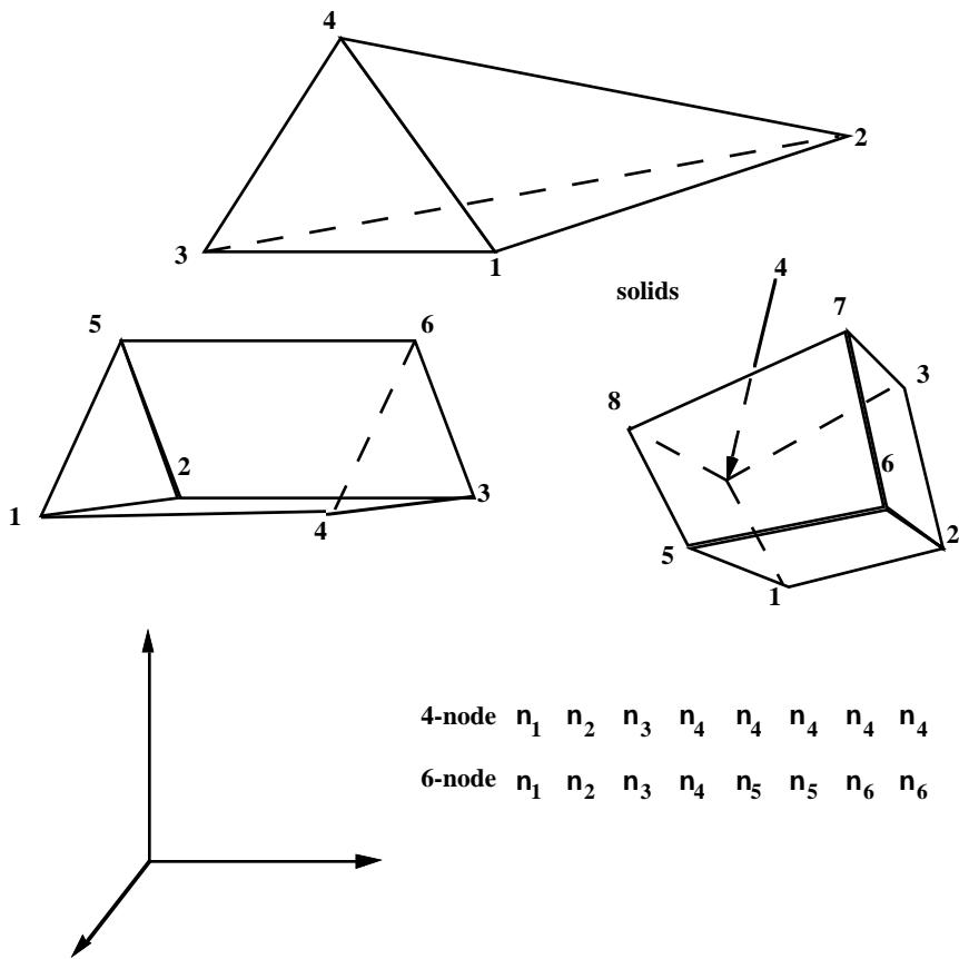
Figure 7.1. Four, six, and eight node solid elements.
