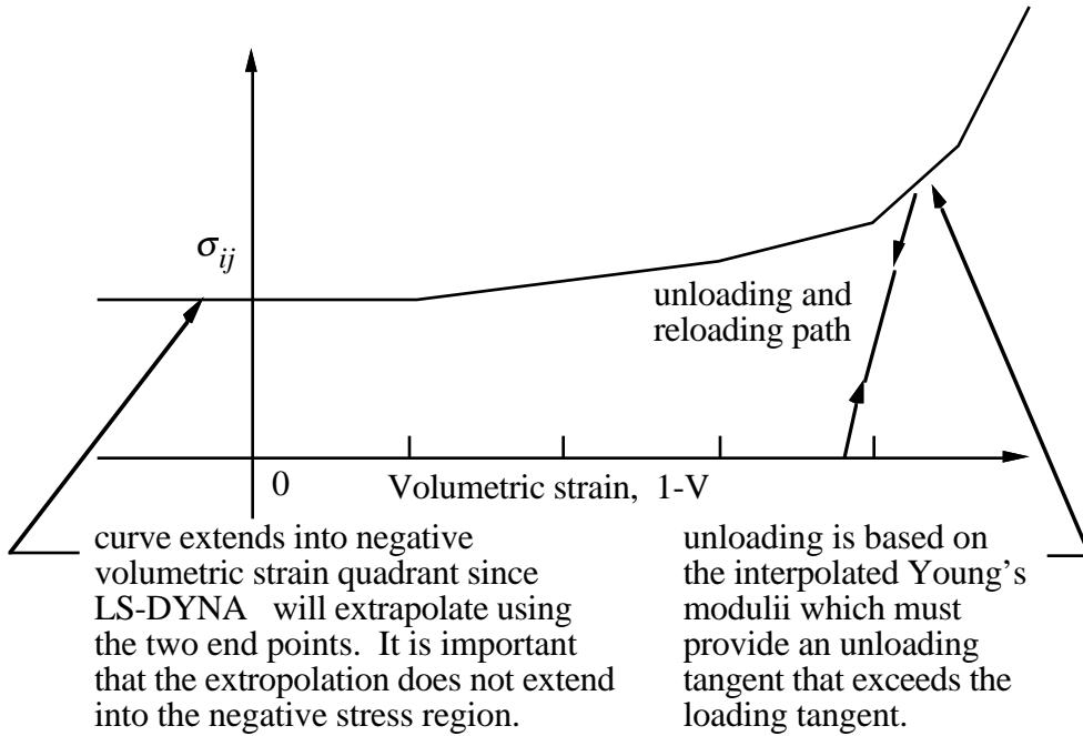
Figure 3.11. Stress quantity versus volumetric strain. Note that the “yield stress” at a volumetric strain of zero is nonzero. In the load curve definition the “time” value is the volumetric strain and the “function” value is the yield stress.
