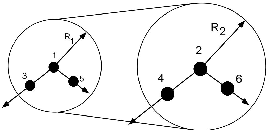
Figure 39.7. Pulley joint. Nodal pairs (1,3) and (2,4) define axes that are orthogonal to the pulleys. Nodal pairs (1,5) and (2,6) define vectors in the plane of the pulleys. The ratio  $\frac{R_2}{R_1}$  is specified.
