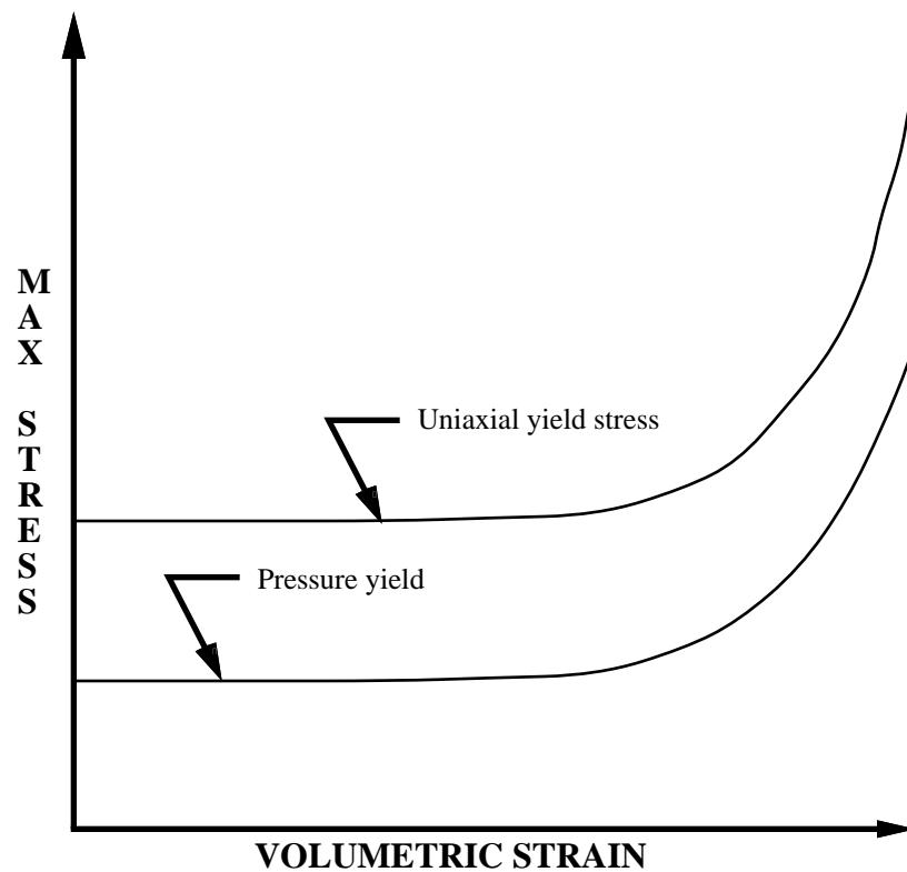
Figure 3.24. Behavior of crushable foam. Unloading is elastic.
