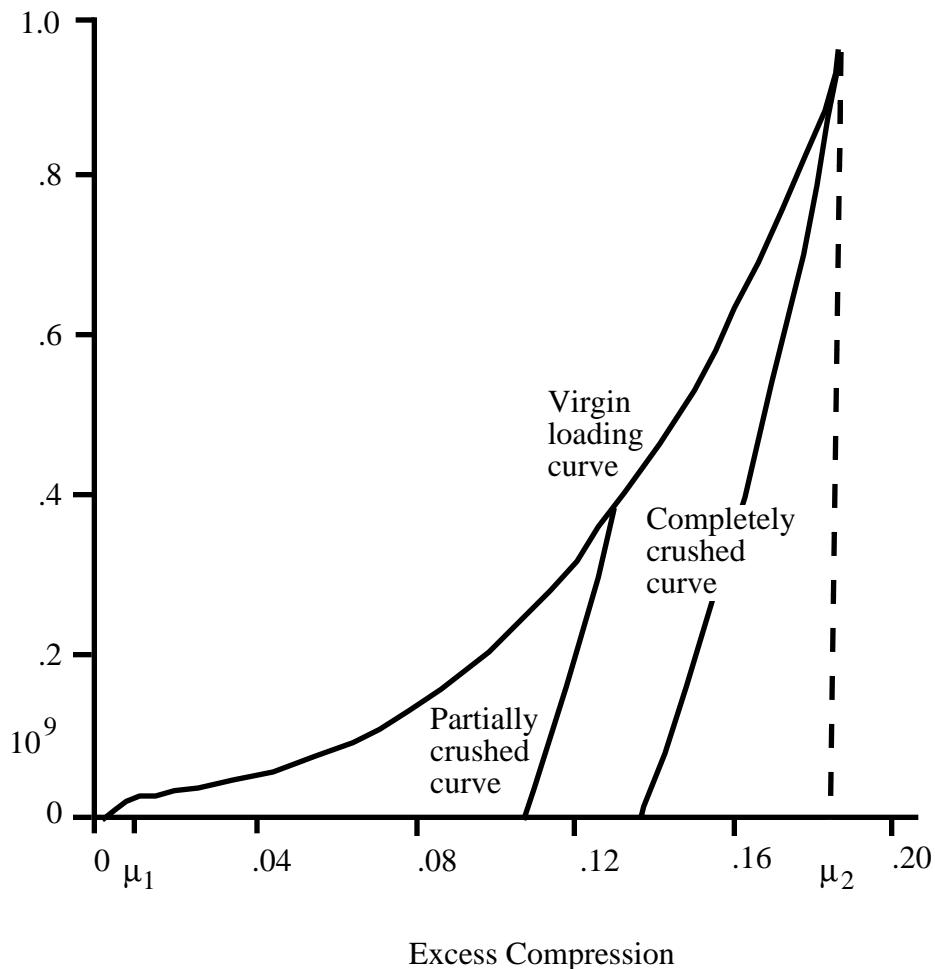
Figure 3.33. Pressure versus compaction curve.
