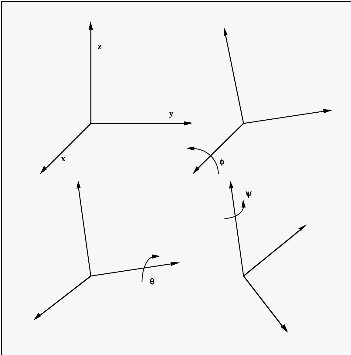
Figure 39.9. Definition of angles for the generalized joint stiffness. The magnitude of the angular rotations are limited by the stop angles defined on Card 5.
