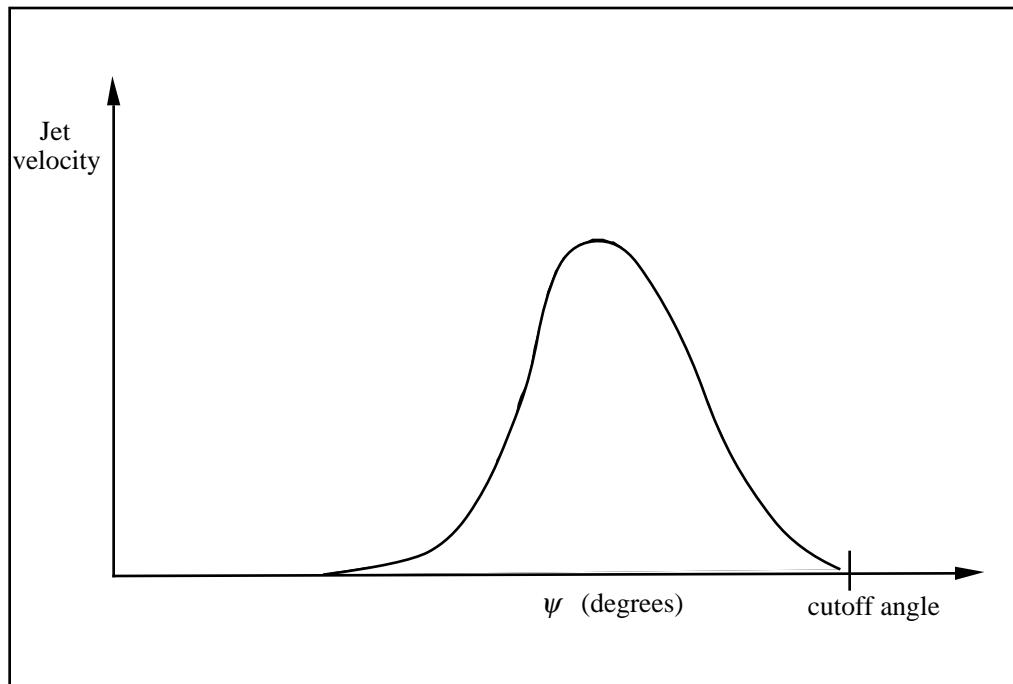
Figure 58.3. Normalized jet velocity versus angle for multiple jet drivers side airbag.
