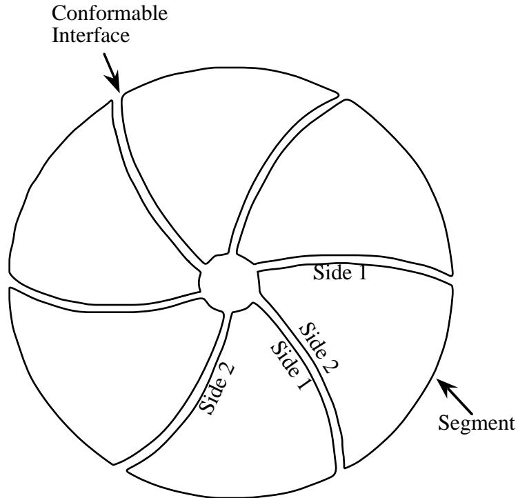
Figure 68.1. With cyclic symmetry only one segment is modeled.
