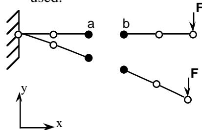
**Offset nodes a and b are constrained to move together.**
