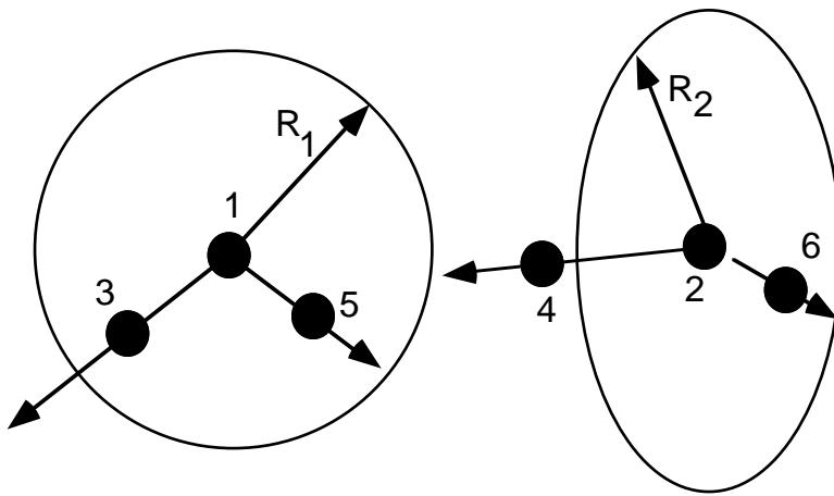
Figure 39.4. Gear joint. Nodal pairs (1,3) and (2,4) define axes that are orthogonal to the gears. Nodal pairs (1,5) and (2,6) define vectors in the plane of the gears.
