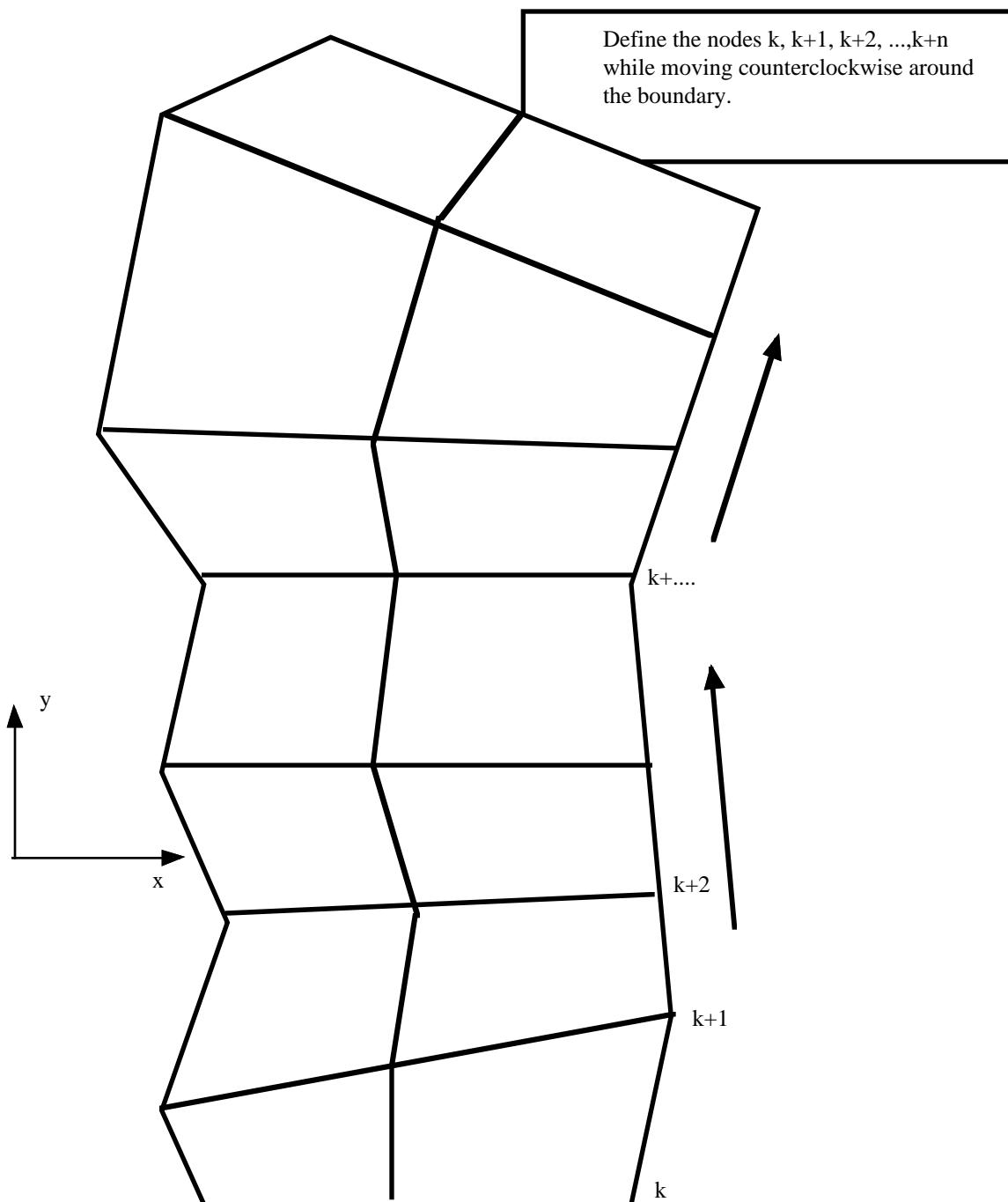
Figure 54.1 When defining a transmitting boundary in 2D define the node numbers consecutively while moving counterclockwise around the boundary.
