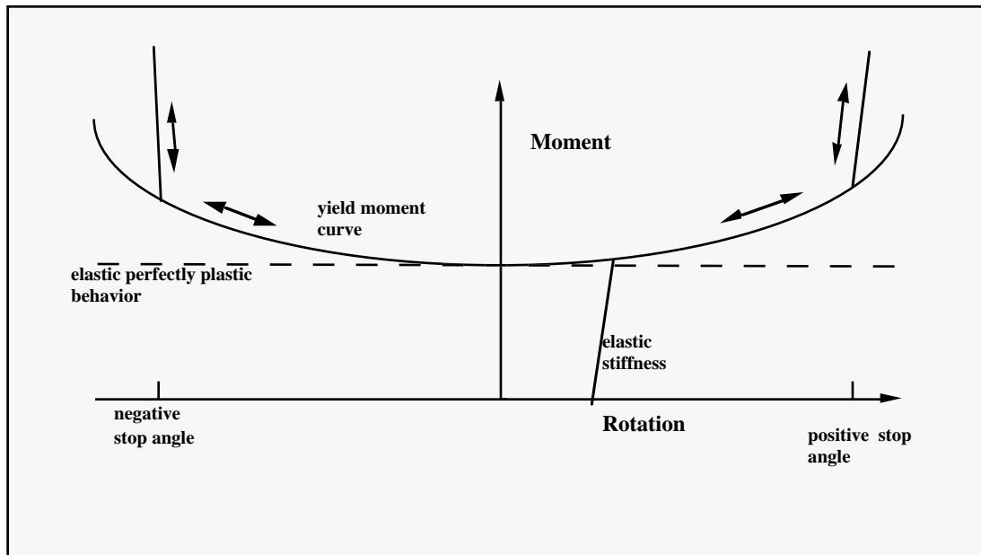
Figure 39.10. Frictional behavior is modeled by a plasticity model. Elastic behavior is obtained once the stop angles are reached.
