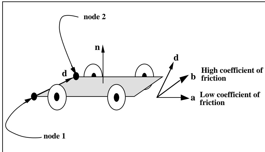
Figure 28.2. Definition of orthotropic friction vectors. The two methods of defining the vector,  $\underline{d}$  are shown. If vector  $\underline{d}$  is defined by nodes 1 and 2, the local coordinate system may rotate; otherwise,  $\underline{d}$  is fixed in space and the local system is stationary.
