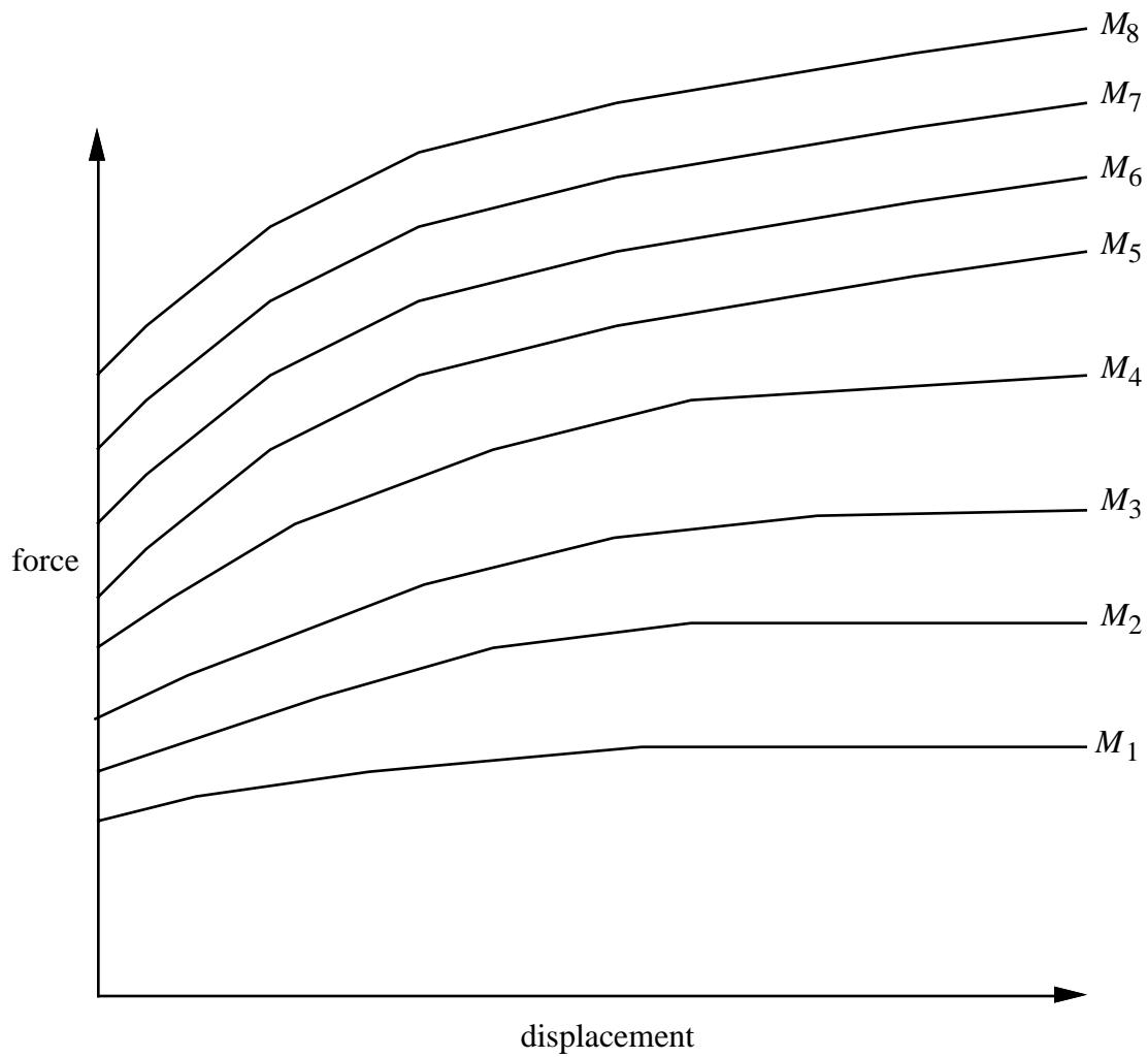
Figure 3.14. The force magnitude is limited by the applied end moment. For an intermediate value of the end moment LS-DYNA interpolates between the curves to determine the allowable force value.
