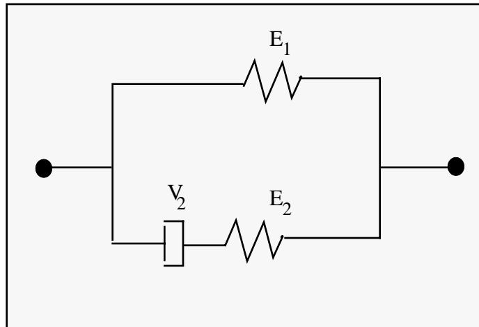
Figure 3.17. Schematic of material model 62.
