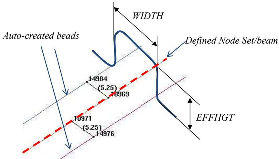
Figure 11-4. Illustration – definition of multiple draw beads.
