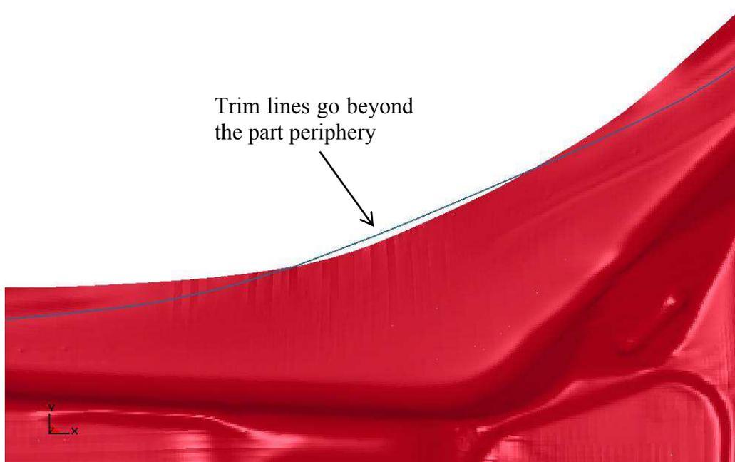
Figure 15-15. R6 Revision 68643 enables trimming for cases where trim lines go beyond part boundary
