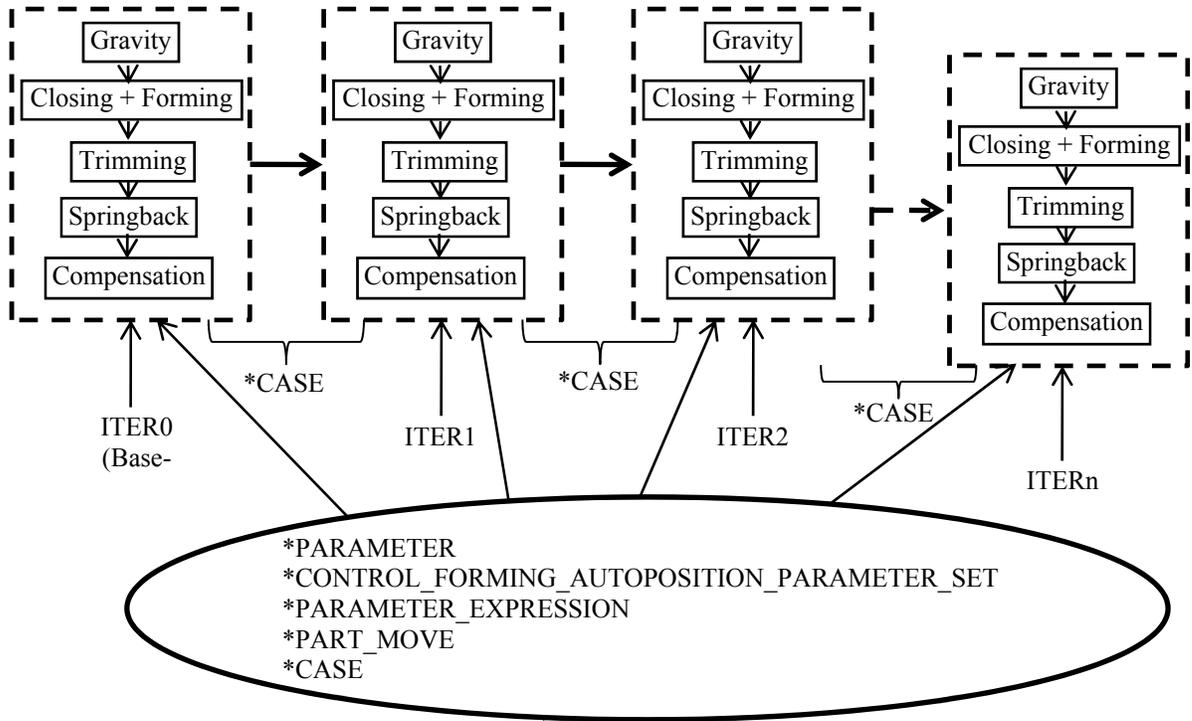
Figure 25-19. Based on a specific stamping die process, a fully automatic and iterative springback compensation loop is possible and shown in the flow chart below.
