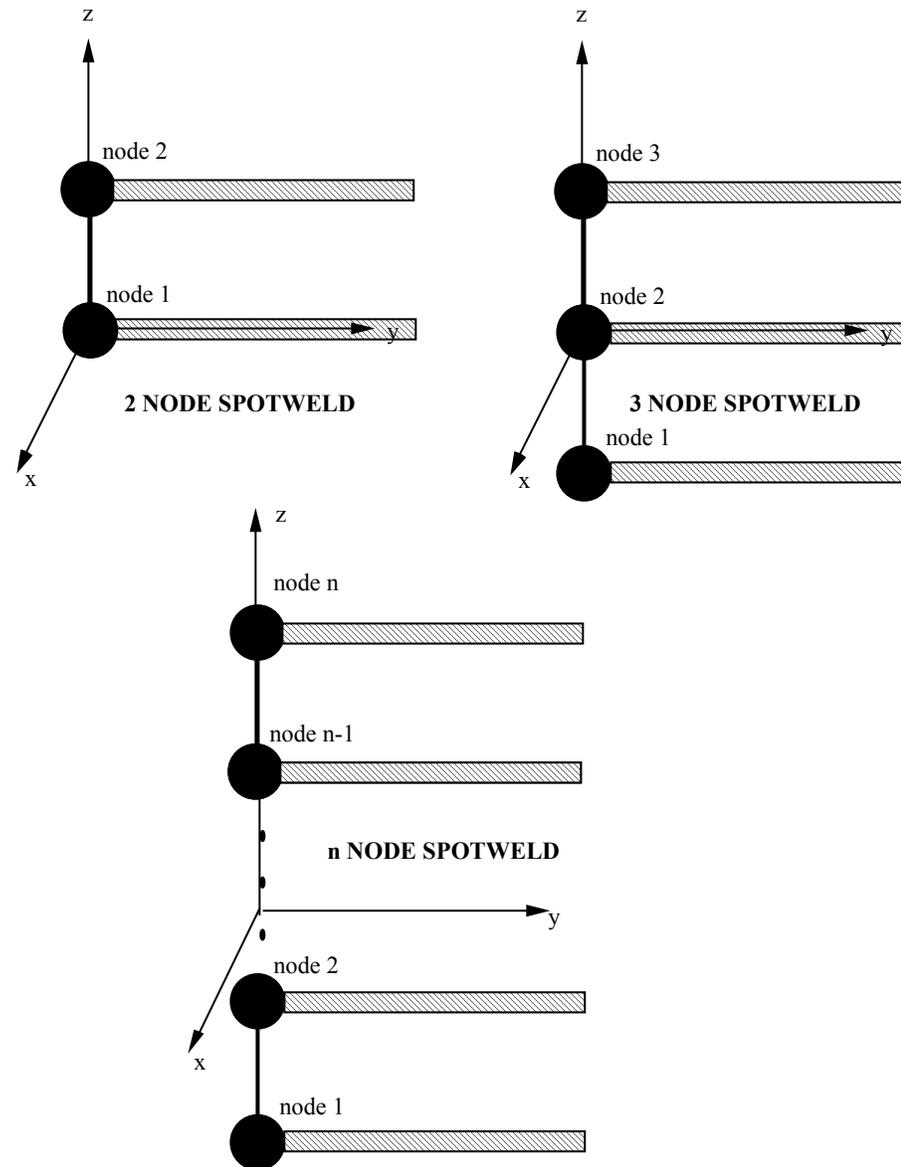
Figure 10-5. Nodal ordering and orientation of the local coordinate system is important for determining spotweld failure.
