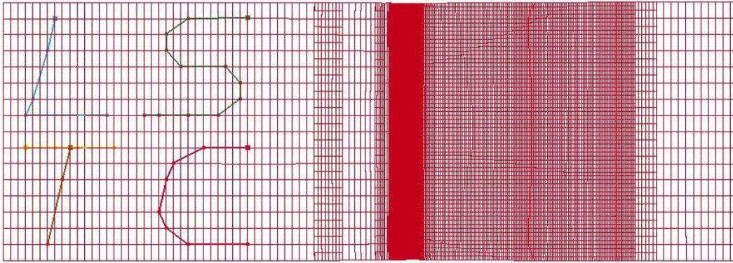
Figure 15-18. Curves used for mesh refinement can be discontinuous and written in one IGES file.
