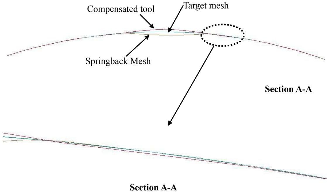
Figure 15-7. Localized Compensation Results along Section A-A
