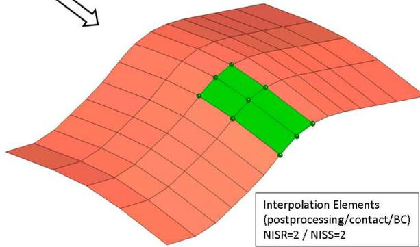
Figure 18-17. Example of a bi-quadratic \*ELEMENT\_SHELL\_NURBS\_PATCH keyword definition
