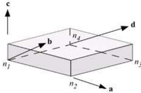
Figure 27-3. Material axes option
