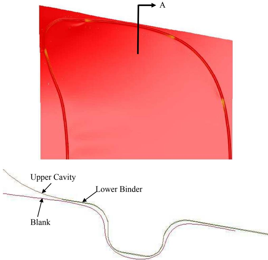
Figure 12-42. Closing with beads (Lower Binder with Contact Offset of 2.2mm)
