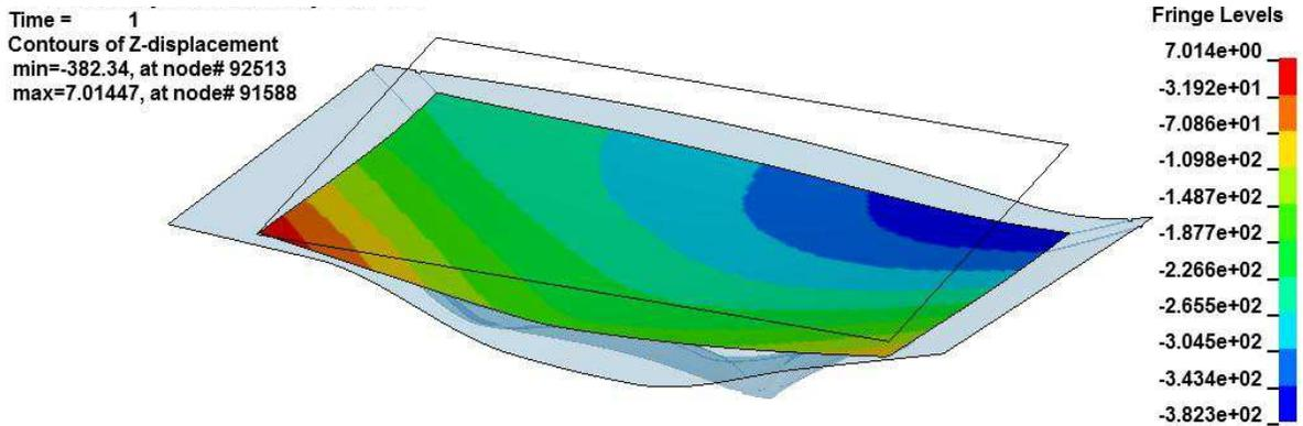
Figure 12-36. Gravity Loading of a Box Side Outer (Courtesy of Autodie, LLC)
