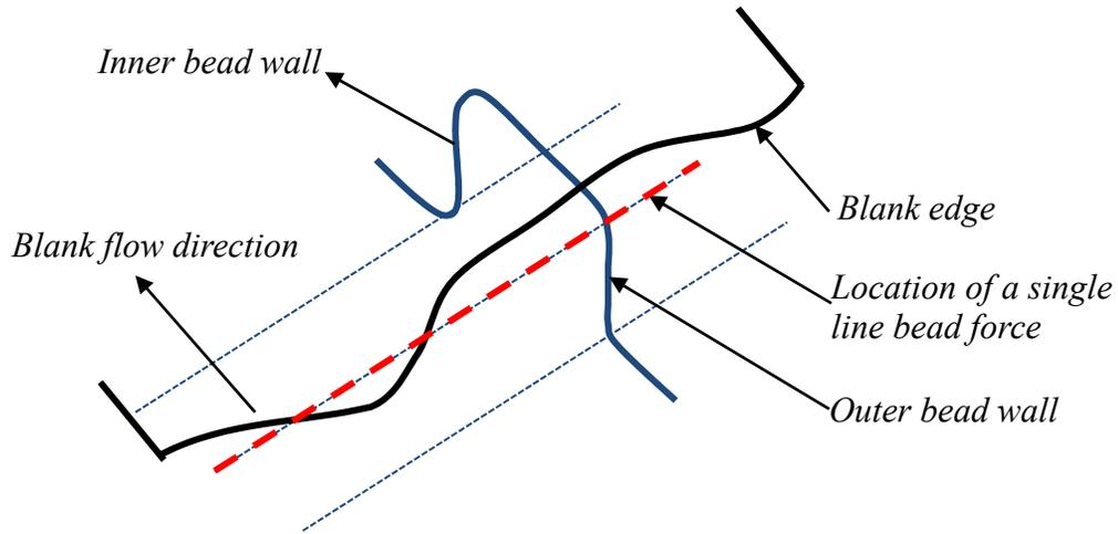
Figure 11-3. A possible scenario of sheet blank edge draw-in condition.
