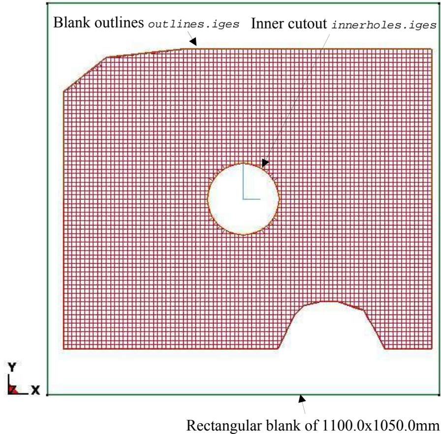
Figure 15-28. Using an IGES outline and an inner cutout curve to create a blank with any arbitrary shape.
