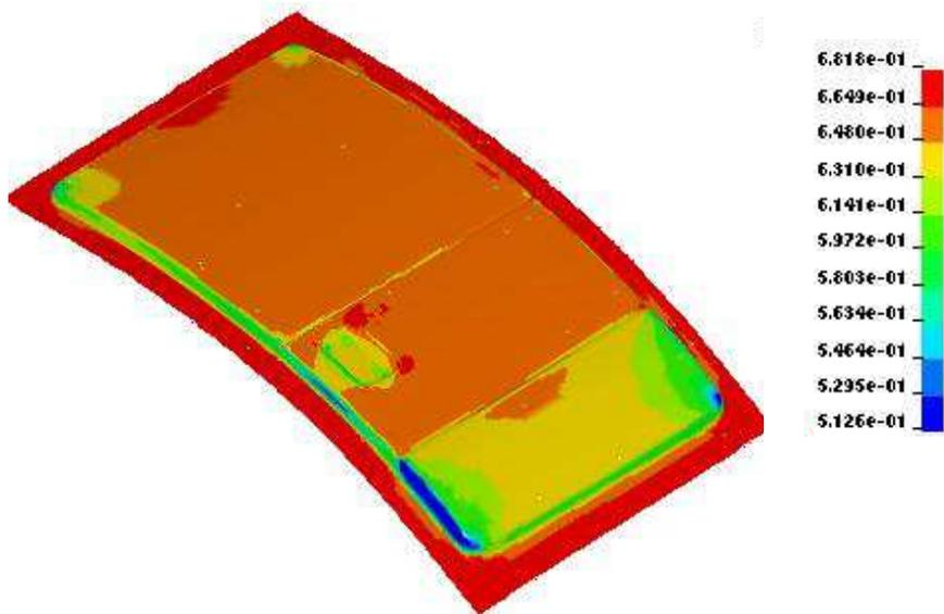
Figure 12-23. Thickness contour of the panel after draw simulation
