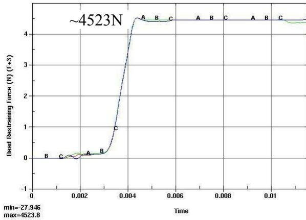
Bead forces on each bead for NBEAD=3
