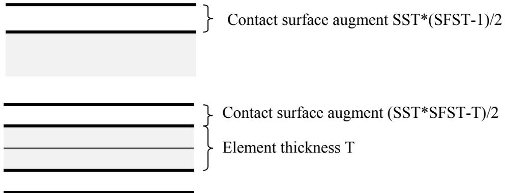
Figure 11-9. Illustration of contact surface location for automatic Mortar contact, solids on top and shells below.
