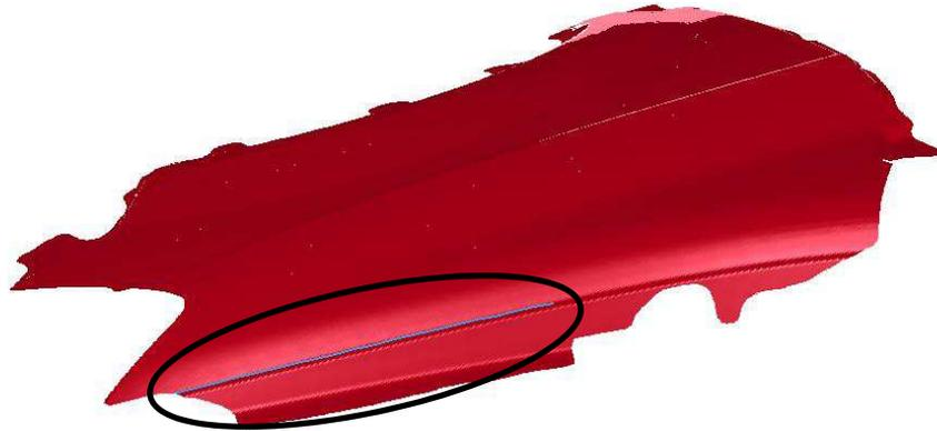
Figure 15-20. A more complex mesh refinement example (NUMISHEET2002 Fender)
