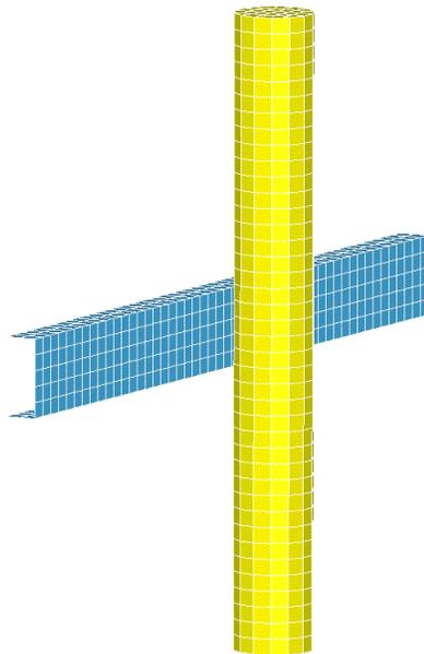
Figure 44-3. Impact between a user-defined shell and user-defined solid part.
