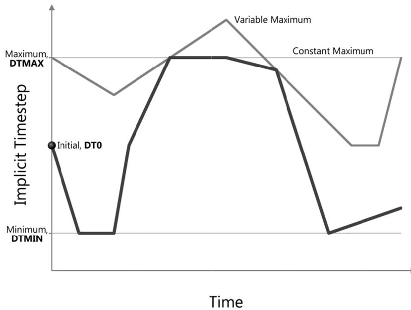
Figure 12-33. The implicit time step size changes continuously as a function of convergence within the bounds set by DTMIN and DTMAX
