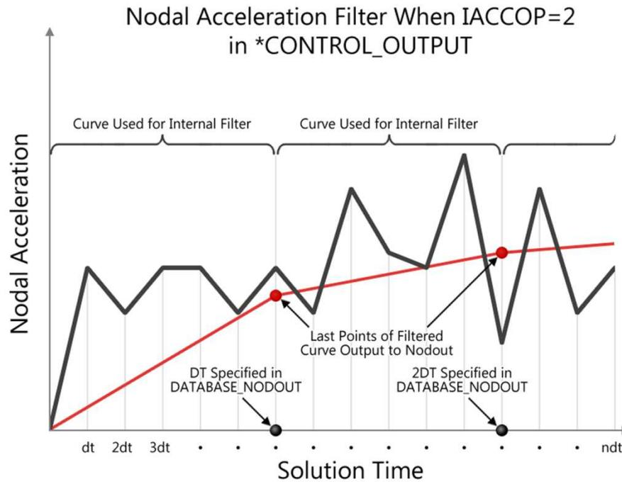
Figure 12-50. Nodal Acceleration Filter for IACOOP=2
