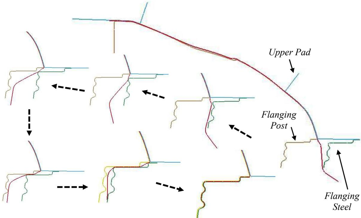
Figure 12-46. Fender flanging along hood line – mean stress (compression/surface lows in red) Deformed shape along section B.
