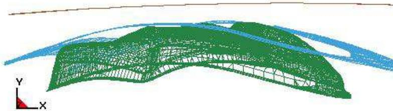
Figure 12-19. Pre-bending with R=10000.0mm using this keyword (1<sup>st</sup> state of D3nlots)
