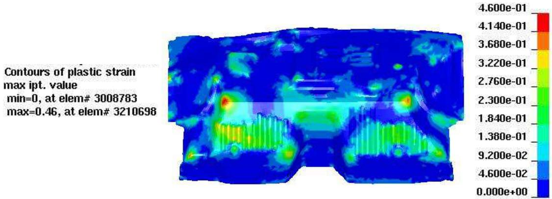
Figure 12-10. Effective plastic strain Prediction
