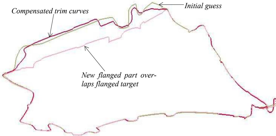
Figure 25-16. Compensated trim curves overlap with the target curves
