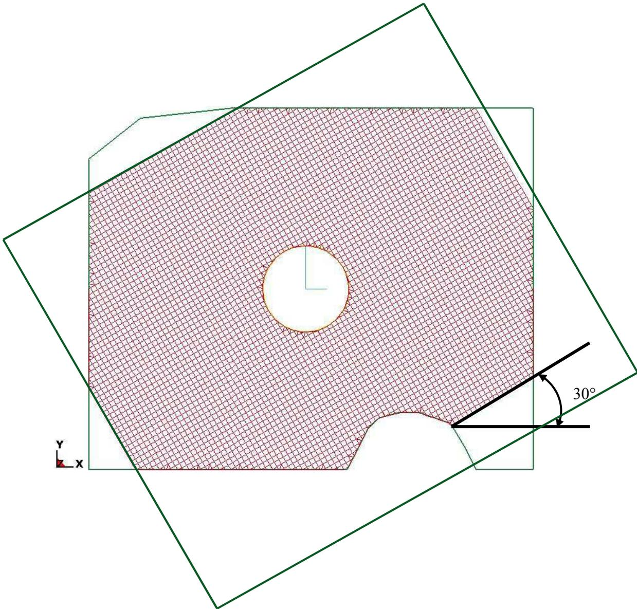
Figure 15-29. Set ANGLEX=30.0 to rotate both the blank and mesh orientation by 30°
