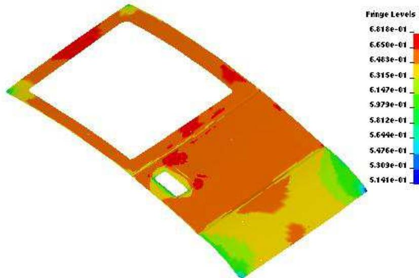
Figure 12-25. Springback amount (mm).
