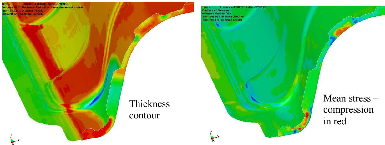
Figure 12-48. A flanging simulation of a rear floor pan using IOPTION 1 (Courtesy of Chrysler, LLC)
