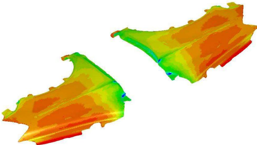
Figure 15-14. A double-attached drawn part trimmed into two pieces with NSEED1/NSEED2 (thickness/thinning plot)
