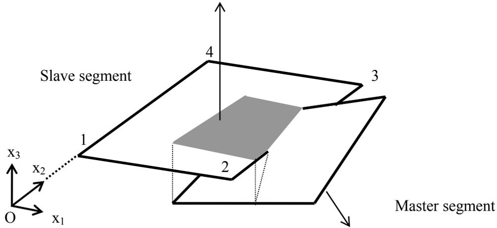
Figure 11-11. Illustration of Mortar segment to segment contact
