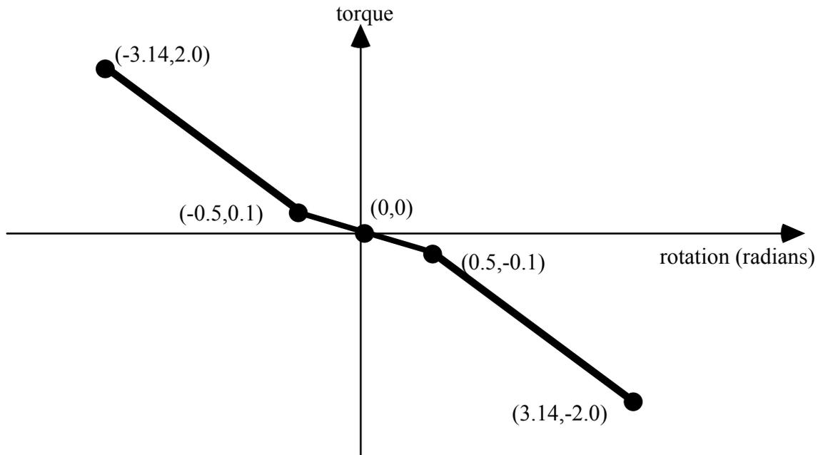
Figure 55-2 Characteristic torque curve shape used by all joints.
