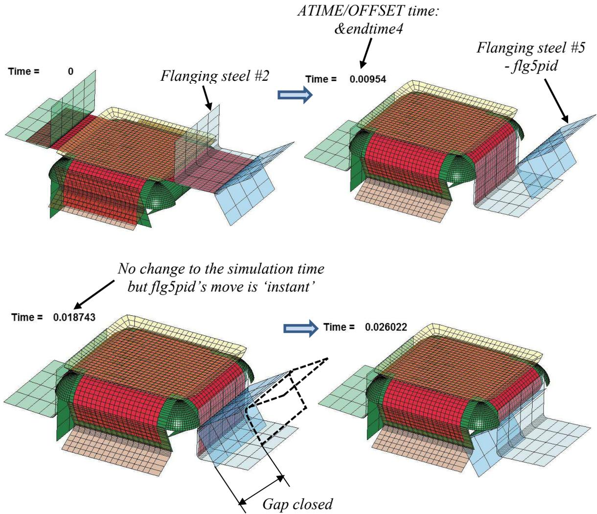
Figure 11-13. Closing a gap distance in a sequential flanging process.
