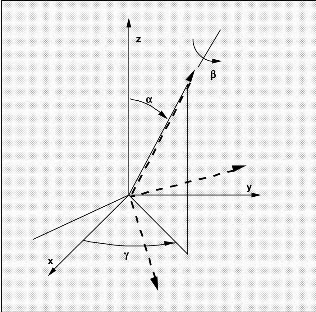
Figure 10-22. Flexion-torsion joint angles. If the initial positions of the local coordinate axes of the two rigid bodies connected by the joint do not coincide, the angles,  $\alpha$  and  $\gamma$ , are initialized and torques will develop instantaneously based on the defined load curves. The angle  $\beta$  is also initialized but no torque will develop about the local axis on which  $\beta$  is measured. Rather,  $\beta$  will be measured relative to the computed offset.
