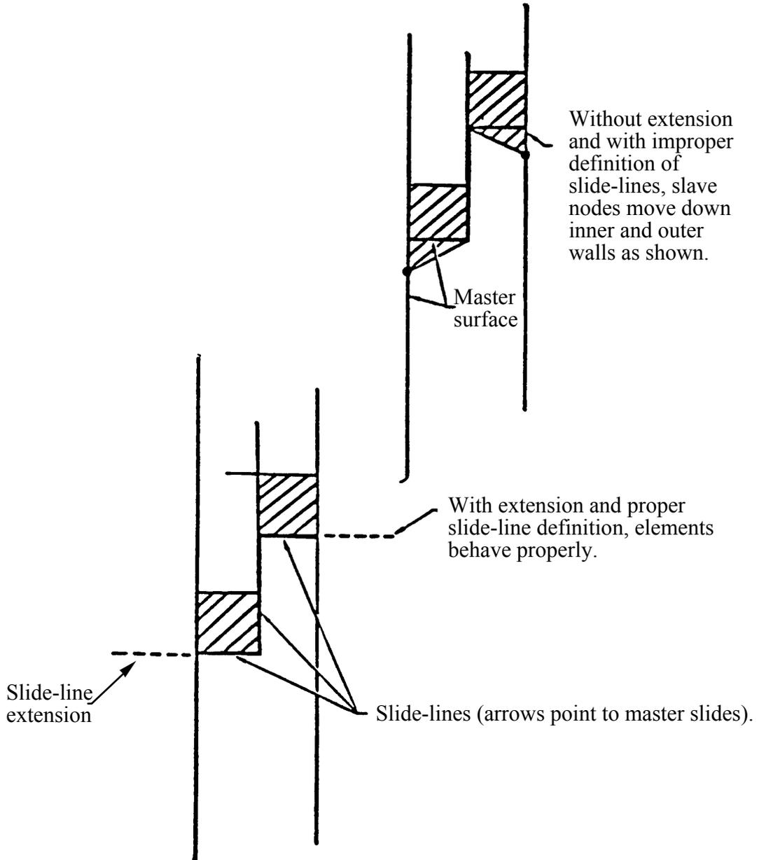
Figure 11-18. Example of slideline extensions helping to provide realistic response.
