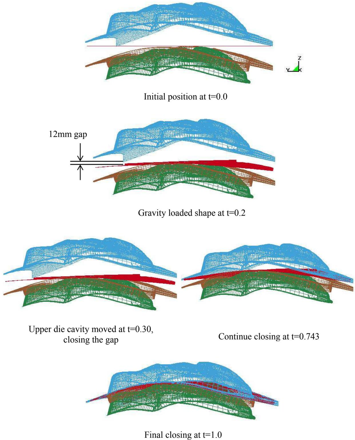
Figure 11-12. Automatic closure of gap in implicit static binder closing
