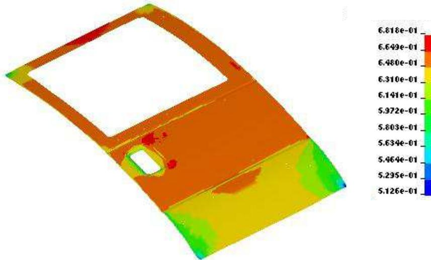
Figure 12-24. Thickness contour of the panel after trimming
