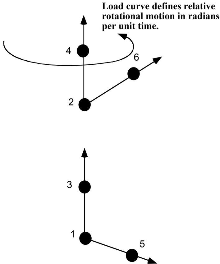
Figure 10-16. Rotational motor joint. This joint can be used in combination with other joints such as the revolute or cylindrical joints.
