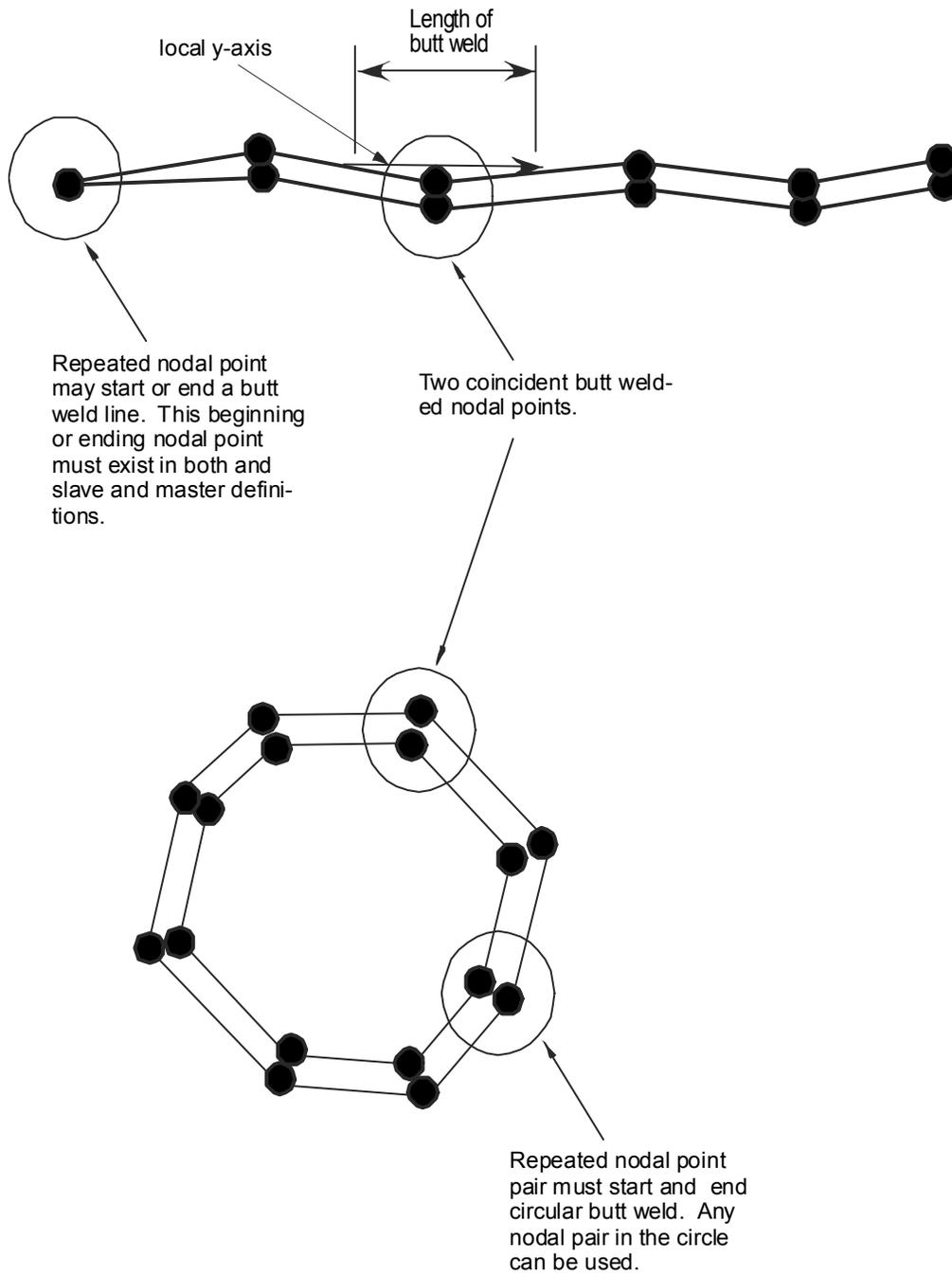
Repeated nodal point may start or end a butt weld line. This beginning or ending nodal point must exist in both and slave and master definitions.
