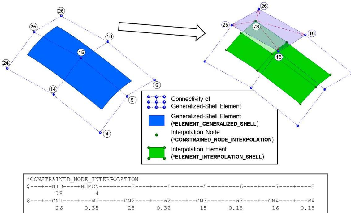
Figure 10-27. Example of a \*CONSTRAINED\_NODE\_INTERPOLATION card
