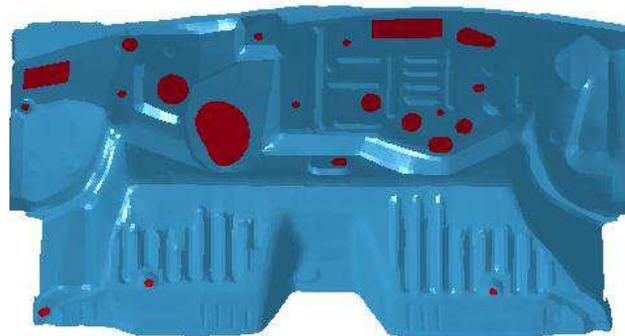
Figure 12-8. Trimmed-out holes dilled with LS-PrePost
