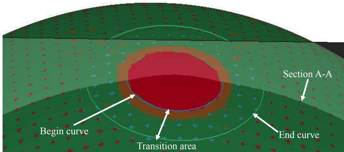
Figure 15-6. Localized Compensation Illustration
