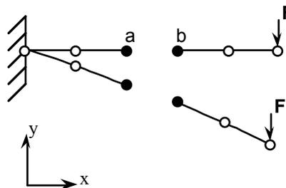
**Offset nodes a and b are constrained to move together.**
