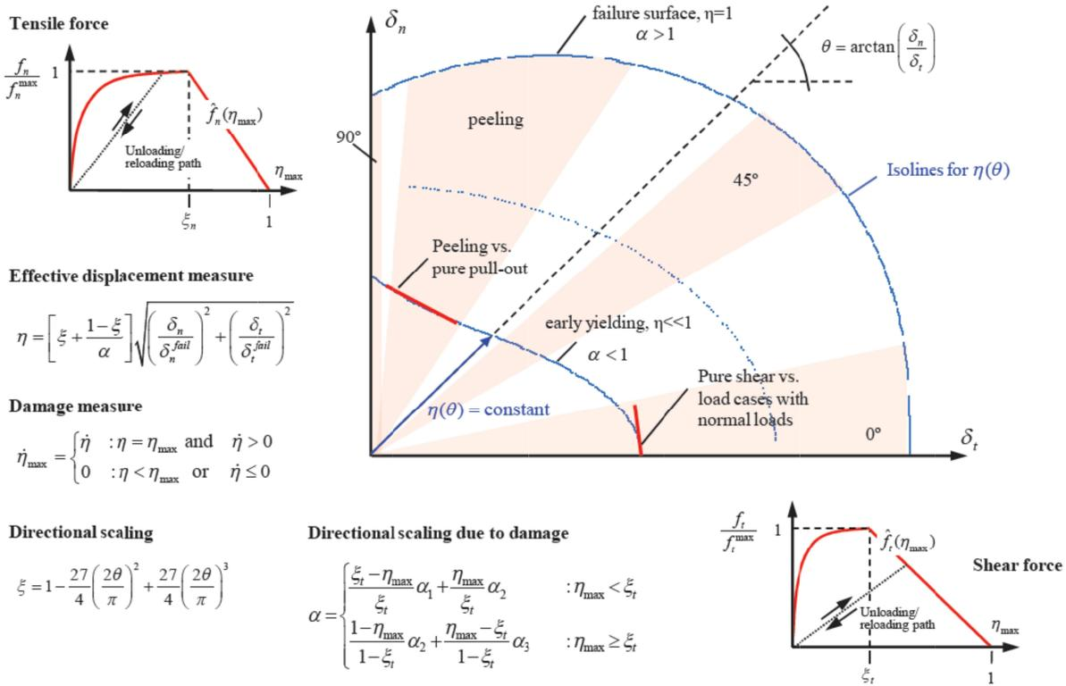
Figure 10-36. Mixed-mode behavior with effective displacement measure.
