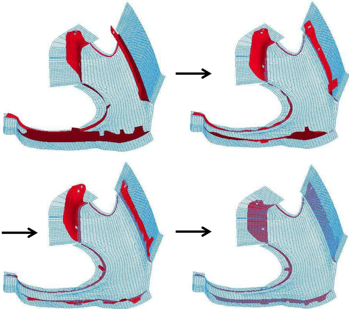
Flange unfolding progression of a fender outer
