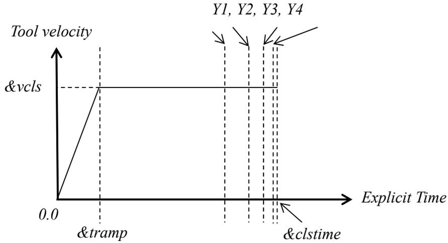
Specifying four additional D3PLOT outputs based on distance to punch home
