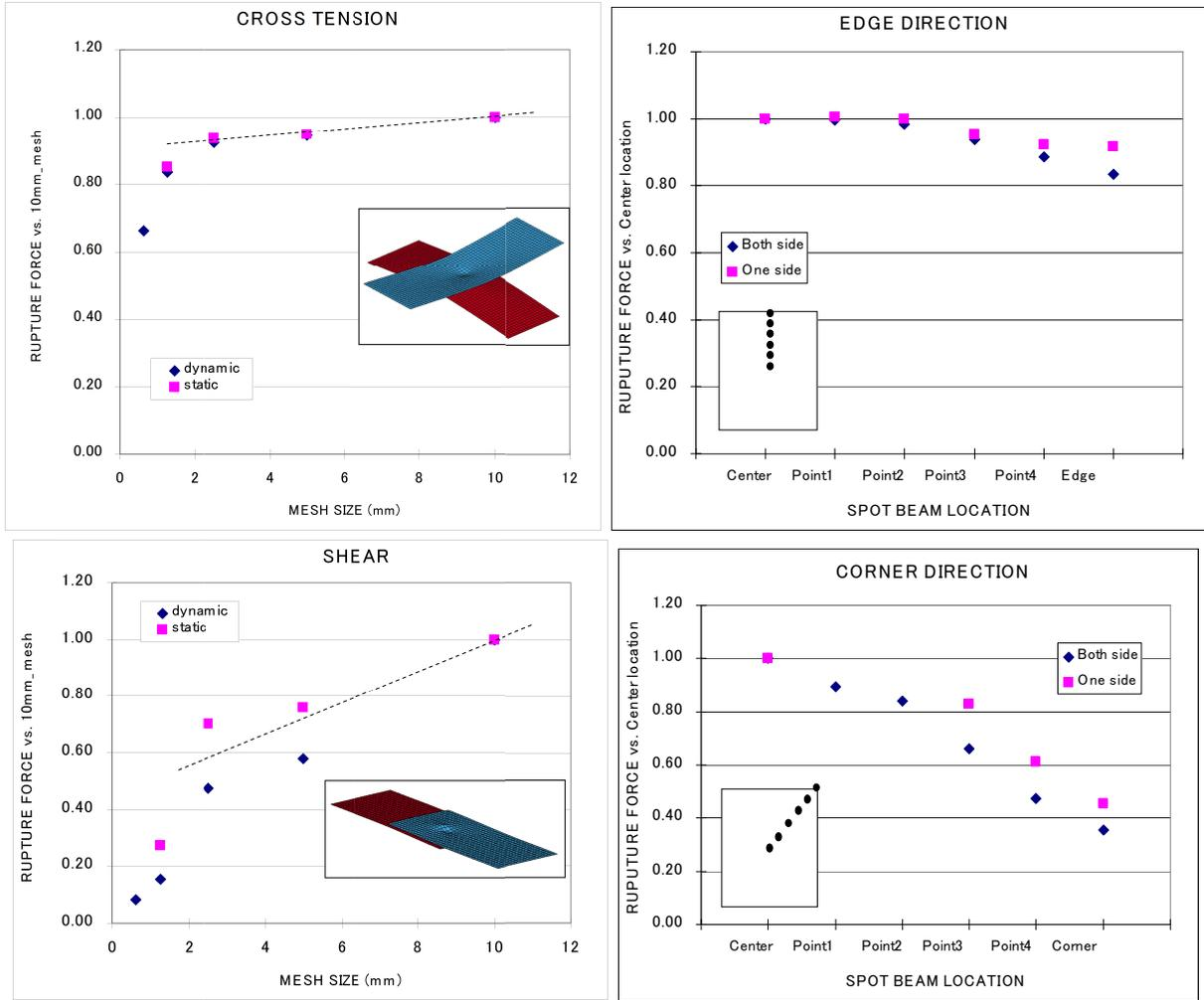
Figure 12-52 The failure force resultants can depend both on mesh size and the location of weld relative to the center of the contact segment.
