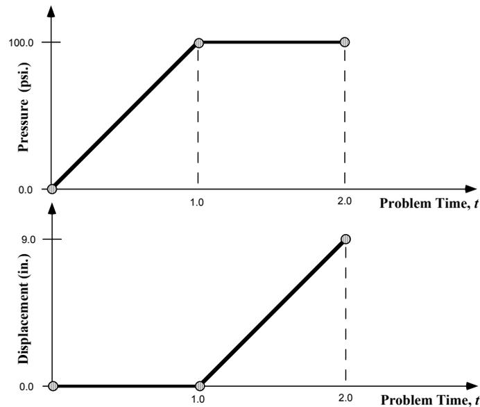
Figure 57-1. Load curves for a static simulation with two loading events. For convenience in this static simulation, the pressure loading is specified to begin at time 0.0 and end at time 1.0, and the displacement begins at time 1.0 and ends at time 2.0.
