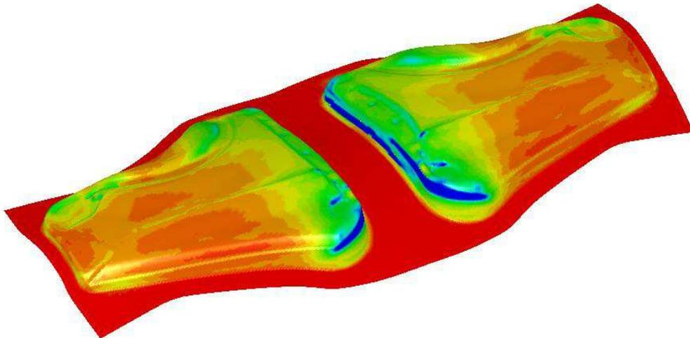
Figure 15-13. A double-attached drawn part (thickness/thinning plot)
