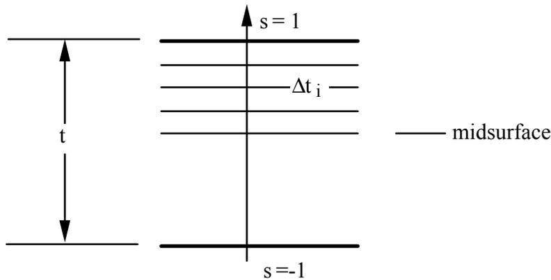
Figure 24-44. In the user defined shell integration rule the ordering of the integration points is arbitrary.
