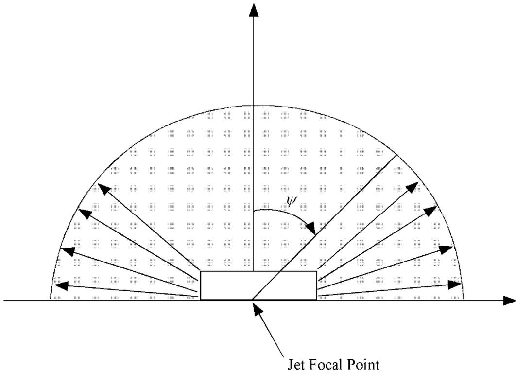
Figure 3-2. Multiple jet model for driver's side airbag
