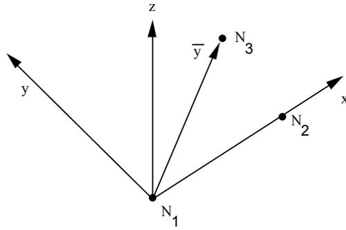
Figure 15-2. Definition of local coordinate system using three nodes when the node N2 lies along the x-axis.
