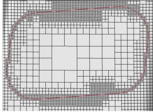
Figure 12-2. Refinement along a curve.
