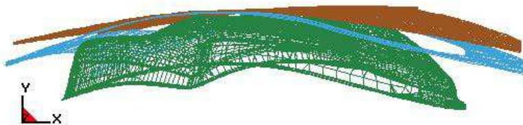
Figure 12-16. Pre-bending of a fender outer (*NUMISHEET 2002*) Gravity loaded shape (last state of D3plots) – Convex shape blank achieved and binder closing distance reduced
