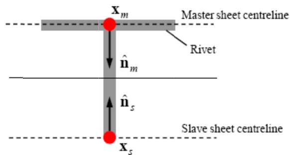
Figure 10-32. Single-sheet rivet system.
