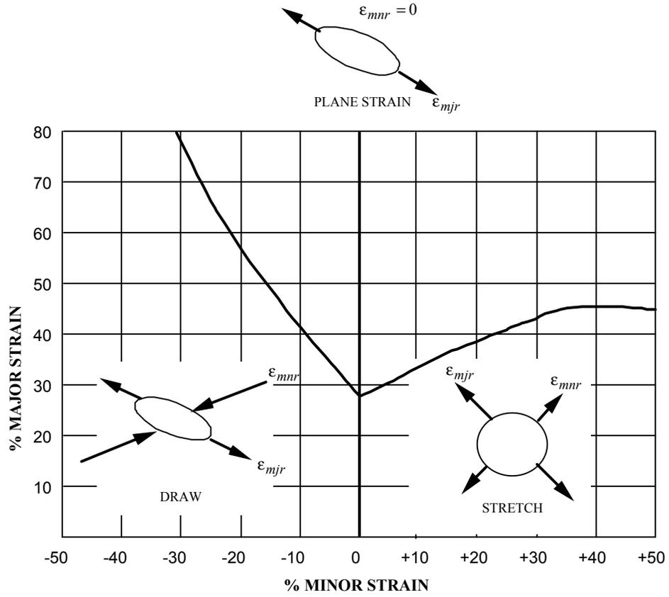
Figure 15-9 . Flow limit diagram
