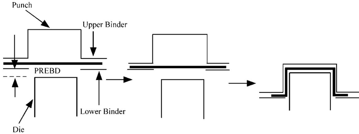
Figure 12-30. IDTEMP=3: Four-Piece Draw
