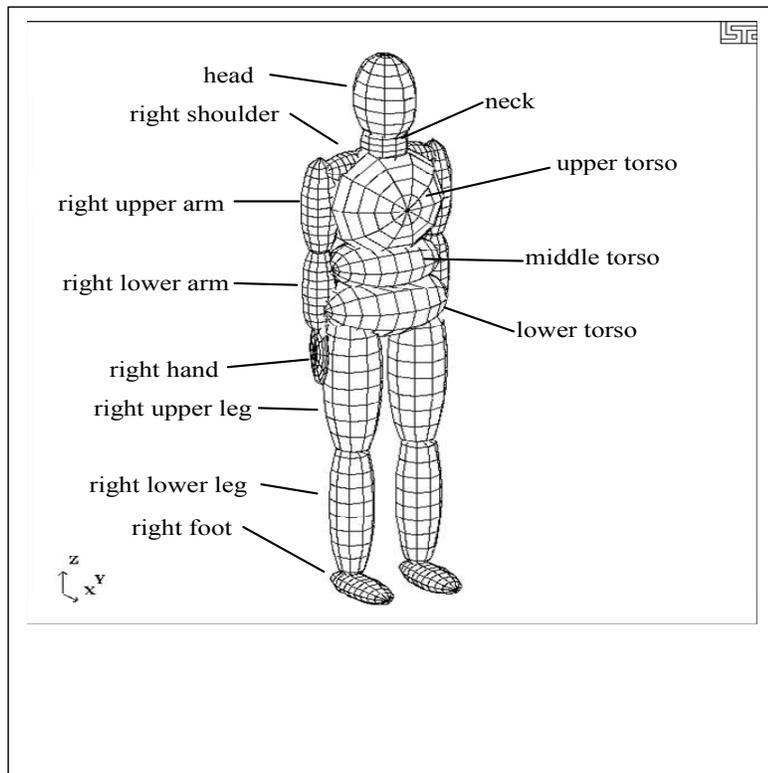
Figure 55-1. 50th percentile male dummy in the nominal position.
