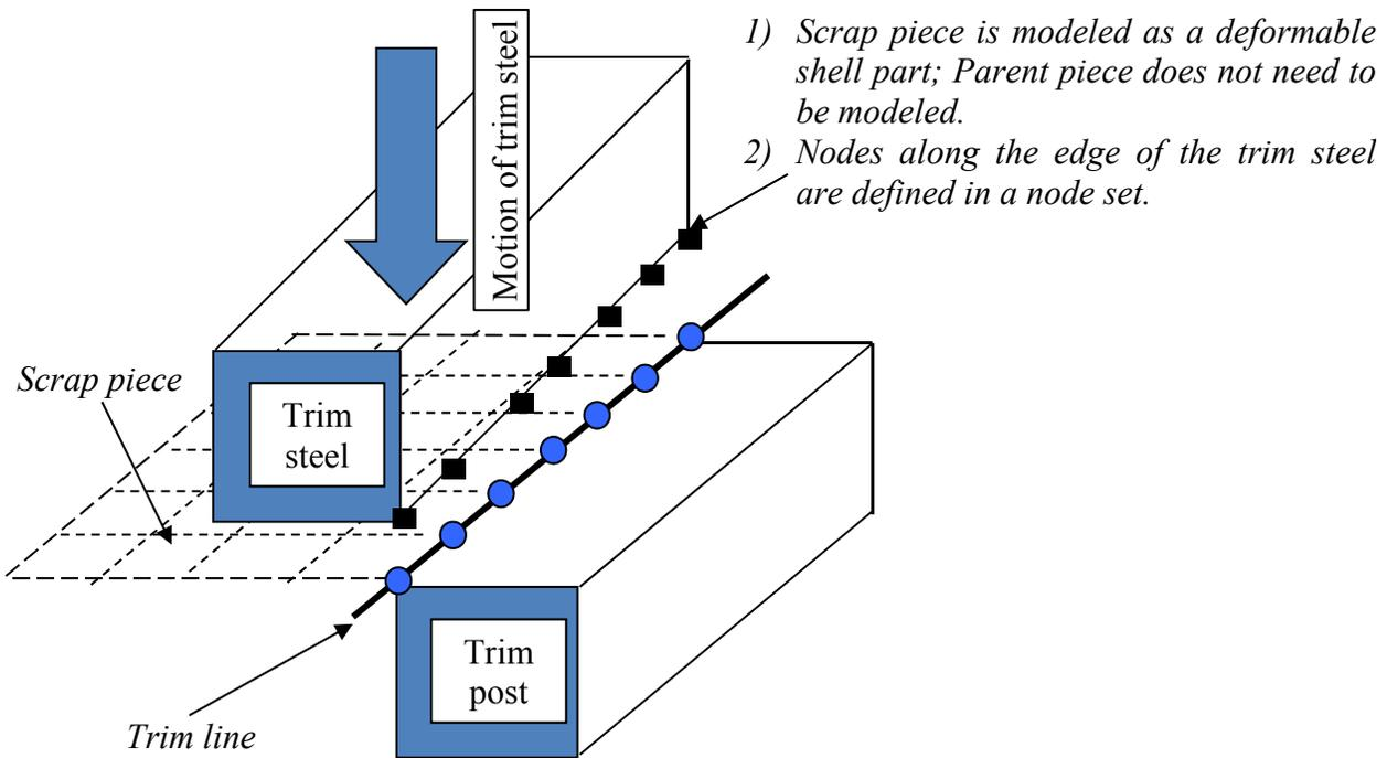
Figure 12-20. Modeling details for the scrap fall simulation. (Courtesy of Ford Motor Company)
