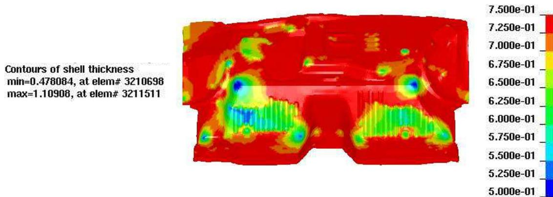
Figure 12-9. Sheet thickness prediction ( $t_0=0.75mm$ )
