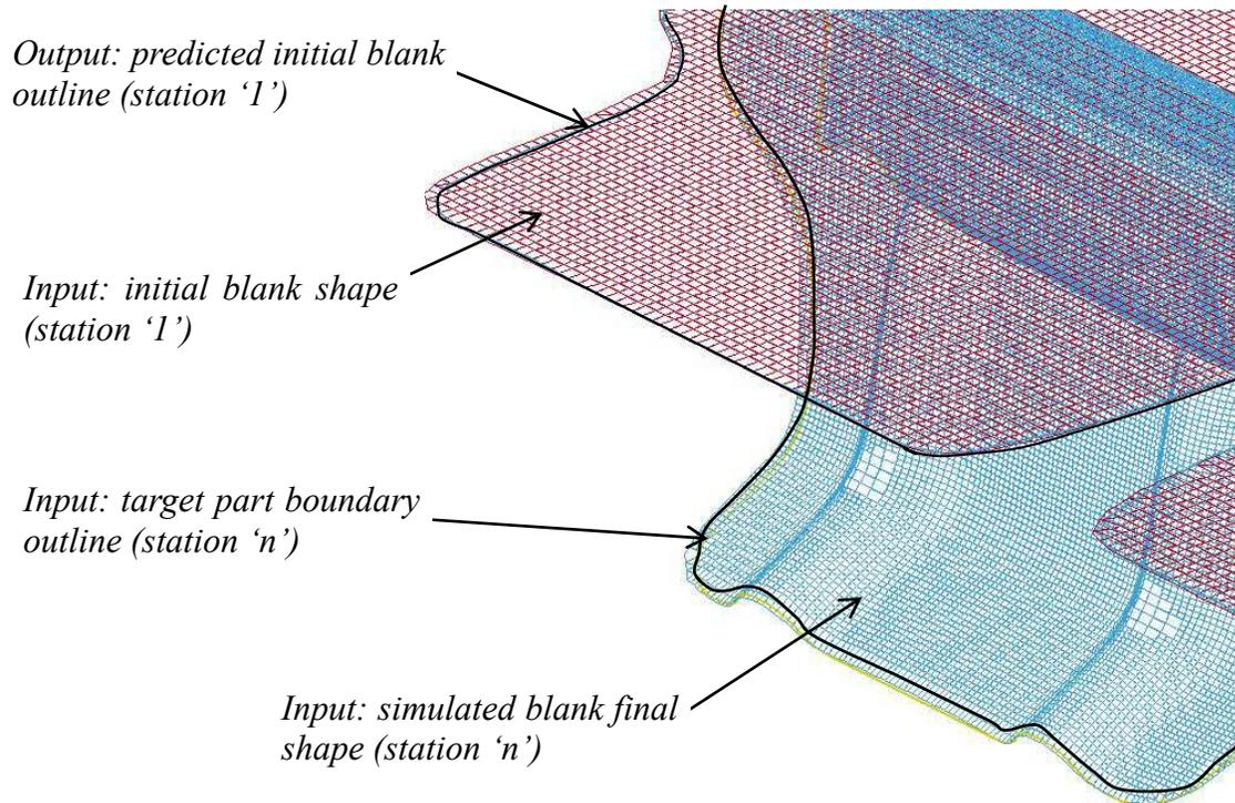
Figure 25-4. Blank size development in a progressive die with  $IADAPT=1$
