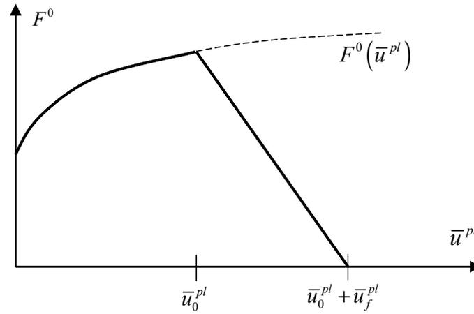
Figure 10-12. Force-displacement curve: plasticity and linear damage
