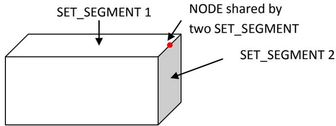
Figure 20-2. Nodes shared by two SET\_SEGMENT
