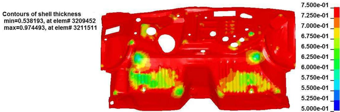
*Blank thickness without holes ( $t_0=0.75\text{mm}$ )*
