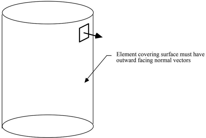
Figure 27-6. The shell elements interacting with the fluid must be numbered such that their outward normal vector points into the fluid media.
