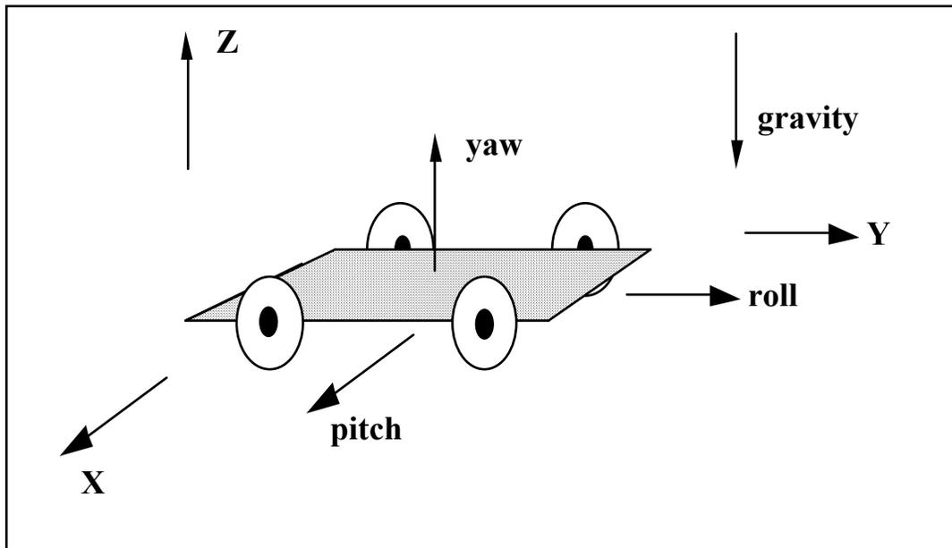
Figure 23-3. The vehicle pictured is to be oriented with a successive rotation sequence about the yaw, pitch, and roll axes, respectively. Accordingly, AAXIS=3, BAXIS=1, and CAXIS=2. The direction of gravity is given by GRAV=-3.
