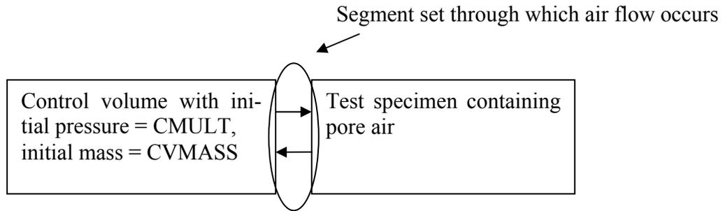
3. CVRPER allows users to model the porosity properties of the cover material. If SEGID is covered by a material of very low permeability (e.g., coated fabric), it is appropriate to set CVRPER=0. In this case,  $P_c$ , the pressure calculated assuming no boundary condition, is applied to SEGID. If SEGID is not covered by any material, it is appropriate to set CVRPER=1, the default value. In this case, the applied pressure becomes  $P_b$ , the boundary pressure determined by CMULT and LCID.
