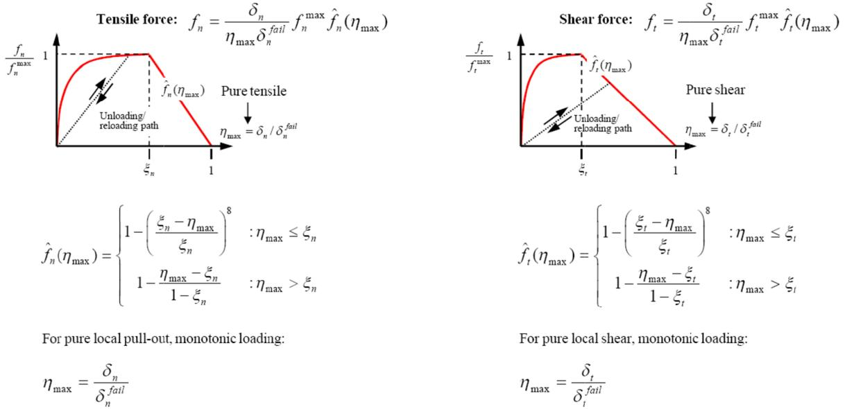
Figure 10-35. Force-deformation relationship: non-linear damage model.
