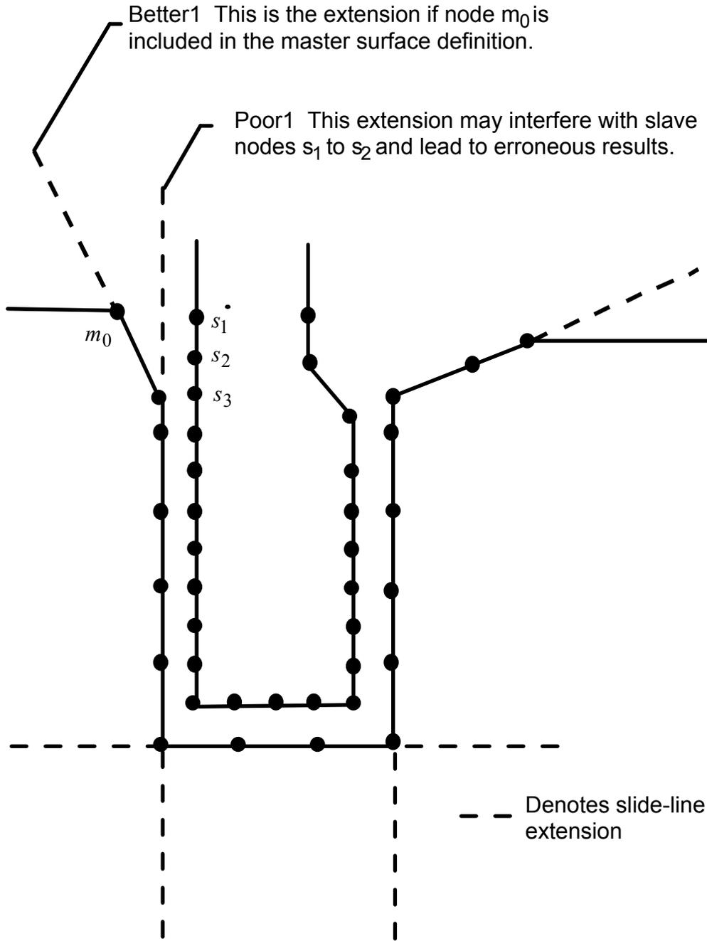
Figure 11-17. Master surface extensions defined automatically by DYNA (extensions are updated every time step to remain tangent to ends of master sides of slidelines unless angle of extension is defined in input).
