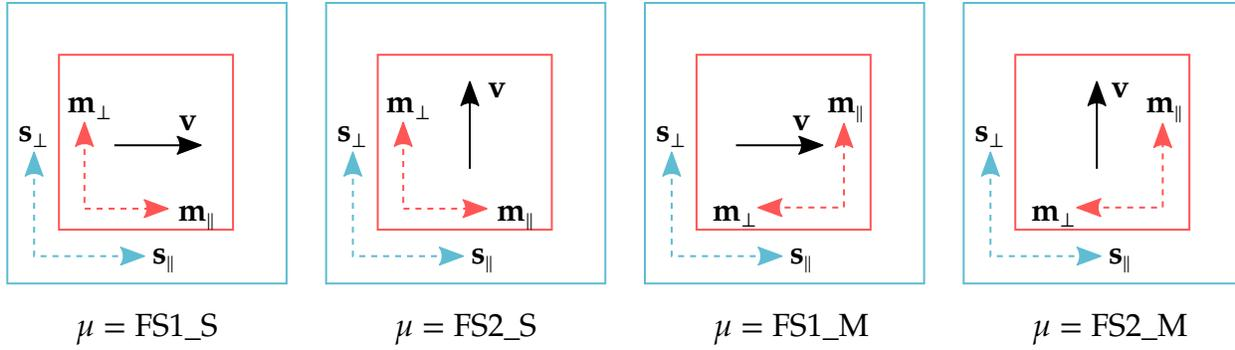
**Figure 11-12.** Interpretation of input parameters for Mortar orthotropic friction
