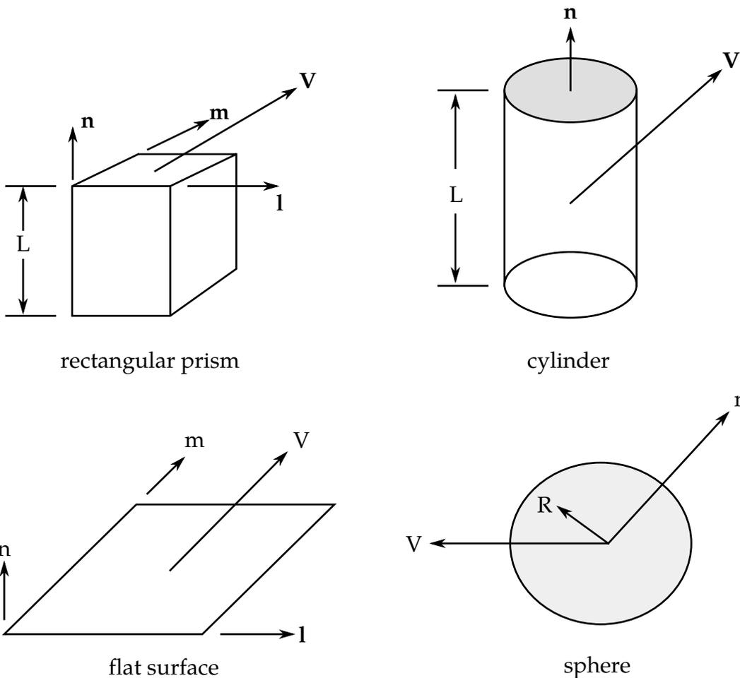
**Figure 38-1.** Vector  $n$  determines the orientation of the rigidwall. By including the MOTION option, motion of the rigidwall can be prescribed in any direction  $V$  as defined by variables  $VX, VY, VZ$ .
