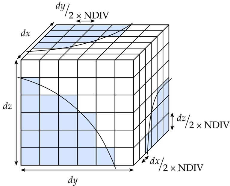
**Figure 4-2.** Division of an ALE element into  $8 \times \text{NDIV}^3$  sub-cells to compute the volume fractions of elements cut by the surface defined by SURFACT
