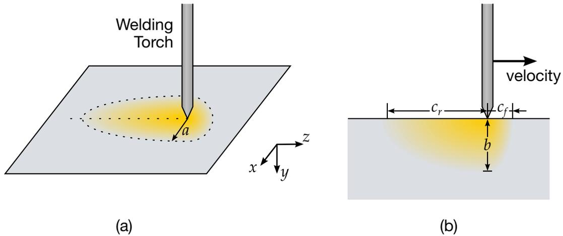
**Figure 5-11.** Schematic illustration of welding with moving torch. The left figure (a) shows the surface of the material from above, while the right figure (b) shows a slice along the dotted line in the  $y$ - $z$  plane.
