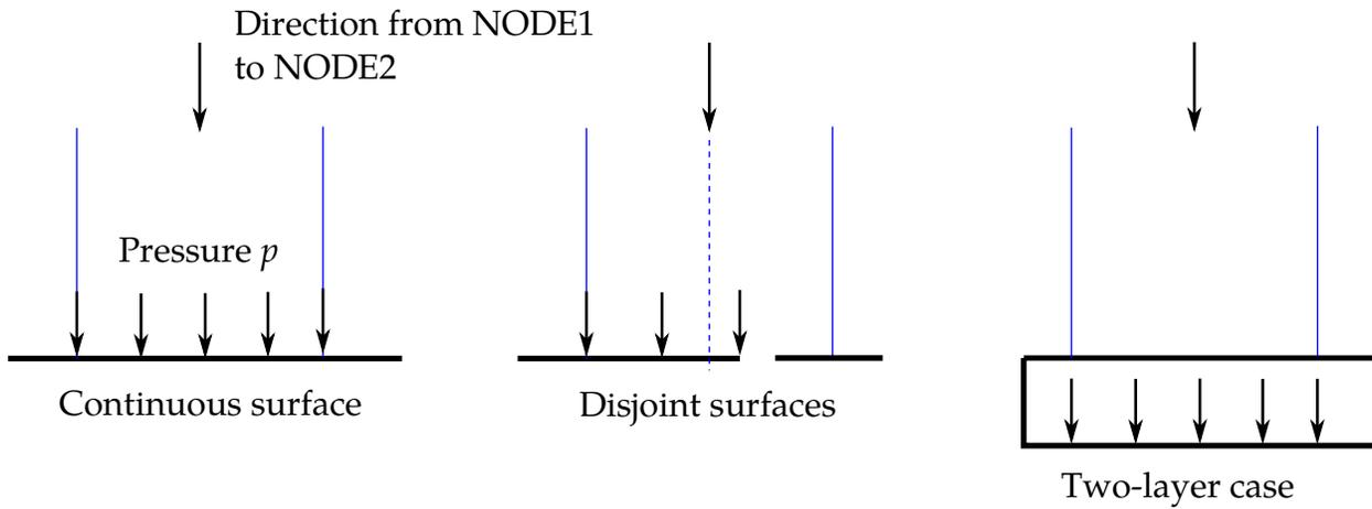
**Figure 31-6.** Applying pressure in SMP when LSFLG = 0
