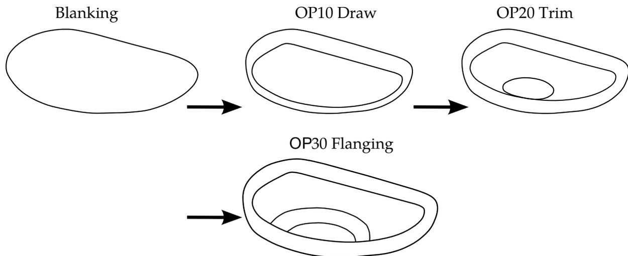
**Figure 29-4.** A stamping process consists of draw, trim and flanging (*Courtesy of Metal Forming Analysis Corporation*). The labels OP10, OP20, and OP30 are used *extensively* in the ensuing discussion.
