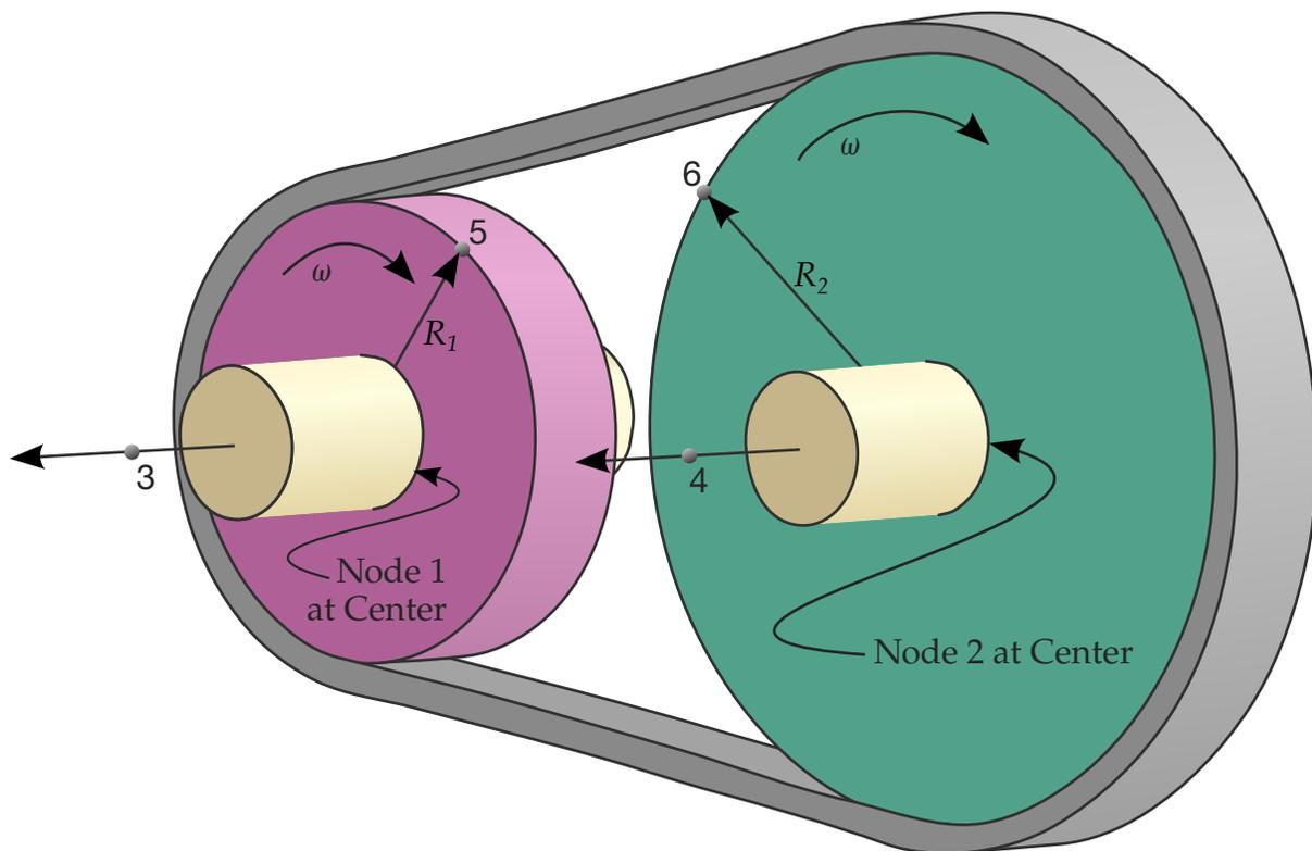
**Figure 10-28.** Pulley joint. Nodal pairs (1, 3) and (2, 4) define axes that are orthogonal to the pulleys. Nodal pairs (1, 5) and (2, 6) define vectors in the plane of the pulleys. The ratio  $R_2/R_1$  is specified.
