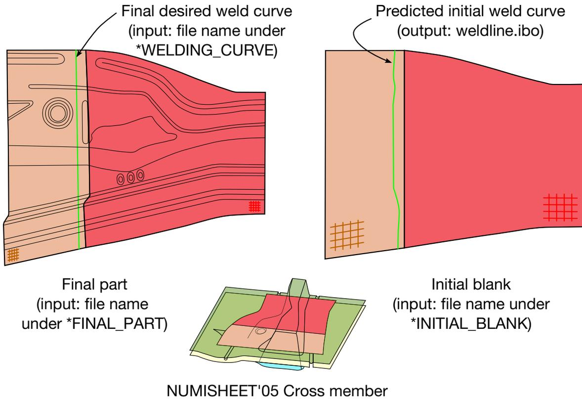
**Figure 29-41.** An example for a welding curve development.
