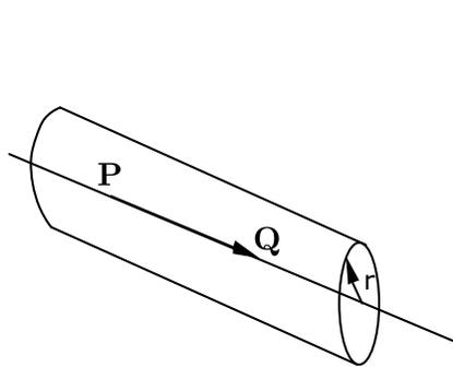
GEOTYP = 3: Infinite Cylinder
