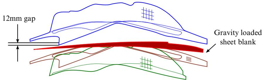
**Figure 11-21.** Gravity loading on blank at  $t = 0.2$ .
