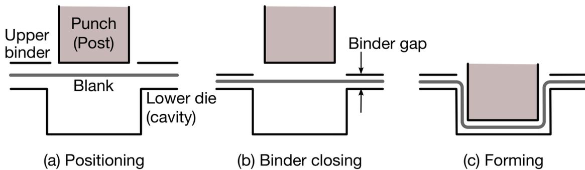
Figure 12-58. IDTEMP = 2: forming in 3-piece toggle draw.
