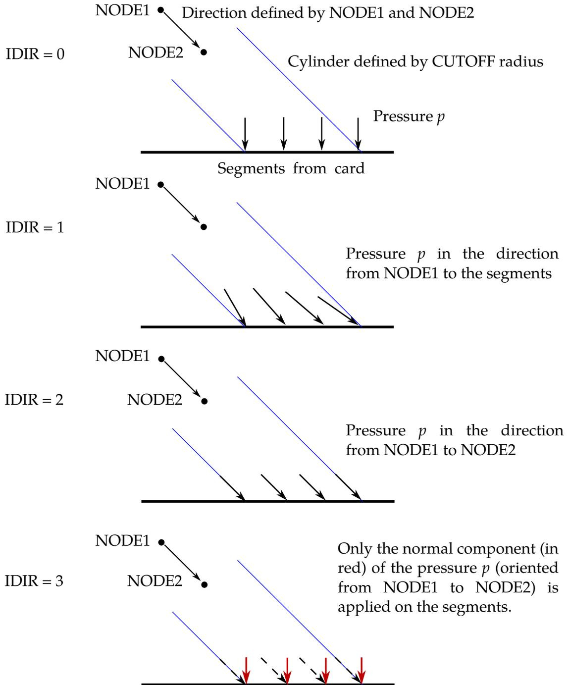
Figure 31-5. Pressure directions for different values of IDIR.
