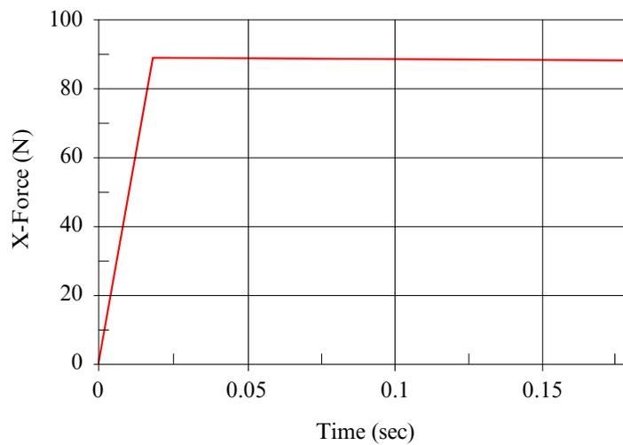
**Figure [17-47].** Pulling force (frictional force) from RCFORC file.
