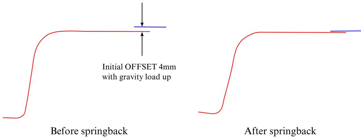
**Figure 12-18.** Springback and contact with nets – gravity up.
