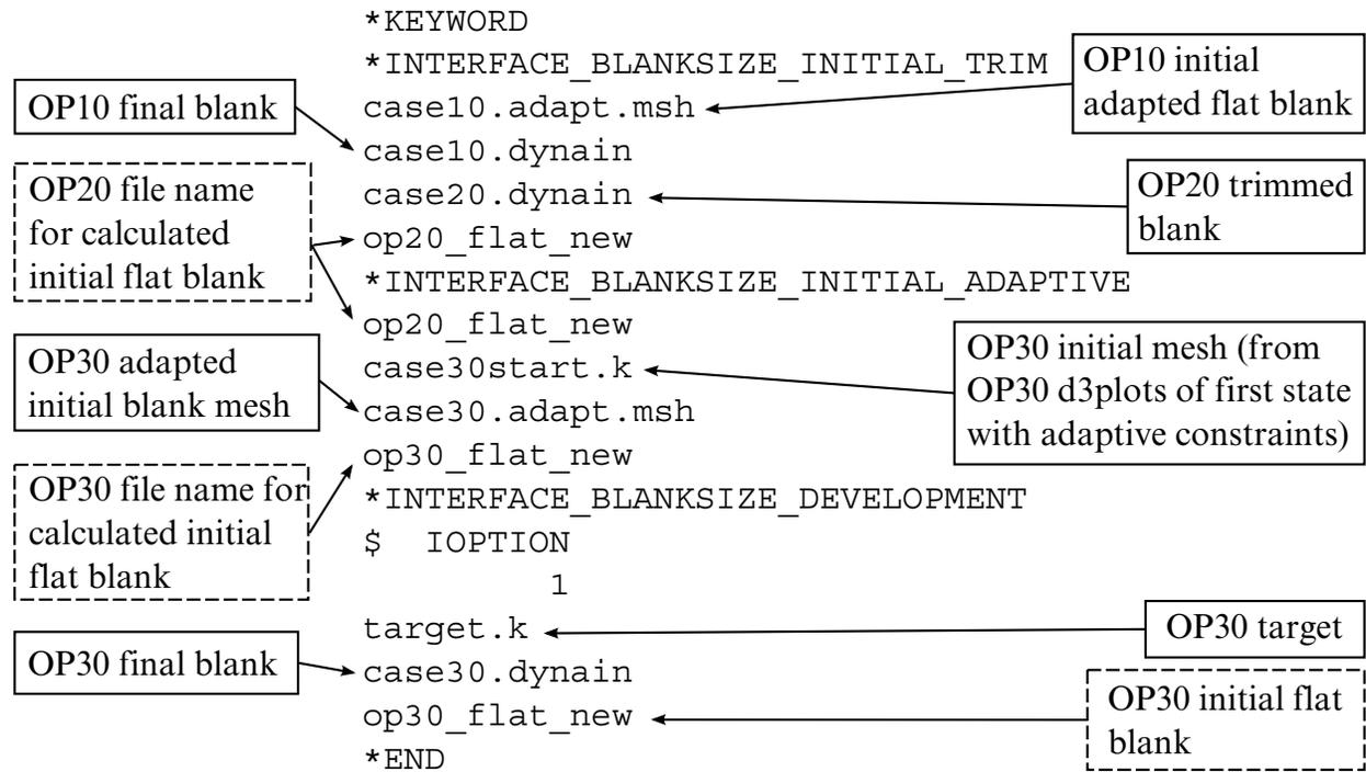
□ User inputs   □□ LS-DYNA intermediate output files
