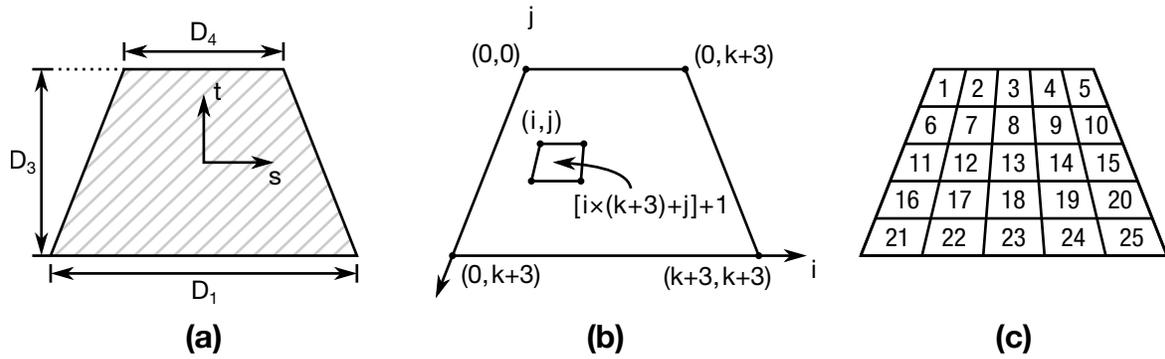
**Figure 28-9.** Type 7: Trapezoidal. (a) Cross section geometry. (b) Integration point numbering. (c) Example for  $k = 2$ .
