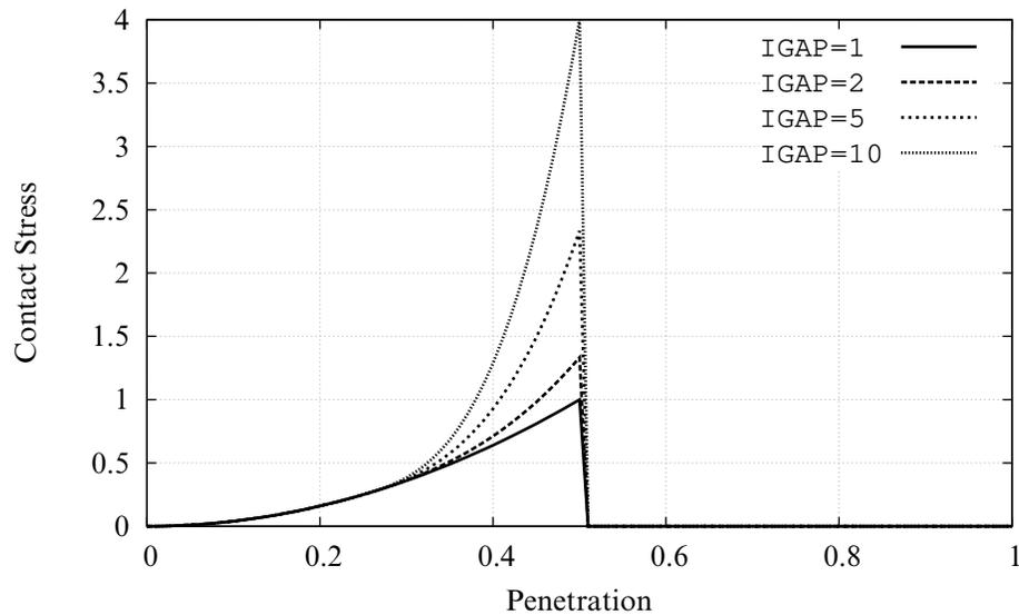
**Figure 11-19.** Mortar contact stress as function of penetration
