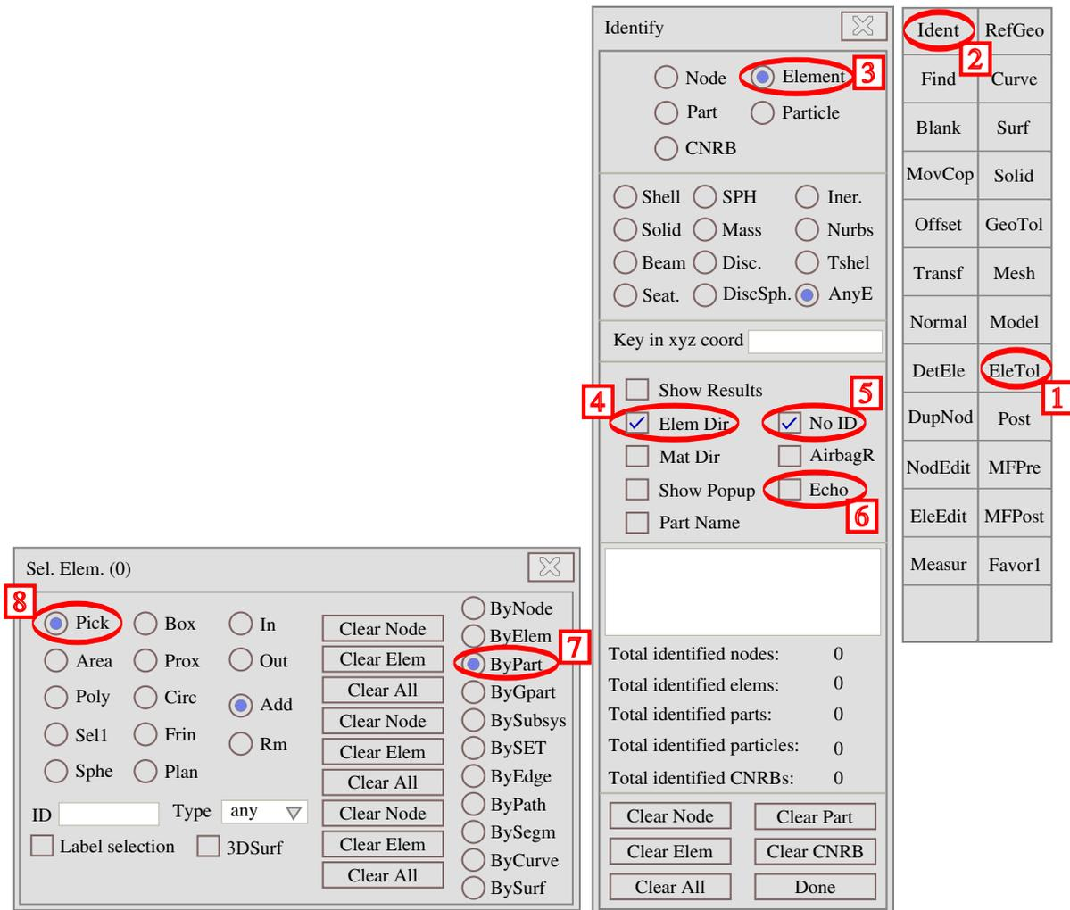
**Figure [17-49].** Checking element directions (N1-N2) by part using LS-PrePost4.0.
