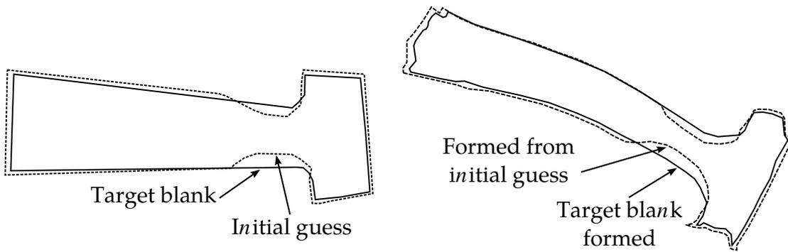
Figure 29-15. Iteration 0 results comparison with target.
