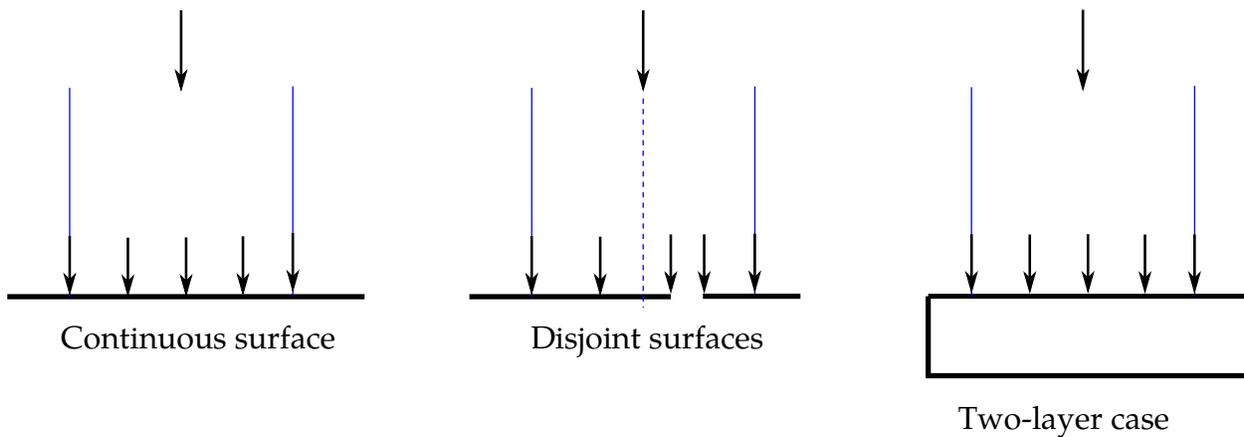
**Figure 31-8.** Applying pressure in SMP/MPP when LSFLG = 1
