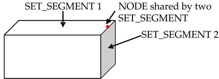
**Figure 23-2.** Nodes with Multiple Boundary Conditions.
