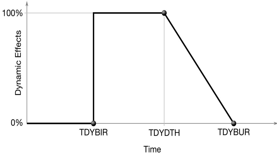
**Figure 12-67.** Birth, death, and burial time for implicit dynamics. The terms involving **M** and **D** are scaled by a factor ranging between 1 and 0 to include or exclude dynamical effects, respectively.
