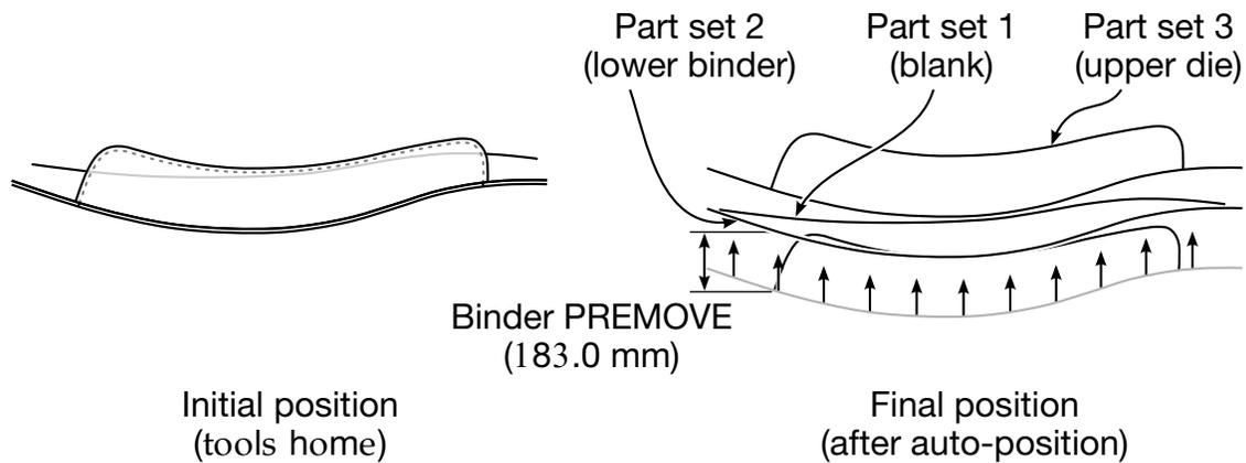
**Figure 12-21.** An example of using the variable REMOVE
