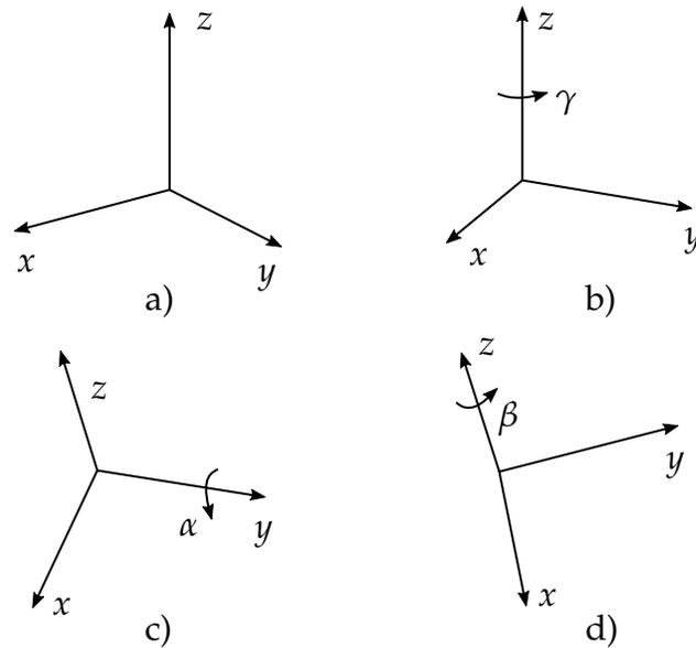
**Figure 10-30.** The angles  $\gamma$ ,  $\alpha$ , and  $\beta$  align rigid body one with rigid body two for the FLEXION-TORSION option, using  $z$ - $y$ - $z$  Euler angles (in the order shown by the figure labels) to calculate the moments. An illustrative version of this figure is shown in [Figure 10-31](#).
