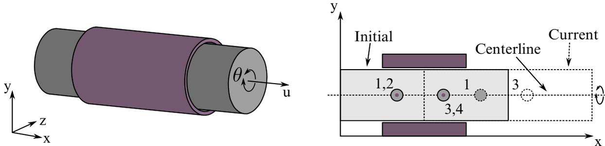
**Figure 10-18.** *Cylindrical Joint.* This joint is derived from the rotational joint by relaxing the constraints along the centerline. This joint admits relative rotation and translation along the centerline.
