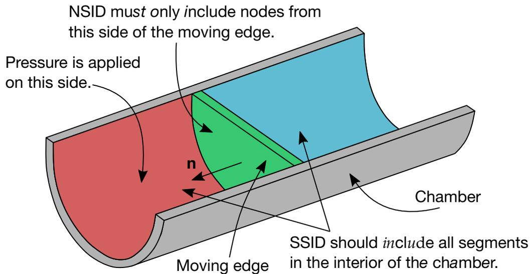
**Figure 31-4.** Schematic view of half a chamber (cut for clarity). Pressure is applied through this keyword to the red region but not the blue region of the chamber. The normal of the moving edge (in green) must point toward the part of the chamber where the pressure is applied.
