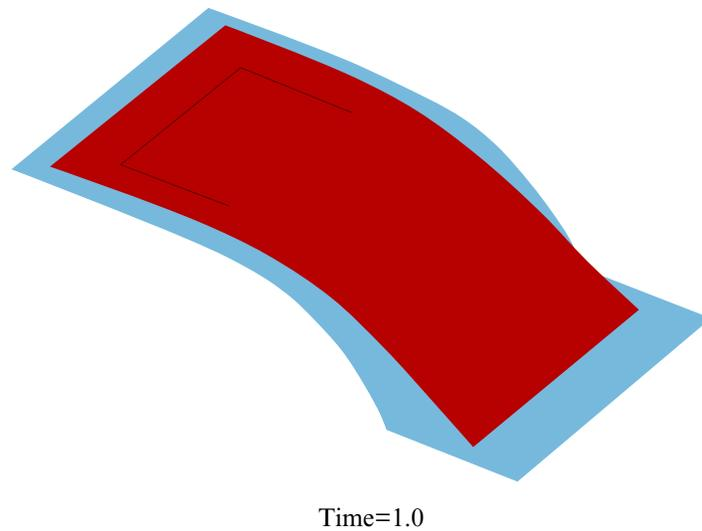
**Figure 12-81.** Gravity loaded blank without the "switching".
