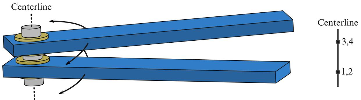
**Figure 10-17.** *Revolute Joint.* Nodes 1 and 2 are coincident; nodes 3 and 4 are coincident. Nodes 1 and 3 belong to rigid body A; nodes 2 and 4 belong to rigid body B. The relative motion of the two rigid bodies is restricted to rotations about the axis formed by the two pairs of coincident nodes. This axis is labeled the “centerline.”
