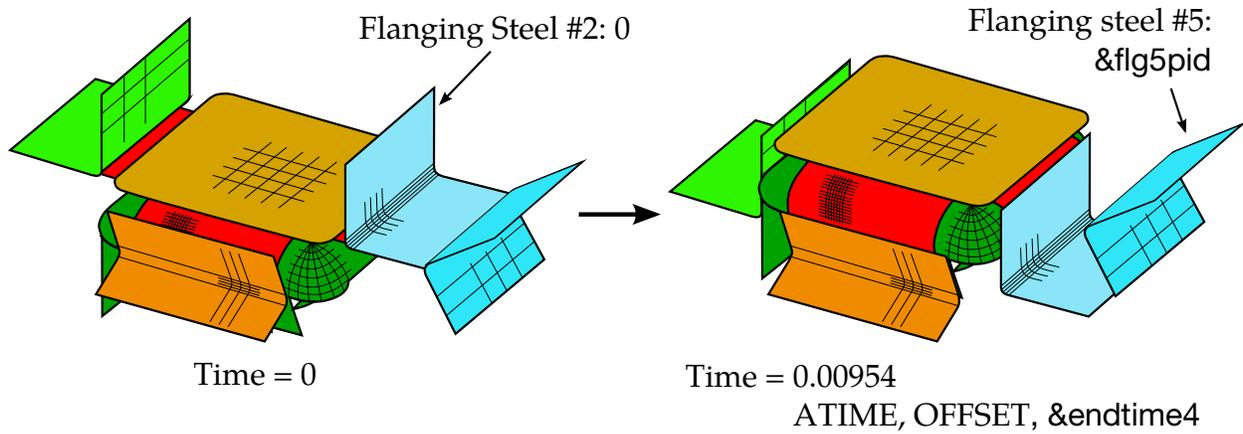
**Figure 11-24.** A sequential flanging process (left); first set of flanging steels reaching home (right).
