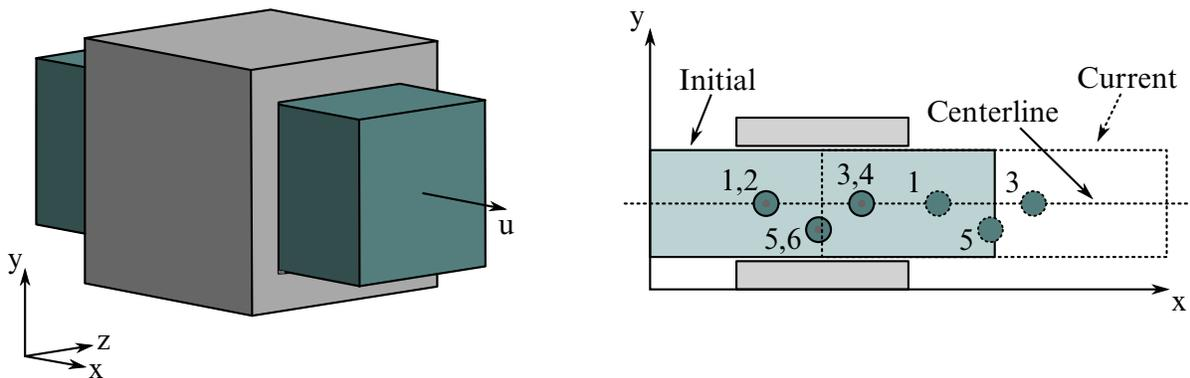
**Figure 10-19.** *Translational joint.* This is a cylindrical joint with a third pair of off-centerline nodes which restrict rotation. Aside from translation along the centerline, the two rigid bodies are stuck together.
