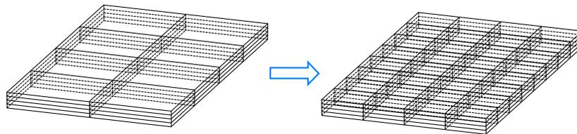
**Figure 12-4.** Mesh fission for sandwich part. Sweeping the top and bottom adaptive shell elements through the thickness, a total of 32 hexahedral elements are refined into 128 of the same type. The number of layers of the solids always remains the same.
