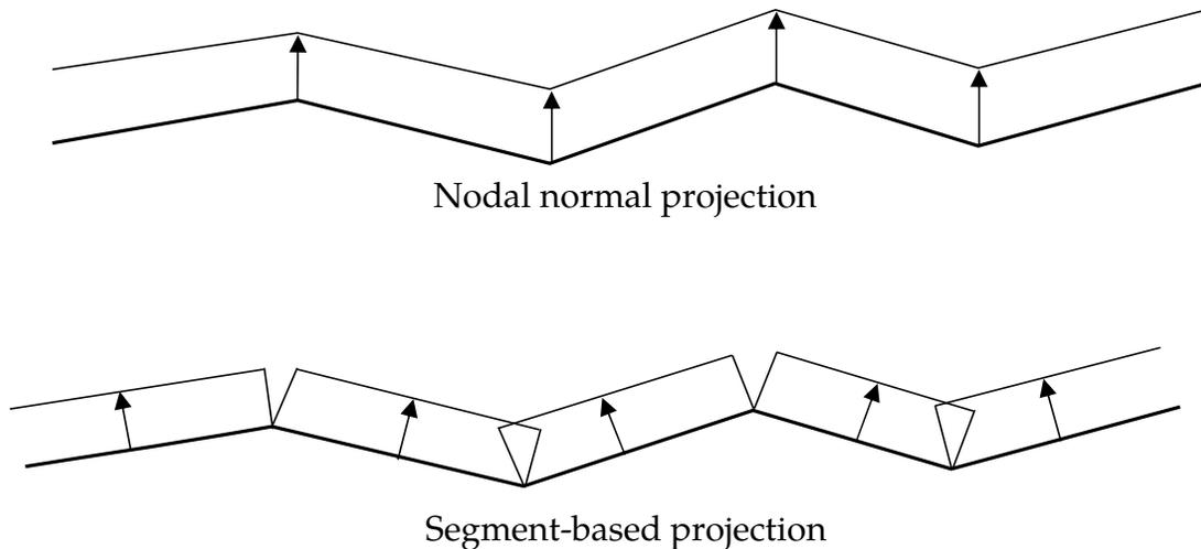
**Figure 11-16.** Nodal normal projection and segment-based projection used in contacts (SMP). MPP contacts use nodal normal projection exclusively.
