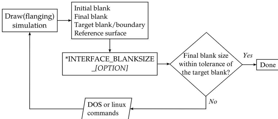
**Figure 29-5.** An iterative blank size development process.
