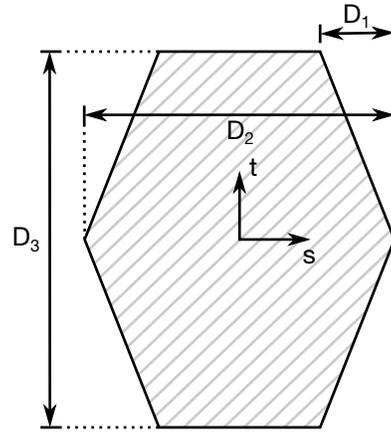
**Figure 39-19.** SECTION\_19  $\Rightarrow$  Box-Shape
