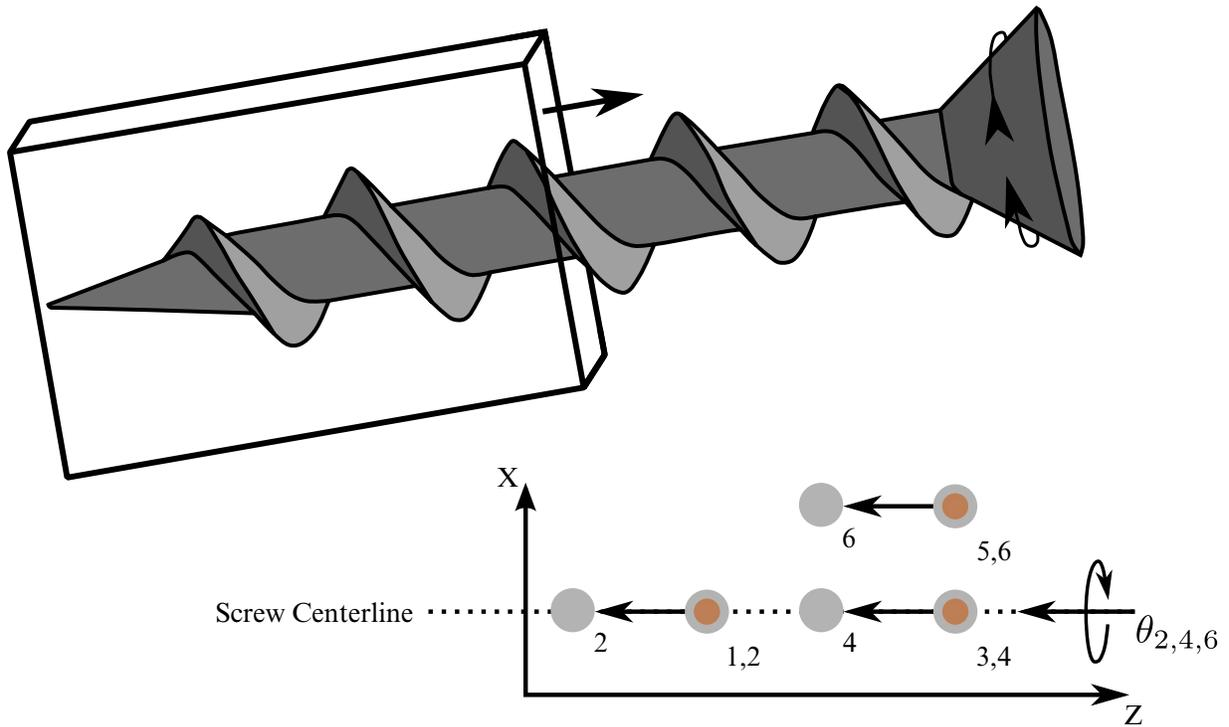
**Figure 10-29.** Screw joint. The second body translates in response to the spin of the first body. Nodal pairs (1, 3) and (2, 4) lie along the same axis and nodal pairs (1, 5) and (2, 6) are orthogonal vectors. The helix ratio,  $\dot{x}/\omega$ , is specified.
