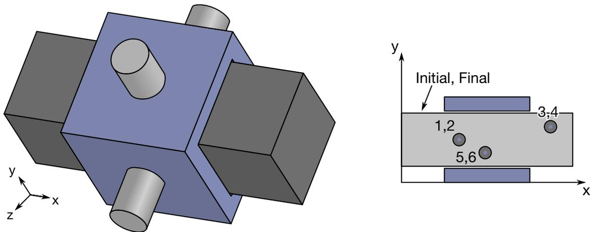
**Figure 10-22.** *Locking Joint.* A locking joint couples two rigid bodies in all six degrees-of-freedom. The forces and moments required to form this coupling are written to the `jntforc` file (\*DATABASE\_JNTFORC). As stated in the Remarks, forces and moments in `jntforc` are calculated halfway between N1 and N3. Nodal pairs (1, 2), (3, 4) and (5, 6) must be coincident. The three spatial points corresponding to three nodal pairs must be neither collocated nor collinear.
