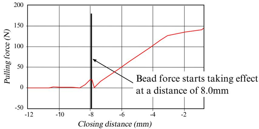
Figure 11-8. Pulling force (NODFOR) as a function of closure distance
