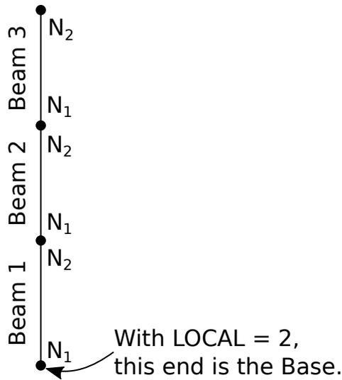
**Figure 10-42.** Example of a beam element topology in a pile. We recommend each beam having the same order for N<sub>1</sub> and N<sub>2</sub>, so that the Base is not ambiguous for LOCAL = 2.
