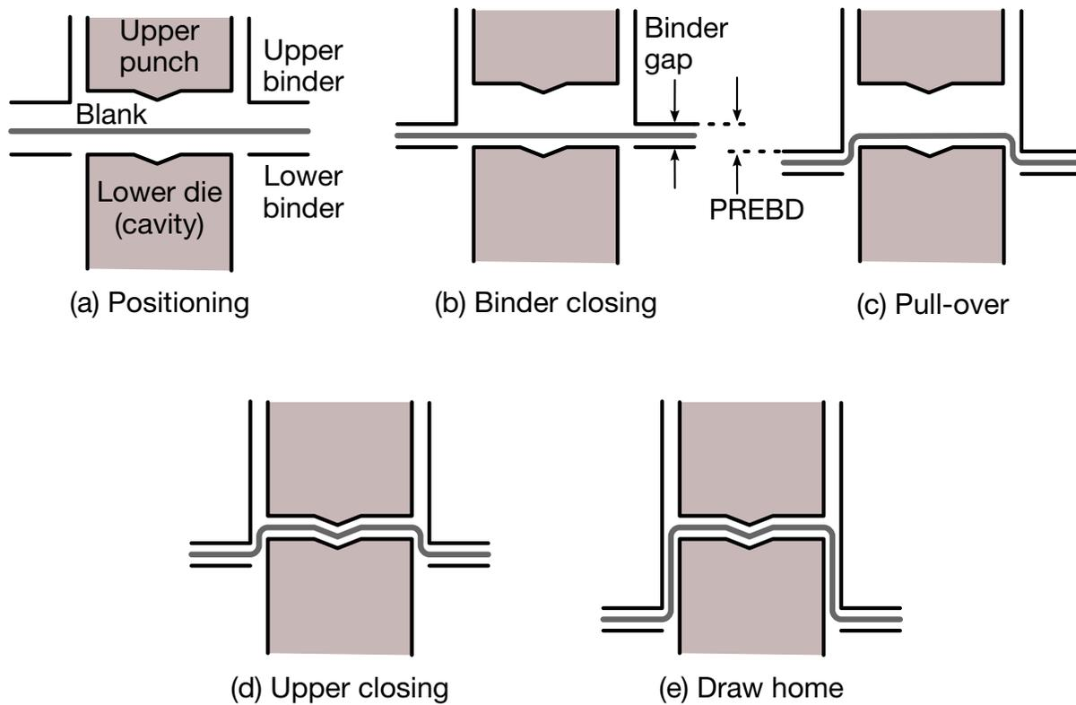
Figure 12-60. IDTEMP = 3: forming in 4-piece stretch draw.
