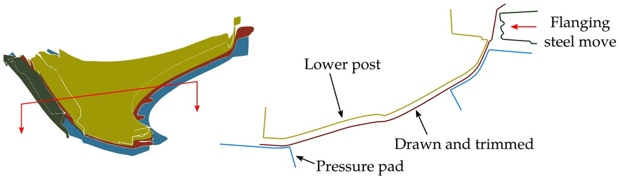
**Figure 29-18.** The flanging process on NUMISHEET 2002 fender outer.
