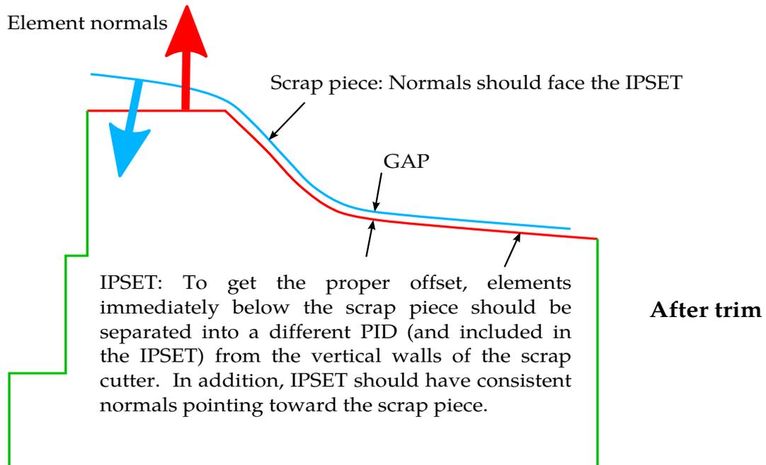
**Figure 12-50.** Element normal of the IPSET in the scrap trimming method.
