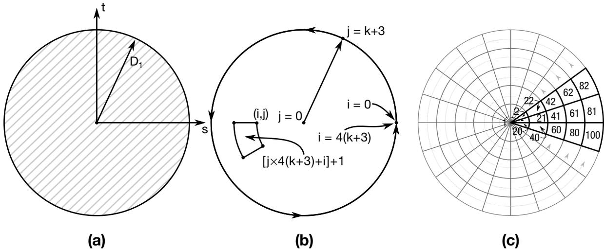
**Figure 28-10.** Type 8: Circular. (a) Cross section geometry. (b) Integration point numbering. (c) Example for  $k = 2$ .
