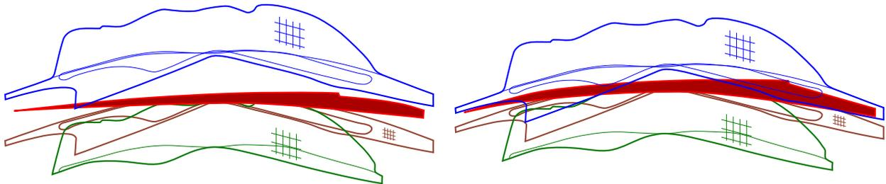
**Figure 11-22.** Upper die move down at  $t = 0.3$  closing the gap (left); continue closing at  $t = 0.743$  (right).
