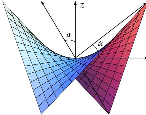
**Figure 12-86.** Illustration of an element in a *W-Mode*. One pair of opposite corners go up, and the other pair goes down. The angle,  $\alpha$ , is formed by the plane of the flat element and by the vector connecting the center to the corner. See [Remark 5](#).
