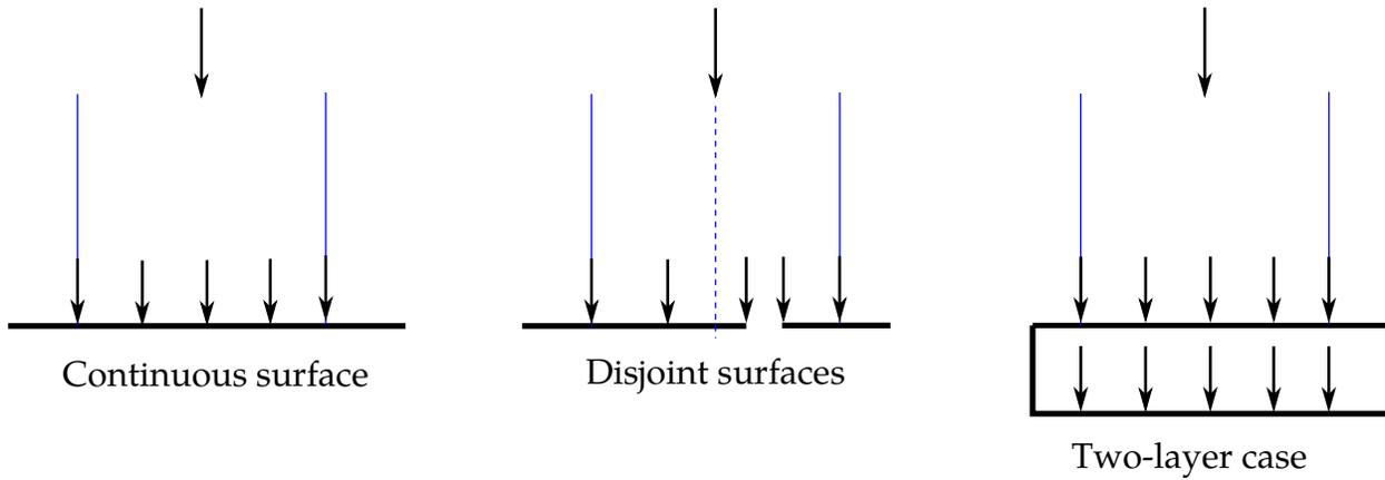
**Figure 31-7.** Applying pressure in MPP when LSFLG = 0
