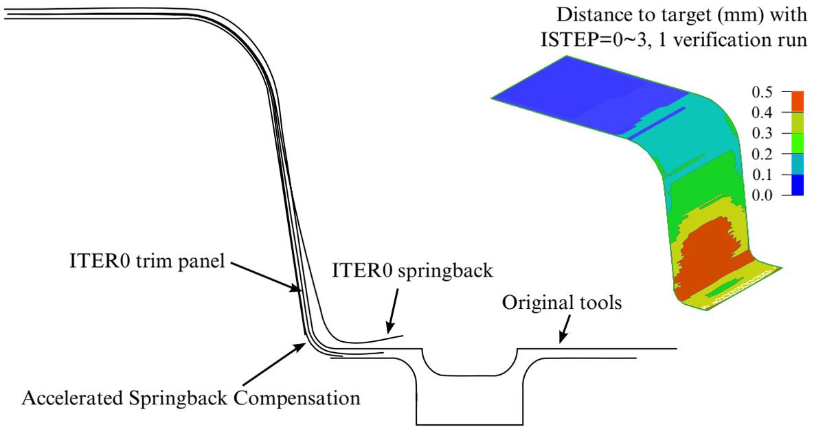
Figure 29-33. Accelerated Springback Compensation.
