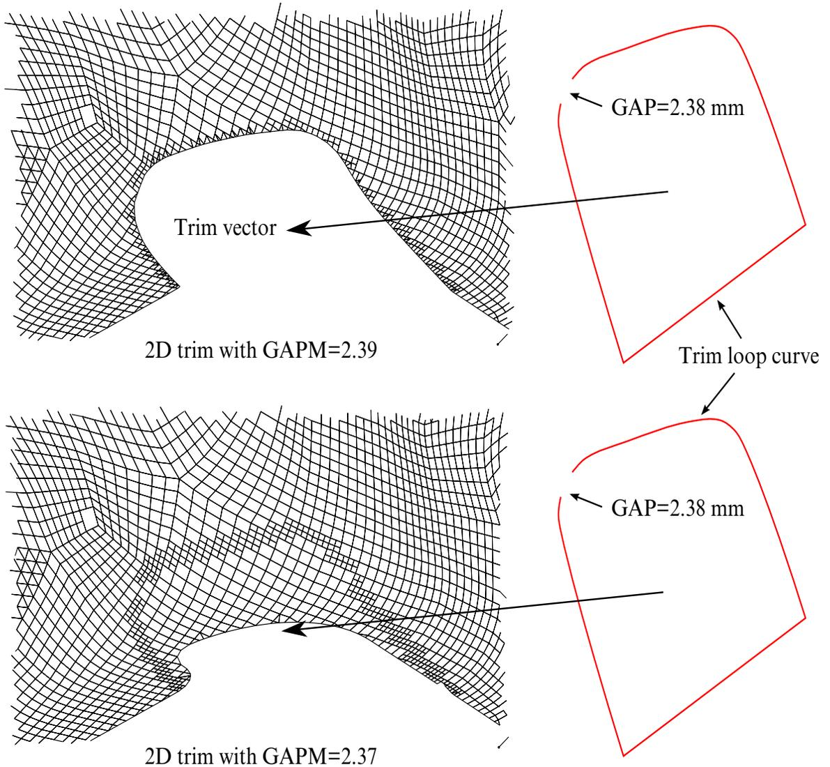
Figure 12-61. A 2D trimming with different GAPM values.
