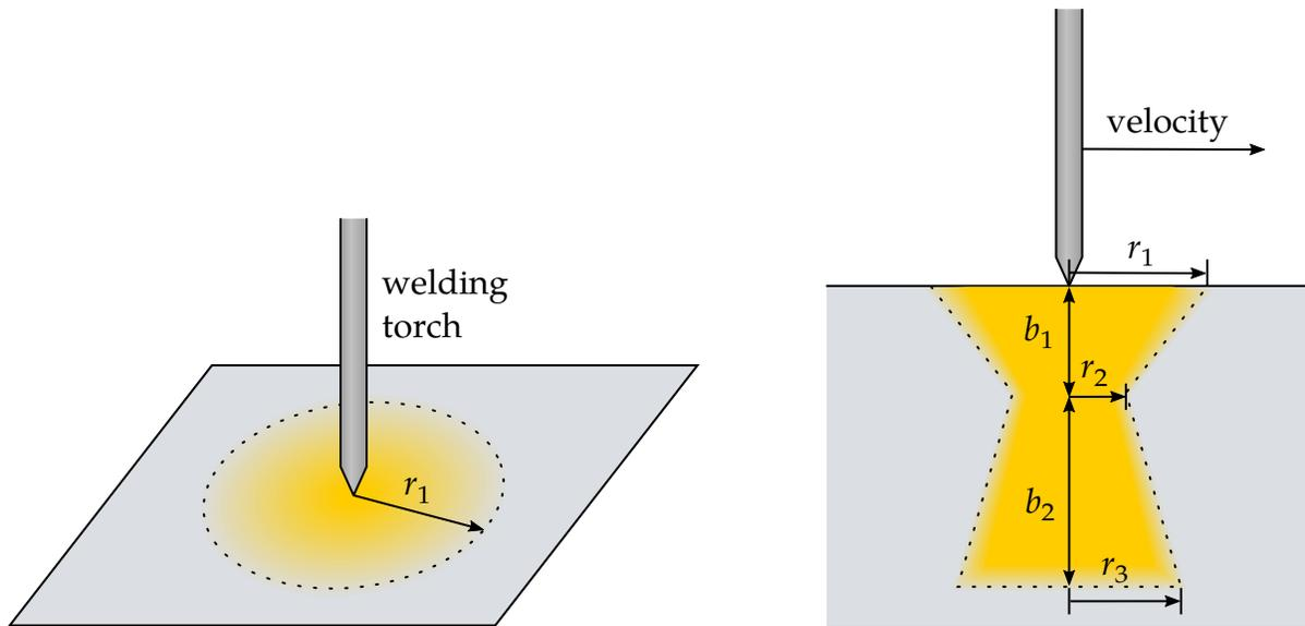
Figure 5-14. Heat source distribution geometry for IFORM = 3
