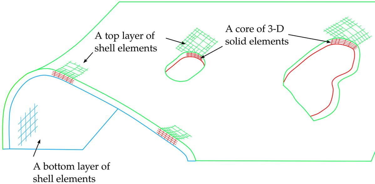
**Figure 12-3.** Activate sandwich composite mesh adaptivity by setting IF-SAND = 1. Before R11.0, adaptivity is limited to only one layer of solid elements; starting with R11.0 adaptive meshing applies to multiple layers of solid elements.
