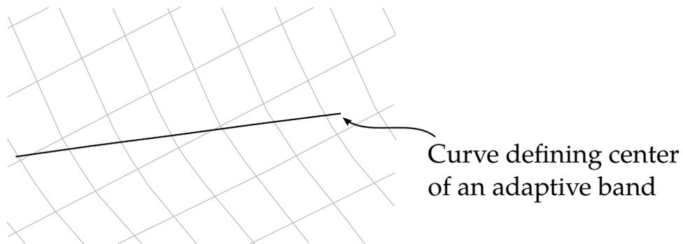
**Figure 12-10.** Original mesh with target curve defined.
