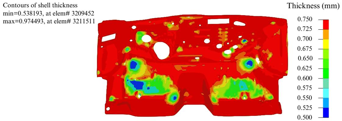
Figure 12-32. Blank thickness with trimmed holes ( $t_0 = 0.75$  mm).
