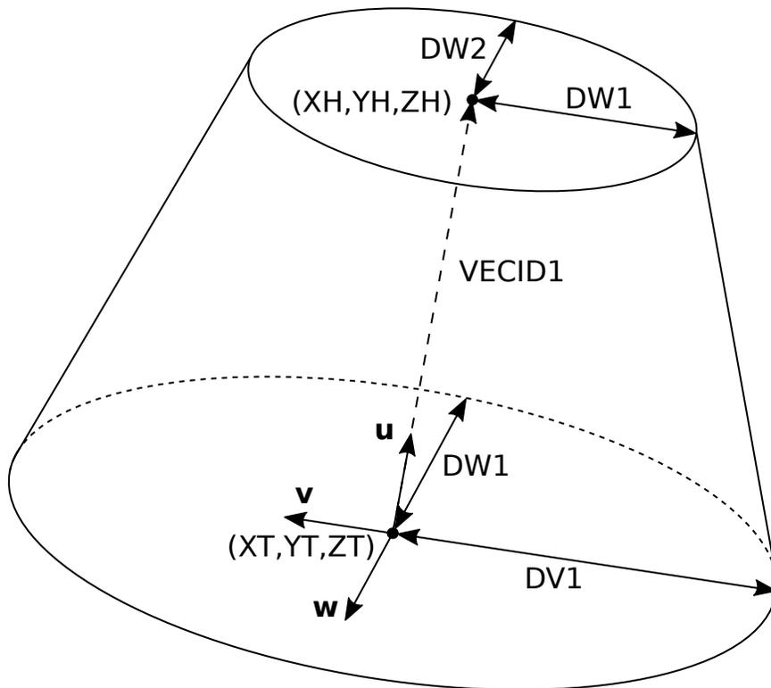
Figure 4-11. Elliptic Truncated Cone (VOLTYP = 2)
