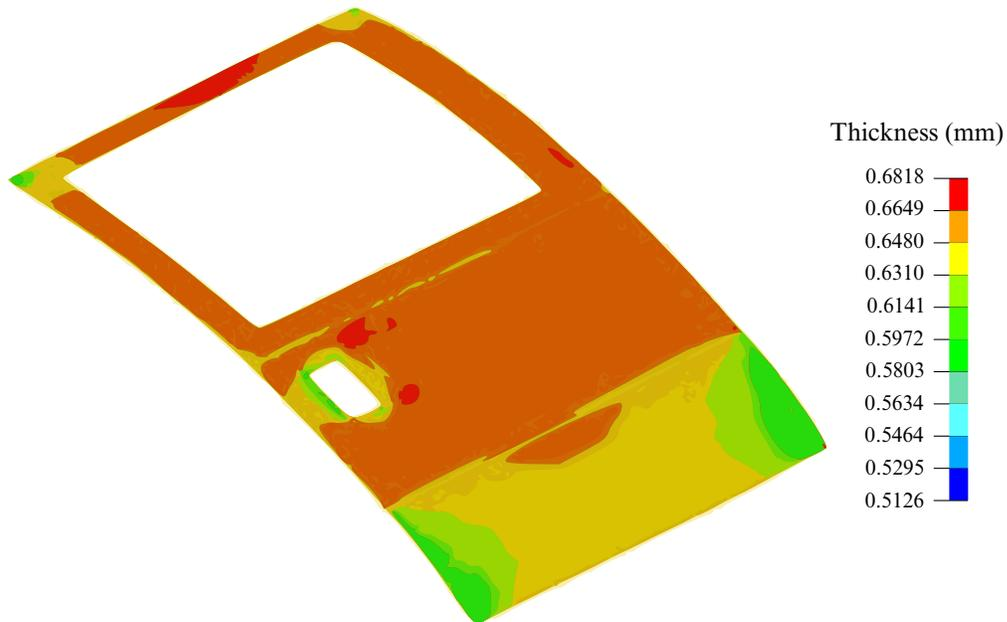
Figure 12-53. Thickness contour of the panel after trimming.
