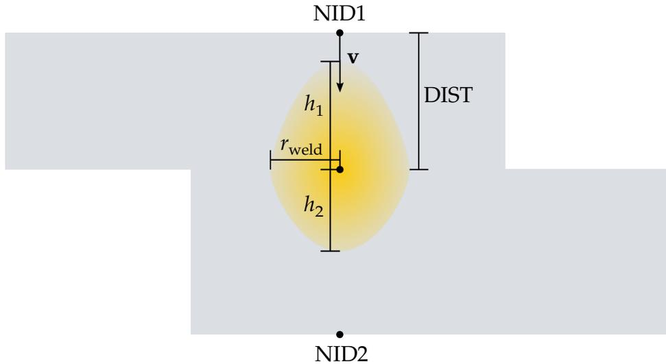
**Figure 5-8.** Example of geometry for OPTION = 0
