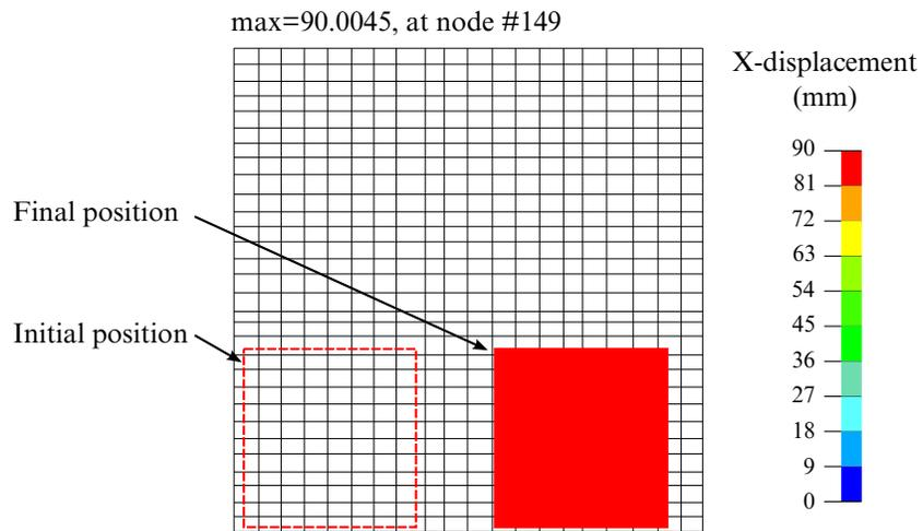
**Figure [17-45].** Initial and final position of the blank.
