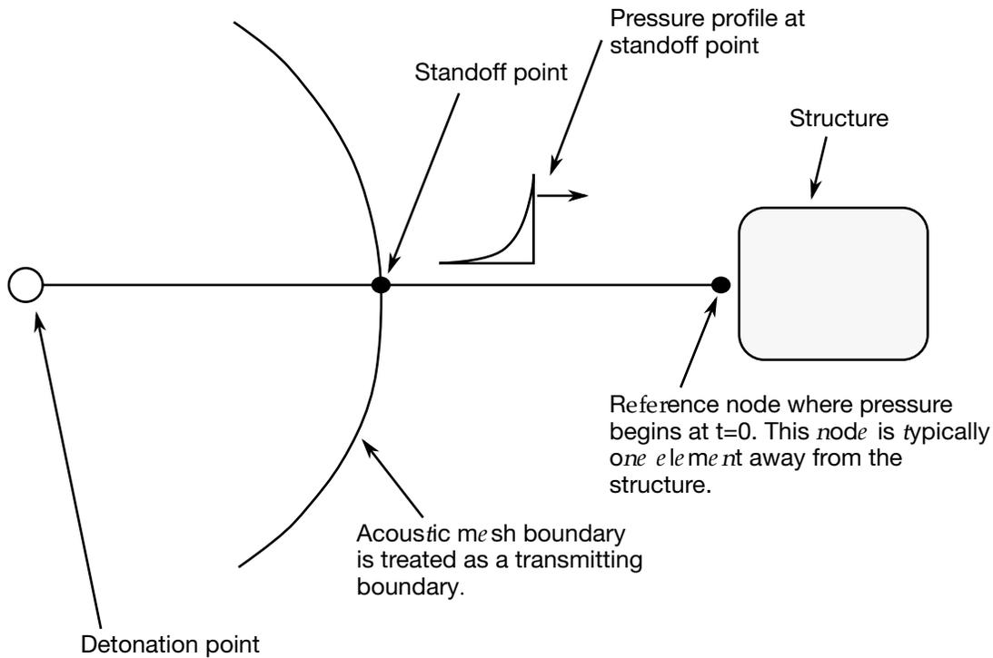
**Figure 27-1.** Initialization of the initial pressures due to an explosive disturbance is performed in the acoustic media. LS-DYNA automatically determines the acoustic mesh boundary and applies the pressure time history to the boundary. This option is only applicable to the acoustic element formulation, see \*SECTION\_SOLID.
