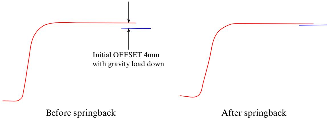
**Figure 12-17.** Springback and contact with nets - gravity down.
