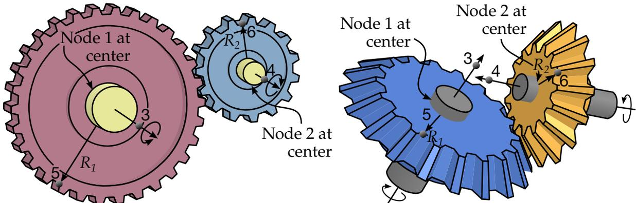
**Figure 10-25.** Gear joints. Nodal pairs (1, 3) and (2, 4) define axes that are orthogonal to the gears. Nodal pairs (1, 5) and (2, 6) define vectors in the plane of the gears. The ratio  $R_2/R_1$  is specified but need not necessarily correspond to the geometry, if for instance the gear consists of spiral grooves. Note that the gear joint in itself does not maintain the contact point but this requires additional treatment, such as accompanying it with other joints.
