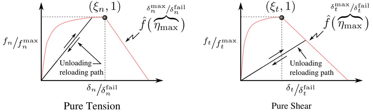
**Figure 10-53.** Force response of self penetrating rivet.
