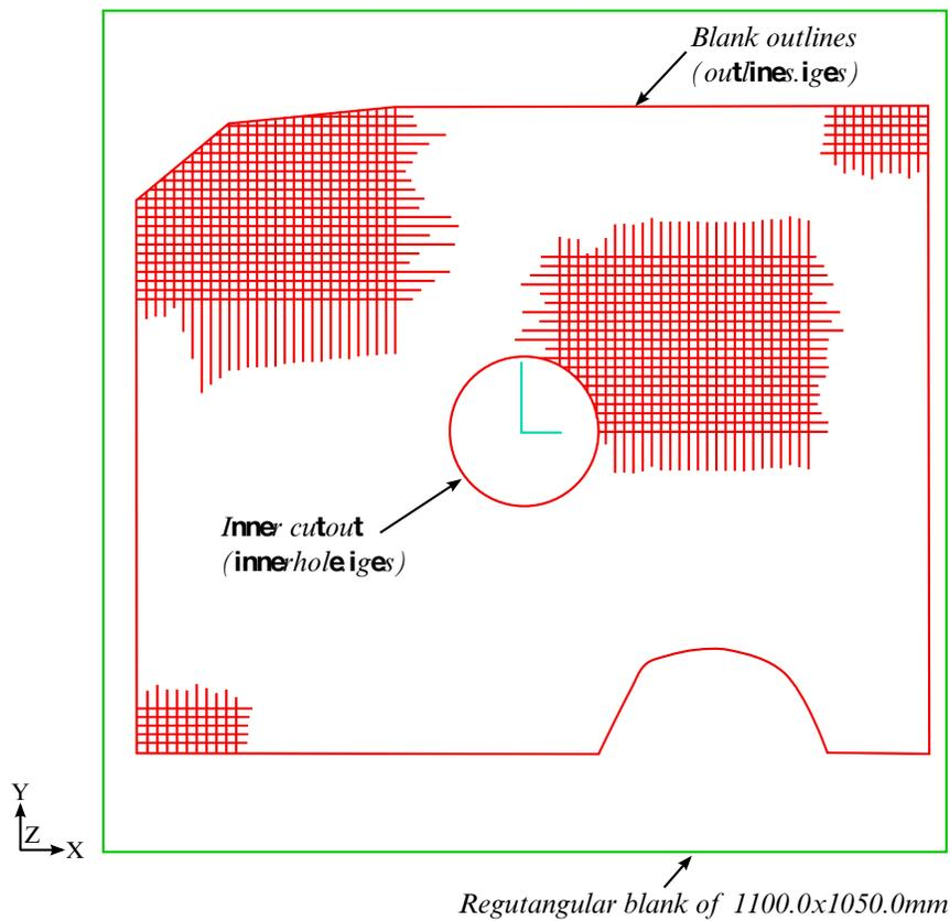
**Figure 17-40.** A rectangular blank mesh is generated and trimmed into a developed blank shape, with an inner cutout defined by *innerhole.iges* and outline defined by *outlines.iges*.
