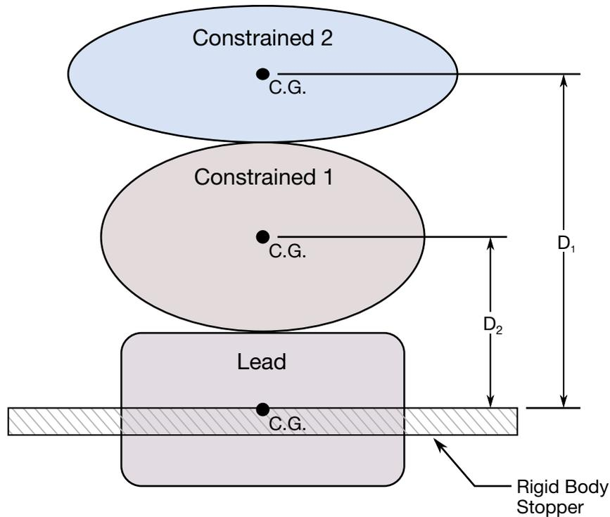
**Figure 10-40.** When the lead rigid body reaches the rigid body stopper, the velocity component into the stopper is set to zero. Constrained rigid bodies 1 and 2 also stop if the distance between their mass centers and the lead rigid body is less than or equal to the input values  $D_1$  and  $D_2$ , respectively.
