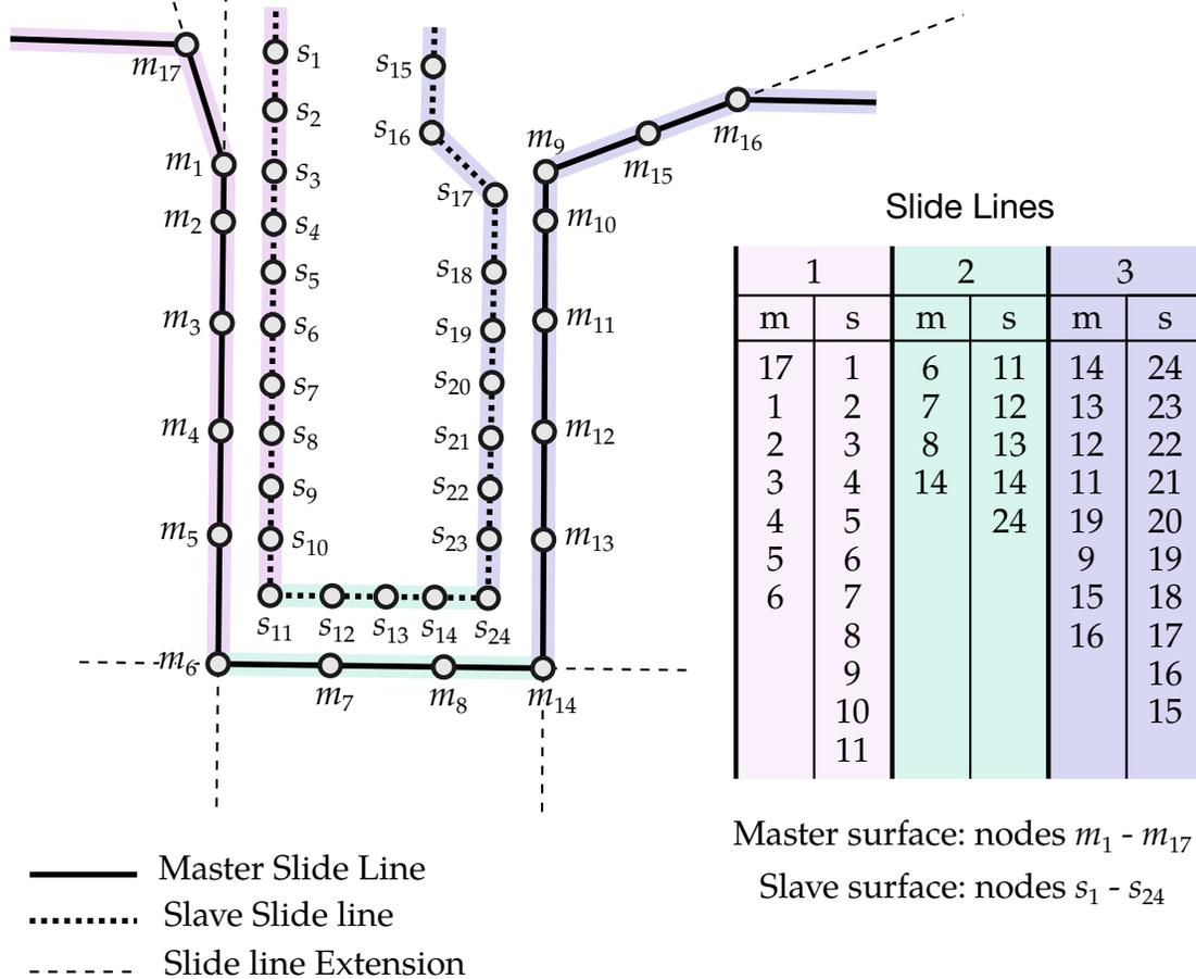
**Figure 11-27. Slide line Example.** Note: (1) as recommend, for 90° angles each facet is assigned a distinct slide line; (2) the master slide line is more coarsely meshed; (3) the slave is to the left of the master (following the node ordering, see inset table); (4) as shown for slave nodes 1 and 2 it is important the slide line extension does not spuriously come into contact.
