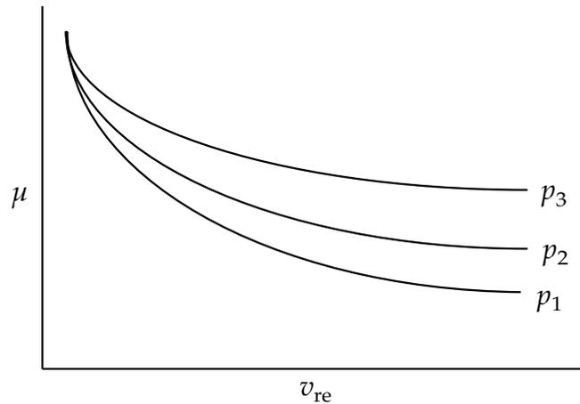
**Figure 11-1.** Friction coefficient,  $\mu$ , can be a function of relative velocity and pressure. See [Remark 1](#) for FS = 2.0.
