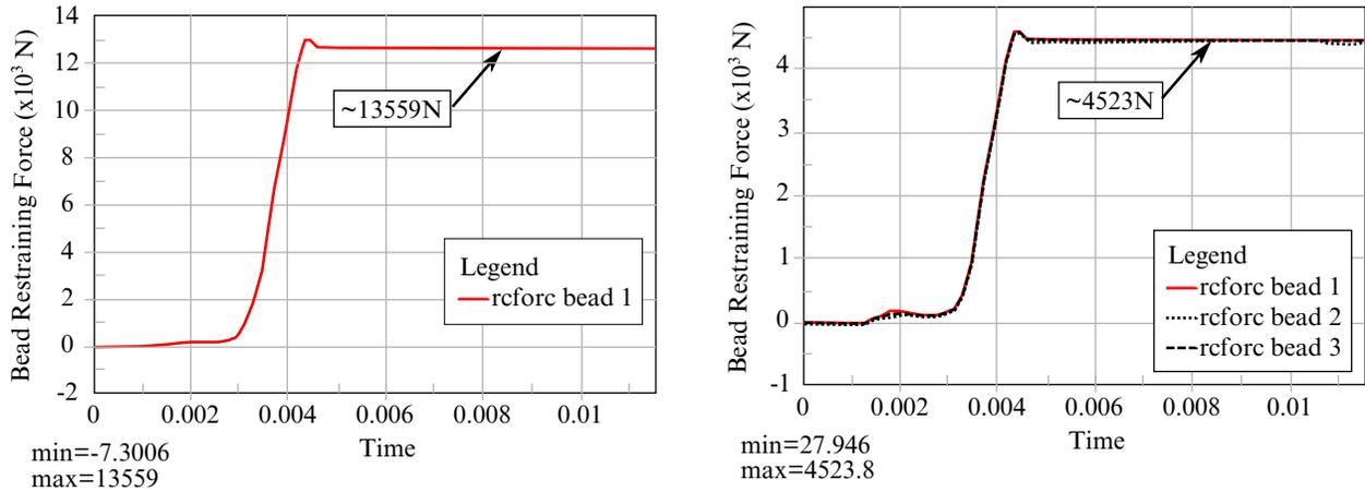
Figure 11-5. Bead force verification between NBEAD = 1 (left) and 3
