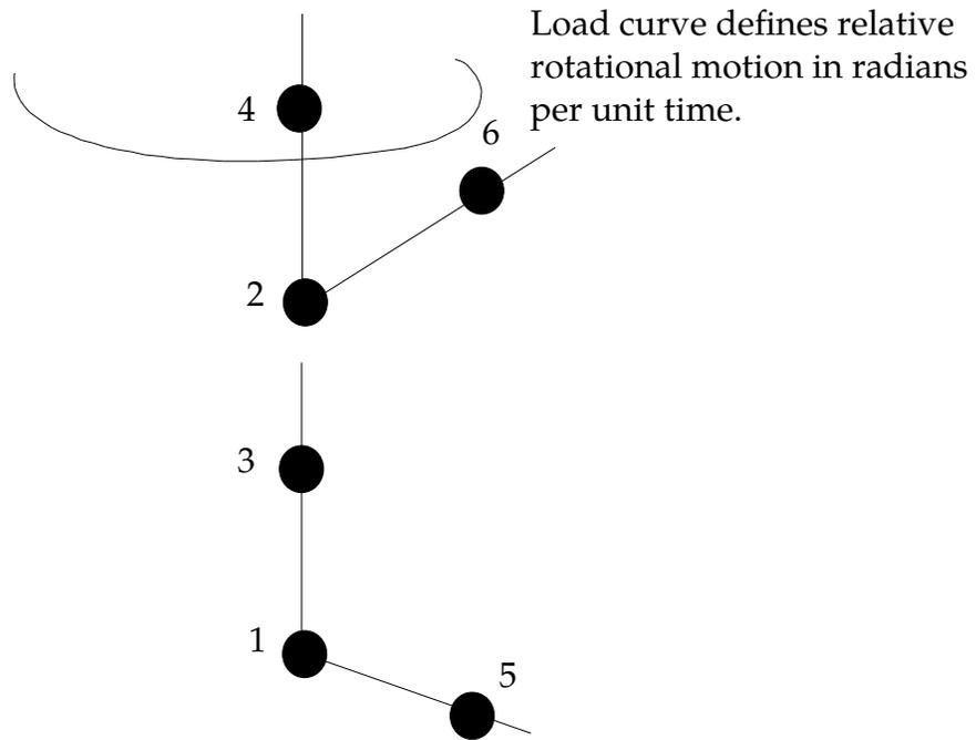
**Figure 10-24.** Rotational motor joint. This joint can be used in combination with other joints such as the revolute or cylindrical joints.
