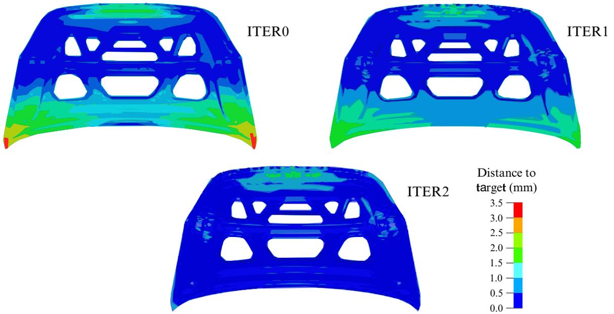
Figure 29-32. Iterative compensation for a localized (backlite) region.
