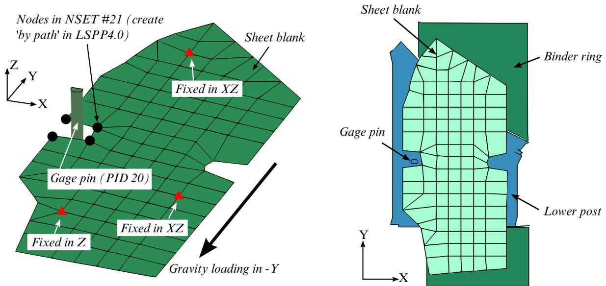
Figure 11-13. Illustrative/test model for SOFT=6 (left) and initial blank position.
