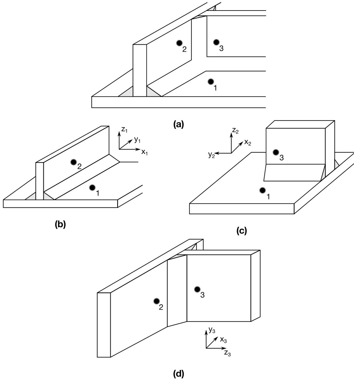
**Figure 10-10.** A simple cross fillet weld illustrates the required input. Here  $NPR = 3$  with nodal pairs  $(A = 2, B = 1)$ ,  $(A = 3, B = 1)$ , and  $(A = 3, B = 2)$ . The local coordinate axes are shown. These axes are fixed in the rigid body and are referenced to the local rigid body coordinate system which tracks the rigid body rotation.
