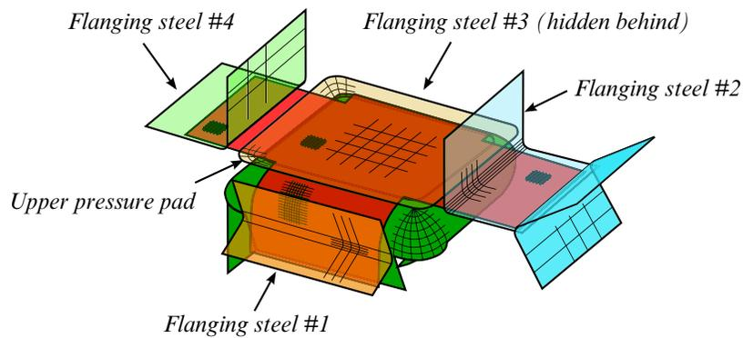
**Figure 12-37.** An example of multiple flanging process.
