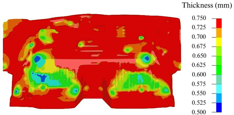
**Figure 12-27.** Shell thickness prediction ( $t_0 = 0.75$  mm).
