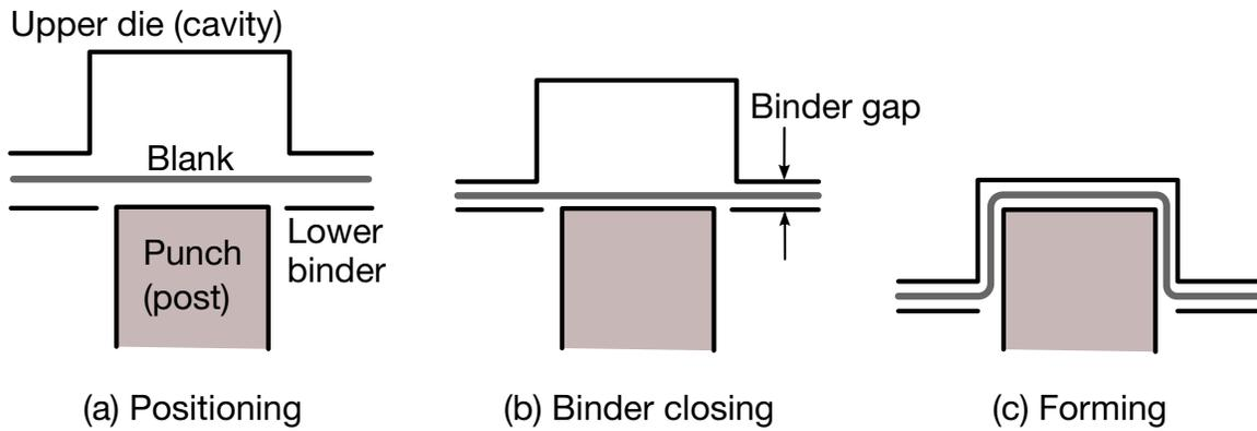
Figure 12-57. IDTEMP = 1: forming in 3-piece air draw.
