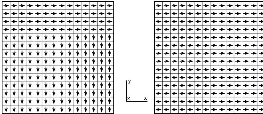
**Figure [17-48].** Element directions (N1-N2) of an incoming sheet blank (left) and directions after re-orientation.
