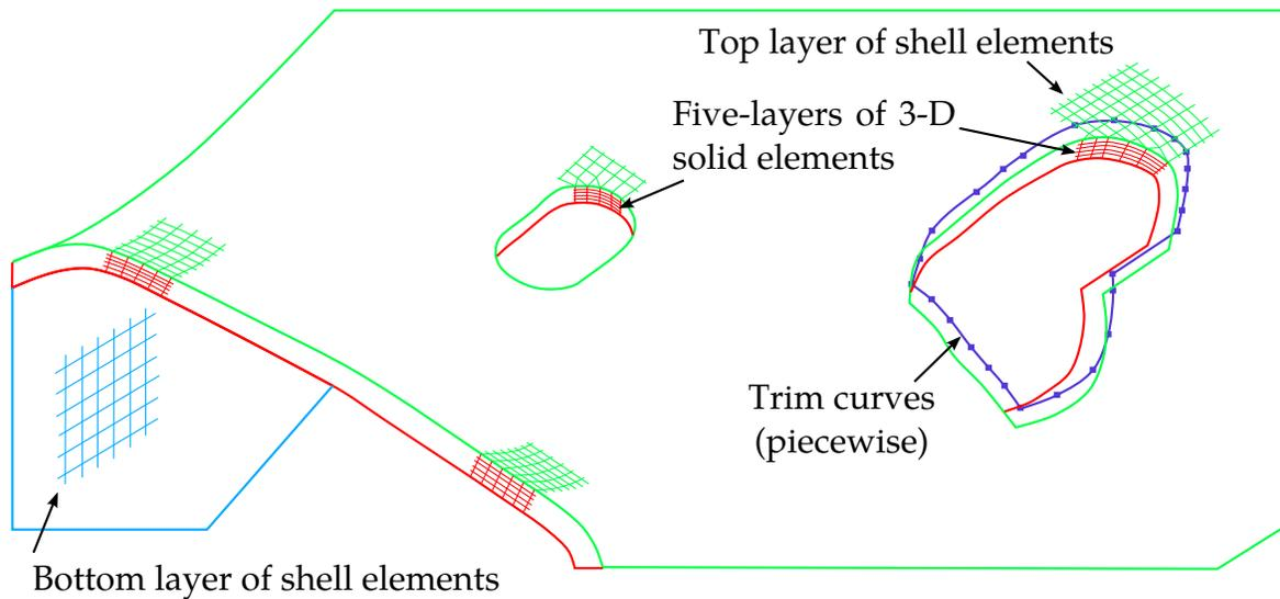
**Figure 17-31.** 3D trimming of laminates (a core of multiple-layers of solid elements with top and bottom layers of shell elements) using \*DEFINE\_CURVE\_TRIM\_3D. Note that shell elements must share the same nodes with the solid elements at the top and bottom layer.
