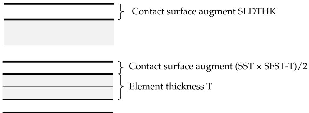
**Figure 11-18.** Illustration of contact surface location for automatic Mortar contact, solids on top and shells below.
