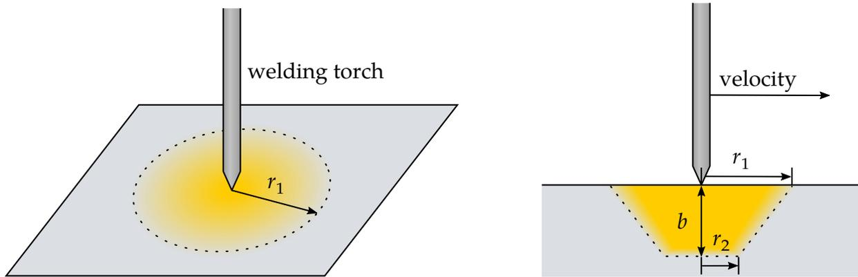
**Figure 5-15.** Heat source distribution geometry for IFORM = 4
