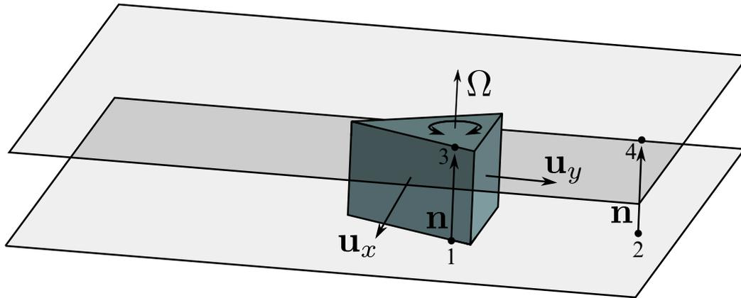
**Figure 10-20.** *Planar joint.* This joint is derived from the rotational joint by relaxing the constraints normal to the centerline. Relative displacements along the direction of the centerline are excluded.
