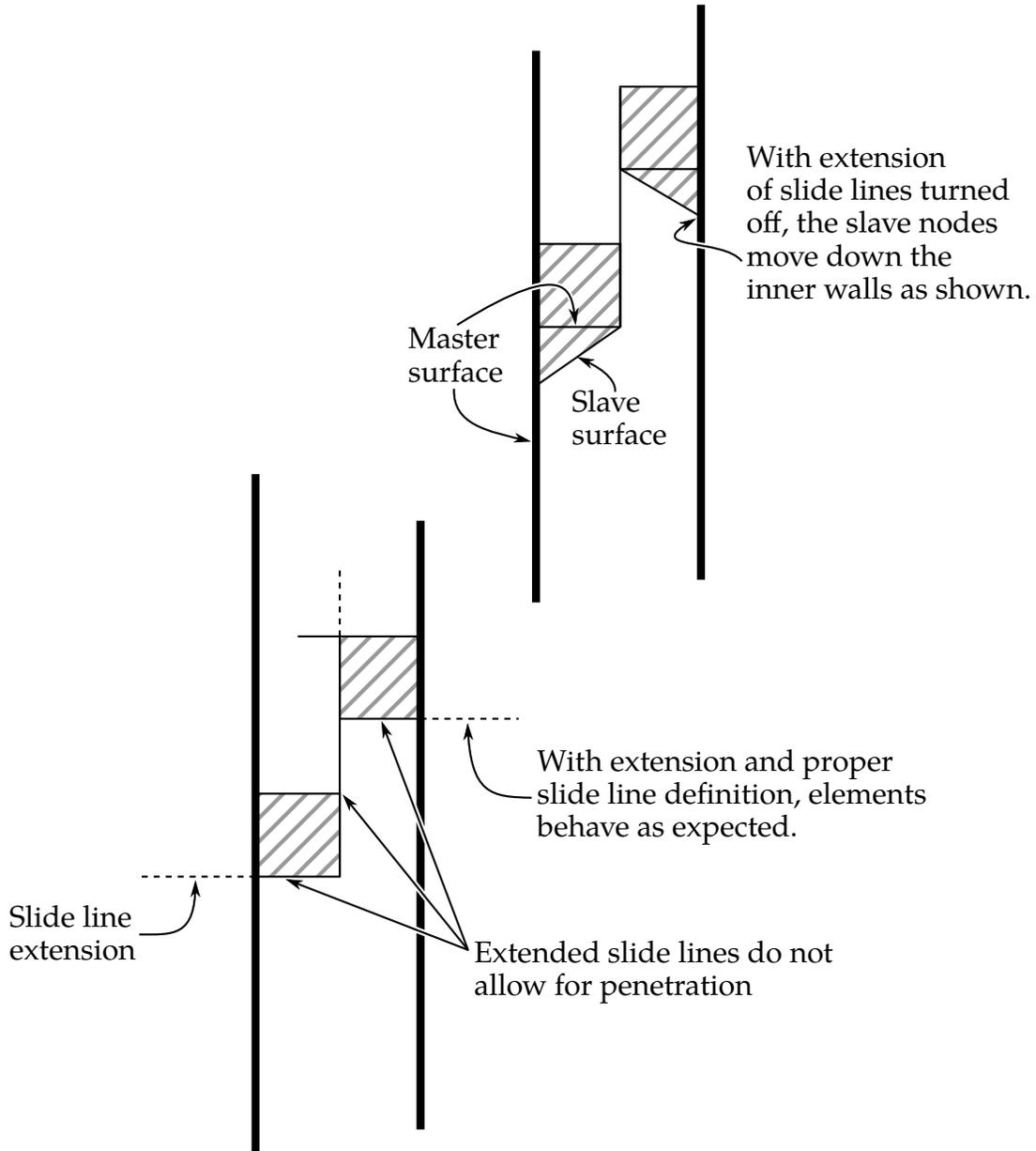
**Figure 11-28.** *With and without extension.* Extensions may be turned off by setting EXT\_PAS (card 2), but, when turned off, slave nodes may “leak” out as shown in the upper version of the figure.
