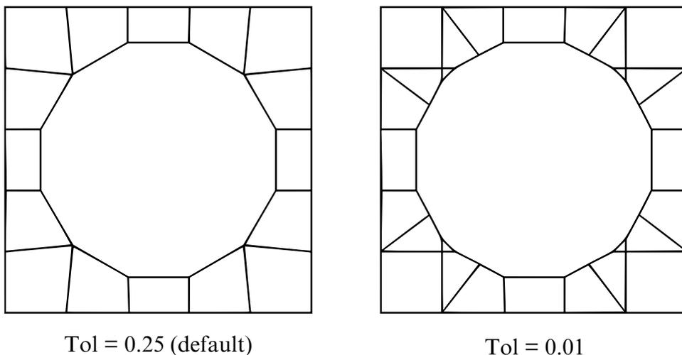
**Figure 17-24.** Trimming Tolerance. The tolerance limits the size of the small elements generated during trimming. The default tolerance (left) produces large elements. Using a tolerance of 0.01 (right) allows smaller elements and more detail in the trim line.
