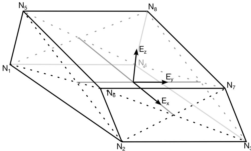
**Figure 10-36.** The  $E_x$  direction is aligned along the line segment connecting the centers of the 2-3-6-7 and the 1-4-8-5 faces. The  $E_y$  direction is orthogonal to the  $E_x$  direction and in the plane containing both  $E_x$  and the segment connecting the centers of the 1-2-6-5 and 3-4-8-7 faces. The  $E_z$  is normal to this plane.
