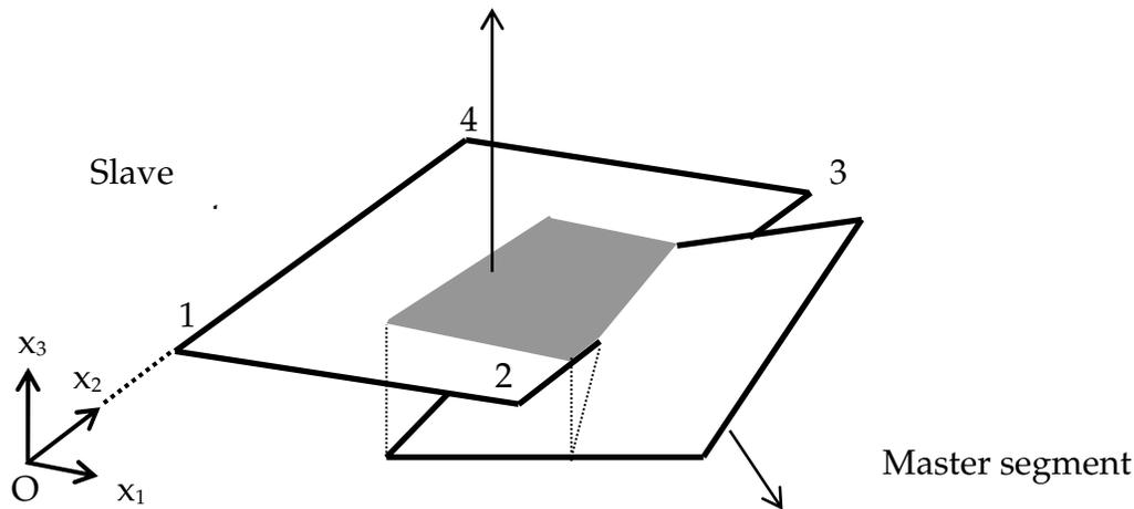
**Figure 11-17.** Illustration of Mortar segment to segment contact
