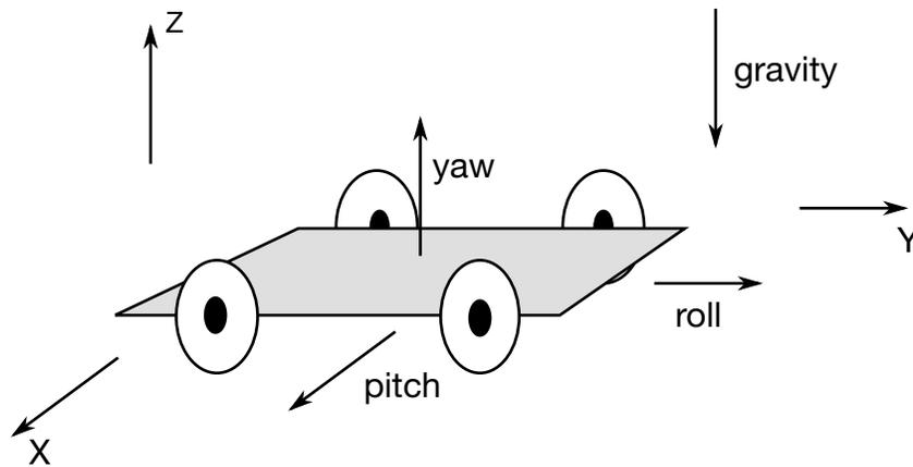
**Figure 27-3.** The vehicle pictured is to be oriented with a successive rotation sequence about the yaw, pitch, and roll axes, respectively. Accordingly, AAXIS = 3, BAXIS = 1, and CAXIS = 2. The direction of gravity is given by GRAV = -3.
