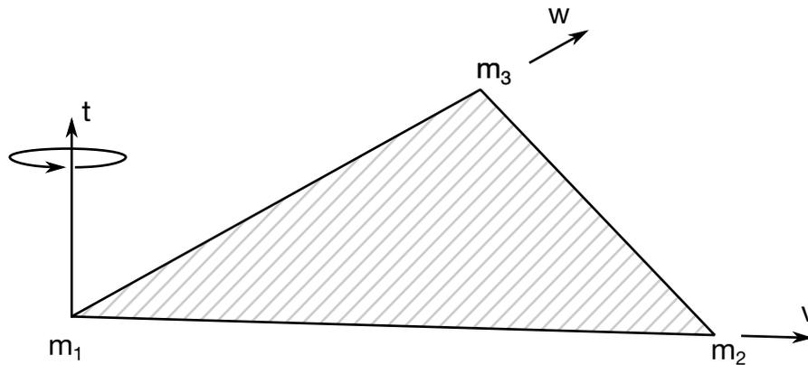
**Figure 31-9.** Nodes M1, M2, and M3 define a plane. A positive follower force acts in the positive  $t$ -direction of that plane, that is, along the normal vector of the plane. A positive follower moment puts a counterclockwise torque about the normal vector. The normal vector is found by the cross product  $\mathbf{t} = \mathbf{v} \times \mathbf{w}$  where  $\mathbf{v}$  and  $\mathbf{w}$  are vectors as shown.
