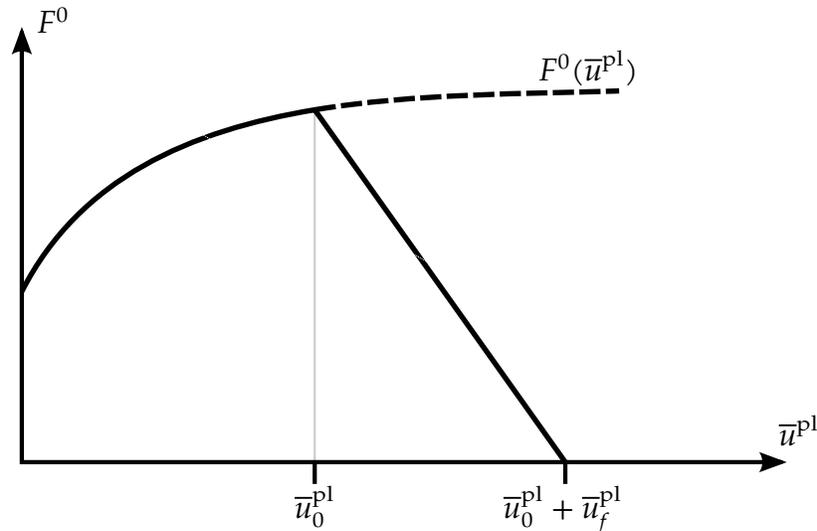
**Figure 10-14.** Force-displacement curve: plasticity and linear damage
