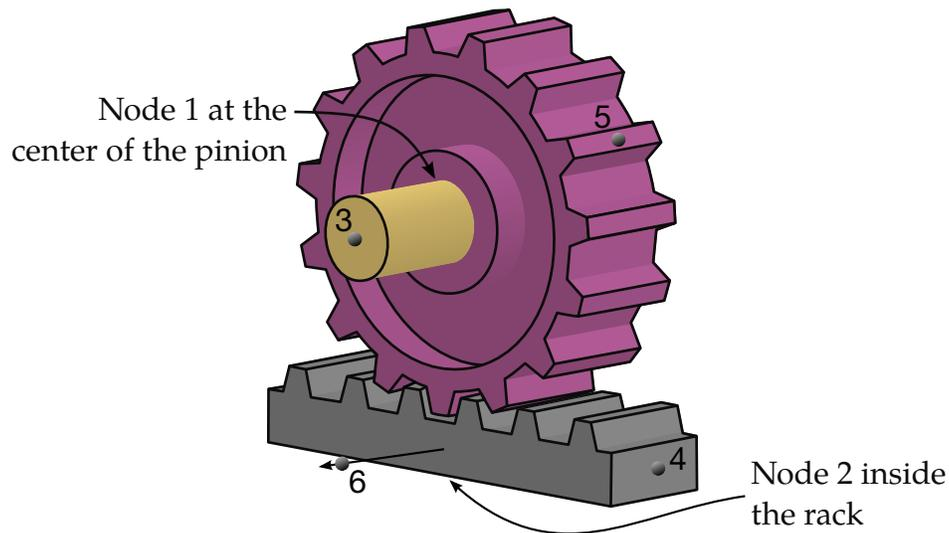
**Figure 10-26.** Rack and pinion joint. Nodal pair (1, 3) defines the axis of rotation of the first body (the pinion). Nodal pair (1, 5) is a vector in the plane of the pinion and is orthogonal to nodal pair (1, 3). Nodal pair (2, 4) defines the direction of travel for the second body (the rack). Nodal pair (2, 6) is parallel to the axis of the pinion and is thus parallel to nodal pair (1, 3). The value  $h$  is specified. The velocity of the rack is  $h\omega_{\text{pinion}}$ .
