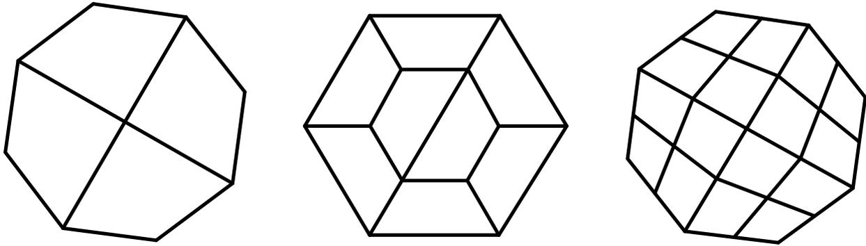
**Figure 17-51.** Illustration of four, eight, and sixteen element assemblies of solid hexahedron elements forming a single spot weld.
