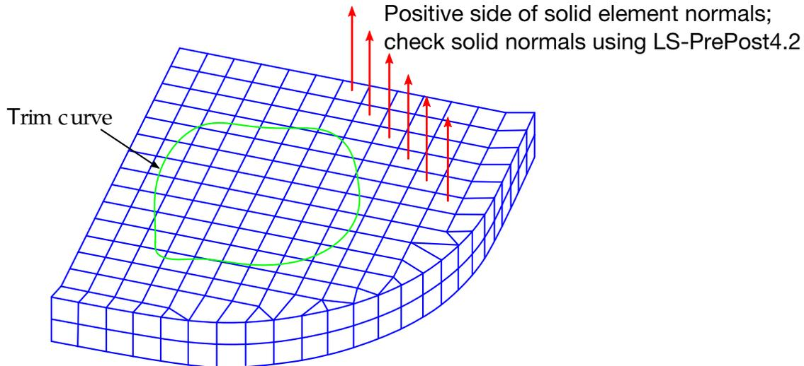
All solid element normals must be consistent. If trim curve is close to the positive normal side, set TDIR=1; otherwise set TDIR=-1. Respacing the curve with more points, project the respaced curve to the top or bottom solid surface may help the trimming.
