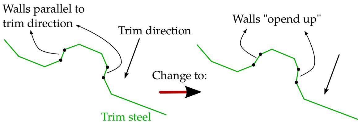
**Figure 12-49.** Walls that are parallel to trim direction anywhere in a trim steel (left) are not allowed. Wall needs to be opened up in relation to the trim direction for a successful simulation (right).
