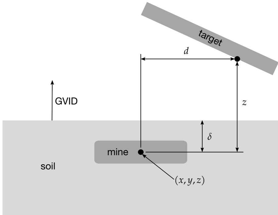
Figure 27-2. Schematic of the buried mine parameters.
