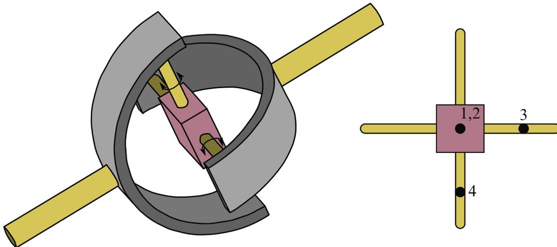
**Figure 10-21.** *Universal Joint.* Nodes 1 and 2 are initially coincident. The segments formed by nodal pairs (1, 3) and (2, 4) must be orthogonal; they serve as axes about which the two bodies may undergo relative rotation. The universal joint excludes all other relative motion and the axes remain orthogonal at all time.
