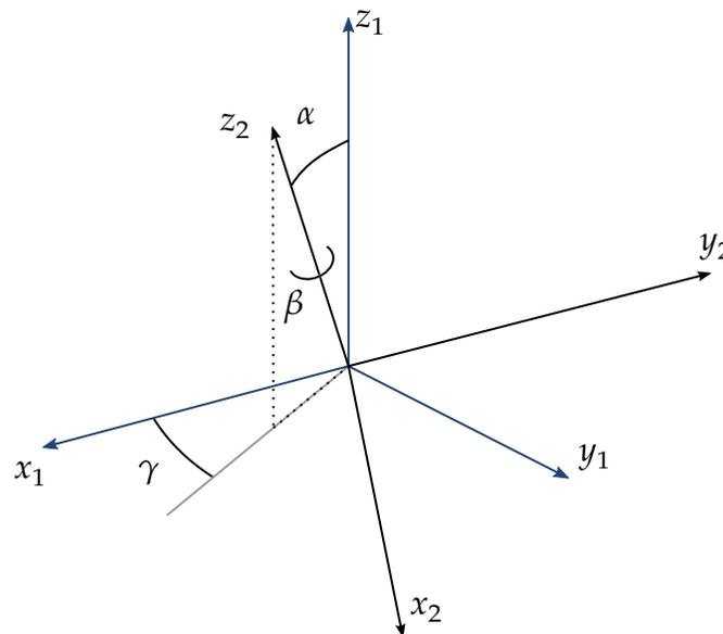
**Figure 10-31.** Flexion-torsion joint angles. If the initial positions of the local coordinate axes of the two rigid bodies connected by the joint do not coincide, the angles,  $\alpha$  and  $\gamma$ , are initialized and torques will develop instantaneously based on the defined load curves. The angle  $\beta$  is also initialized but no torque will develop about the local axis on which  $\beta$  is measured. Rather,  $\beta$  will be measured relative to the computed offset.
