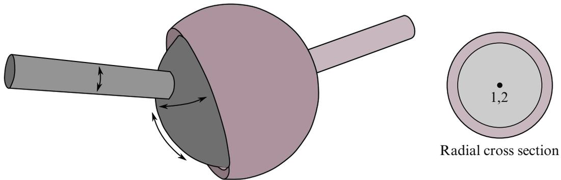
**Figure 10-16.** *Spherical joint.* The relative motion of the rigid bodies is constrained so that nodes which are initially coincident remain coincident. In the above figure the socket's node is not interior to the socket—LS-DYNA does not require that a rigid body's nodes be interior to the body.
