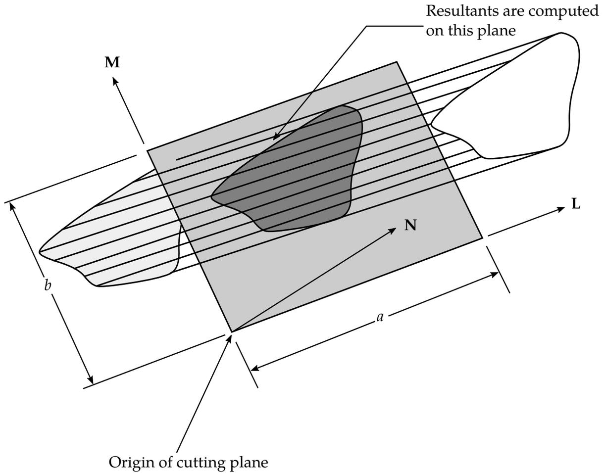
**Figure 16-2.** Definition of cutting plane for automatic definition of interface for cross-sectional forces. The automatic definition does not check for springs and dampers in the section. For best results the cutting plane should clearly pass through the middle of the elements, distributing them equally on either side. Elements that intersect the edges of the cutting plane are deleted from the cross-section.
