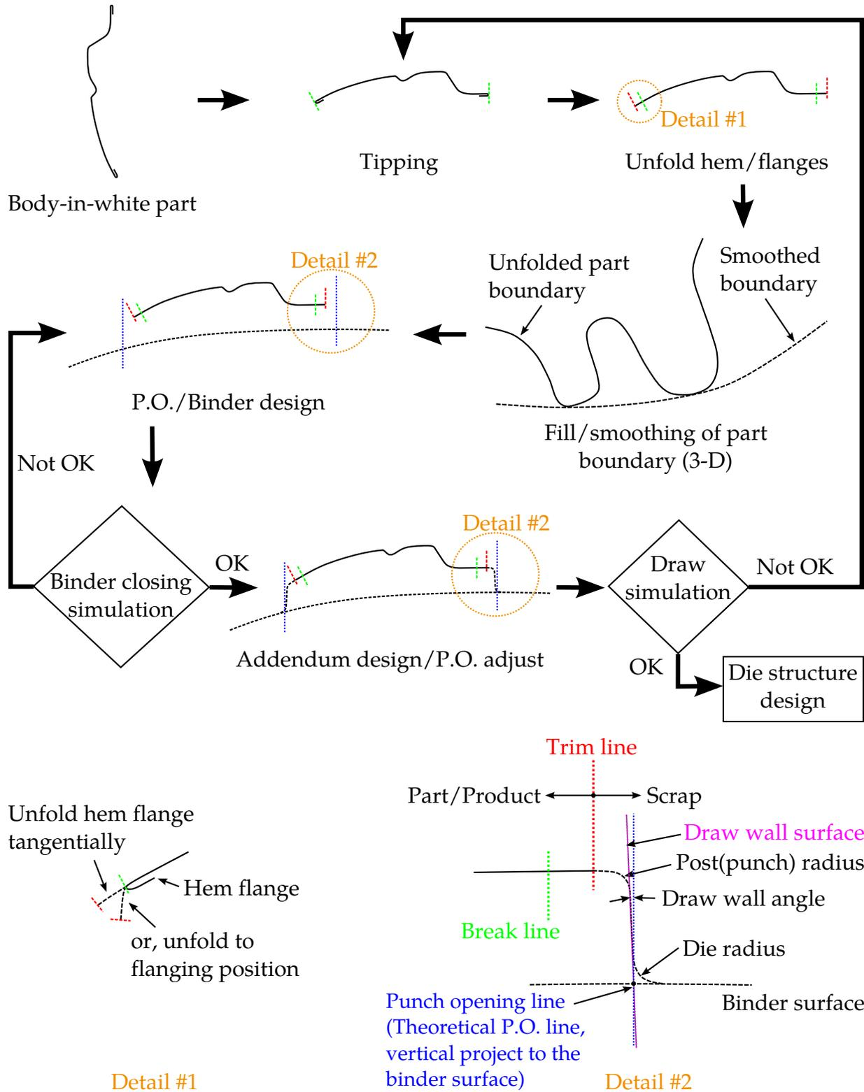
**Figure 68-1.** A typical draw die engineering process
