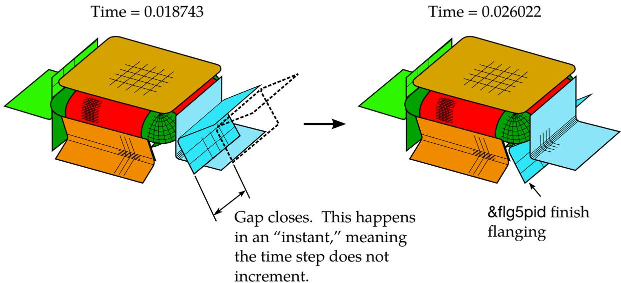
**Figure 11-25.** Closing the empty travel (left); flanging steel &flg5pid completes flanging process (right).
