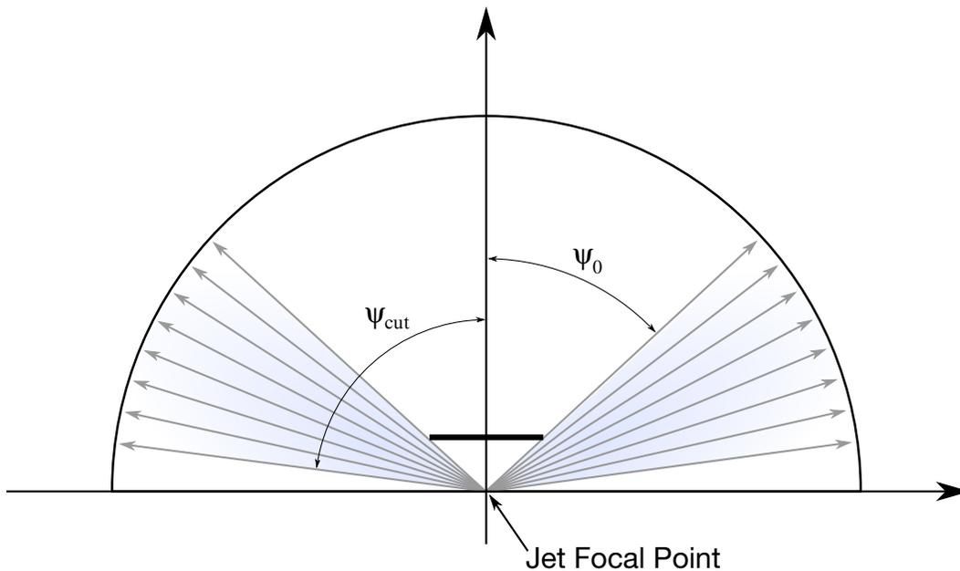
**Figure 3-4.** Multiple jet model for driver's side airbag. Typically,  $\psi_{cut}$  (see input ANGLE) is close to  $90^\circ$ . The angle  $\psi_0$  is included to indicate that there is some angle below which the jet is negligible; see [Figure 3-3](#).
