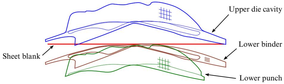
**Figure 11-20.** Initial parts auto-positioned at  $t = 0.0$ .
