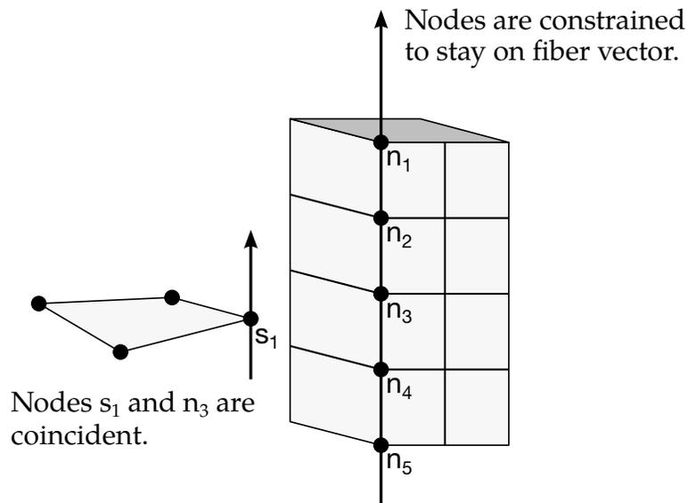
**Figure 10-41.** The interface between shell elements and solids ties a shell node,  $s_1$ , to a line of nodes on the solid elements,  $n_1$  to  $n_5$ . It is very important for the nodes to be aligned.
