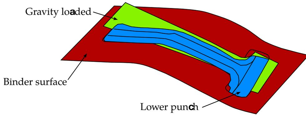
**Figure 29-8.** NUMISHEET 2008 B-pillar; Gravity loaded blank.
