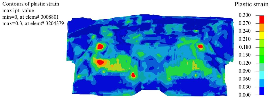
Figure 12-31. Effective plastic strain with EPSMAX = 0.3.
