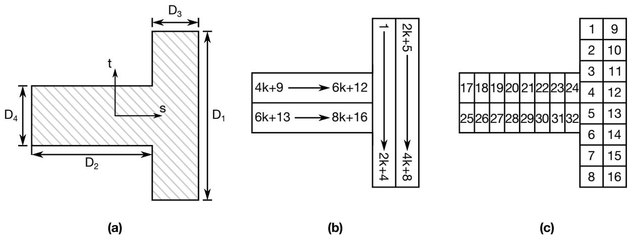
**Figure 28-16.** Type 14: T-Shape 2. (a) Cross section geometry. (b) Integration point numbering. (c) Example for  $k = 2$ .
