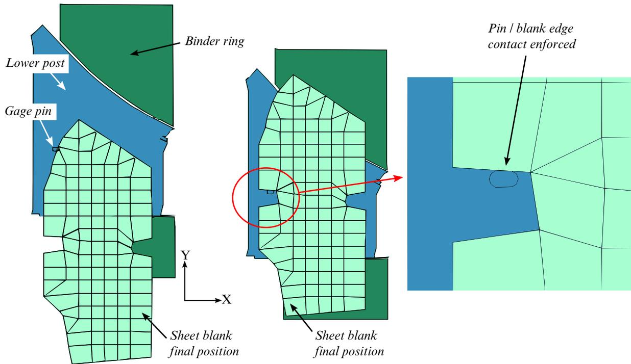
Gravity loading results without using SOFT=6; Pin/blank edge contact missed.
