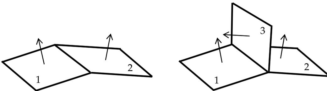
**Figure 17-38.** Bending in fabric, intended use of **\*DEFINE\_FABRIC\_ASSEMBLIES**. The numbers indicate the parts the elements belong to.
