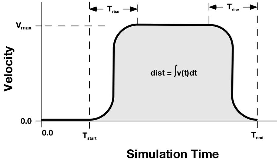
**Figure 17-21.** Smooth curve created automatically using \*DEFINE\_CURVE\_SMOOTH. This shape is commonly used to control velocity of tools in metal forming applications as shown in this figure but can also be used for other applications in place of any standard load curve.
