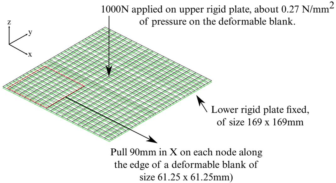
**Figure [17-44].** Boundary and loading conditions of a small test model.
