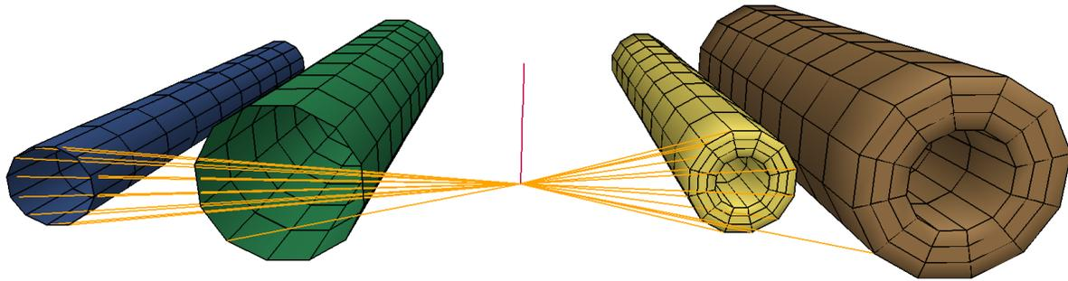
**Figure 17-54.** Automatically generated tubes using TYPE = 1, -1, 0, 2, and -2, from left to right. The beam tube ends are connected with \*CONSTRAINED\_NODAL\_RIGID\_BODY, which applies differently to the generated shell/solid tubes, depending on the sign of TYPE.
