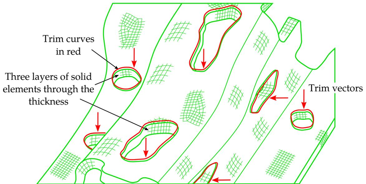
**Figure 17-30.** 2D trimming of solids using \*DEFINE\_CURVE\_TRIM\_2D
