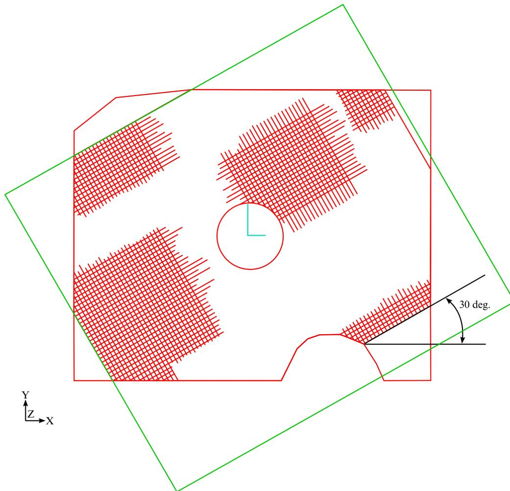
**Figure 17-41.** A rectangular blank mesh is generated in an angle (ANGLEX = 30) and trimmed into a developed blank shape, with an inner cutout defined by innerhole.iges and outline defined by outlines.iges. Note the blank mesh orientation is always parallel to the rectangular blank boundary.
