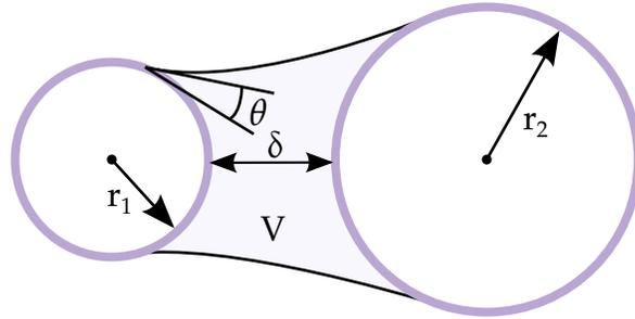
**Figure 12-15.** Schematic representation of capillary force model.
