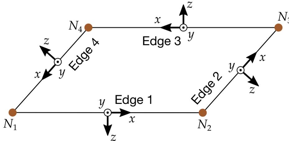
**Figure 31-14.** Local coordinates system for edge load.
