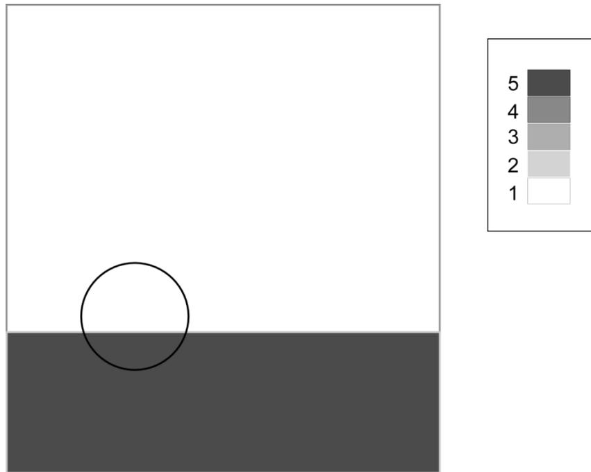
**Figure 27-4.** Before the 1<sup>st</sup> “filling action” the whole ALE mesh of part H1 is filled with AMMG 1 (white). After the 1<sup>st</sup> “filling action”, AMMG 5 fills below the specified plane.
