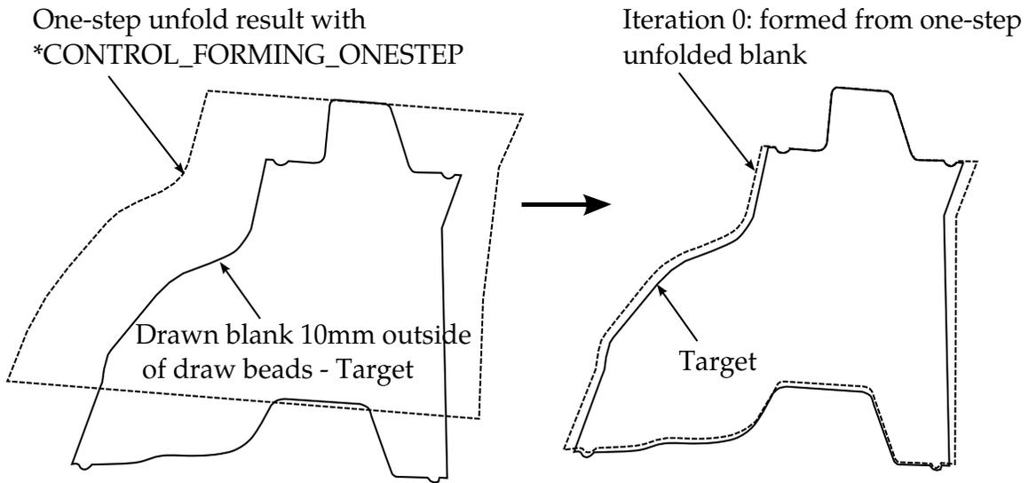
**Figure 29-12.** Initial blank calculation and baseline formed blank.
