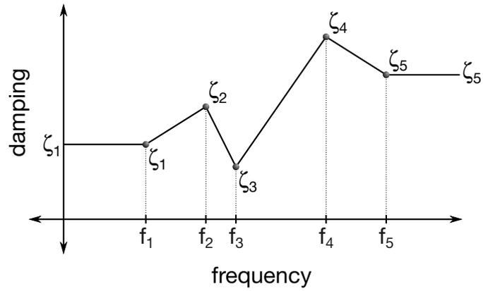
**Figure 12-84.** Schematic illustration of frequency range damping.
