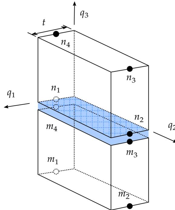
**Figure 39-24.** Cohesive interface coordinate system for element type +/-29
