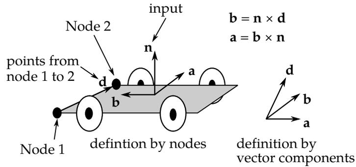
**Figure 38-4.** Definition of orthotropic friction vectors. The two methods of defining the vector, **d**, are shown. If vector **d** is defined by nodes 1 and 2, the local coordinate system may rotate with the body which contains the nodes; otherwise, **d** is fixed in space, thus on the rigid wall, and the local system is stationary.
