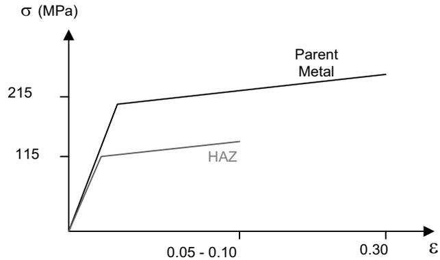
**Fig 8** Parent metal and Heat Affected Zone (HAZ) material model curves
