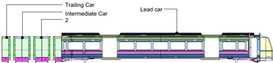
**Fig 6** 3D analysis model with 'simplified' intermediate and trailing cars
