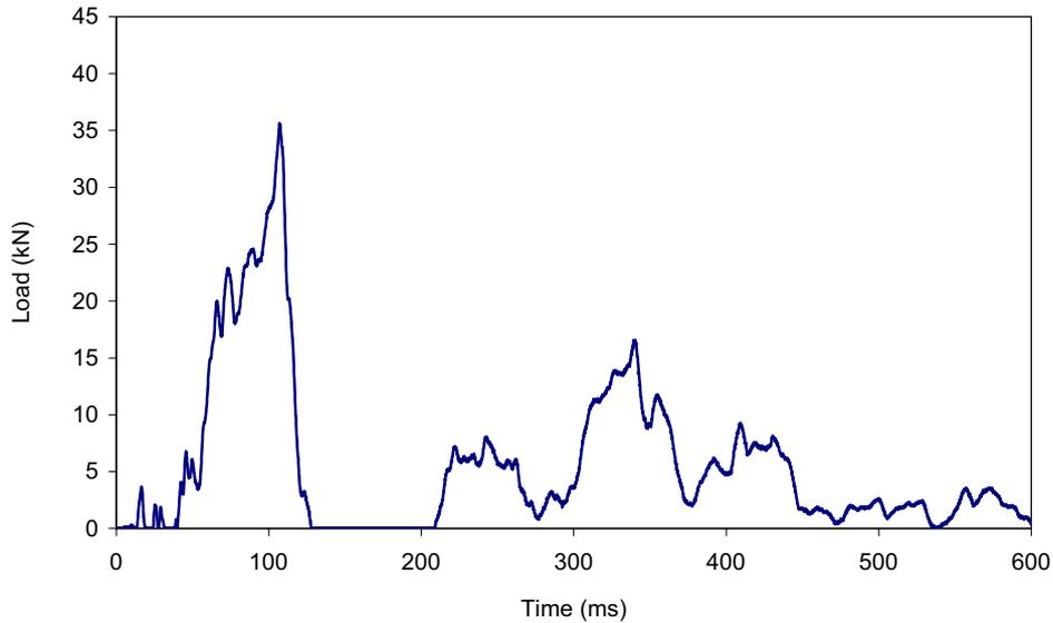
**Fig 13** Load/time history for bodyside spotweld, representing Huckbolt™ connection
