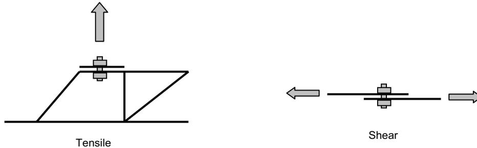
**Fig 10** Tensile and shear test configurations for Huckbolt™ failure load calibration
