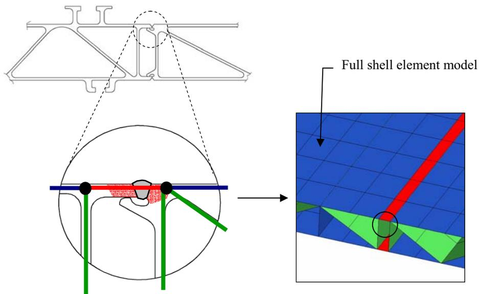
**Fig 7** Section showing geometry, weld location and structure 'as modelled'
