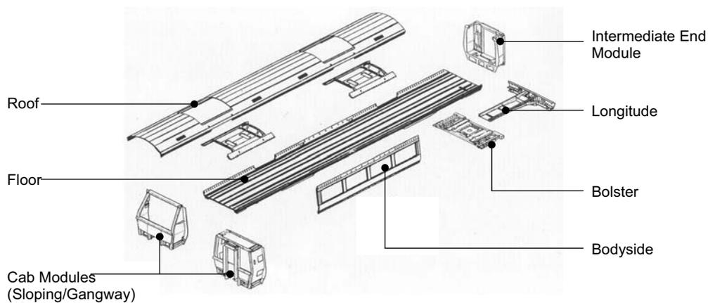
**Fig 1** Components of a 'Complete Knock Down' (CKD) vehicle
