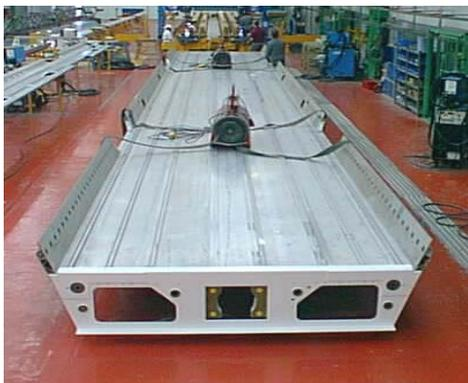
**Fig 2**    Current vehicle floor structure
