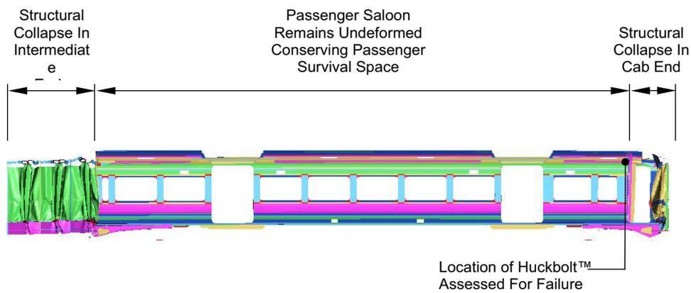
**Fig 11** Multiple unit post 60 km/h closing speed collision - Displaced shape
