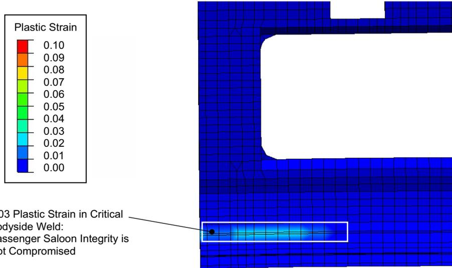
**Fig 12** Plastic strain in bodyside weld located at front end of leading car
