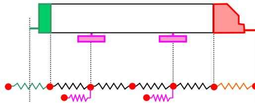
**Fig 5** Spring element representation of cab end car for 1D analysis
