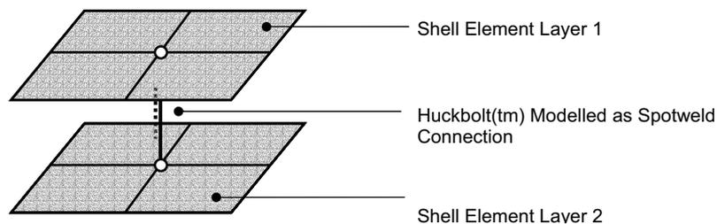
**Fig 9** Schematic of spotwelded shells representing Huckbolt™ connection
