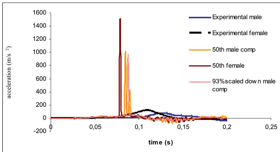
**Figure 2 Head horizontal acceleration**
