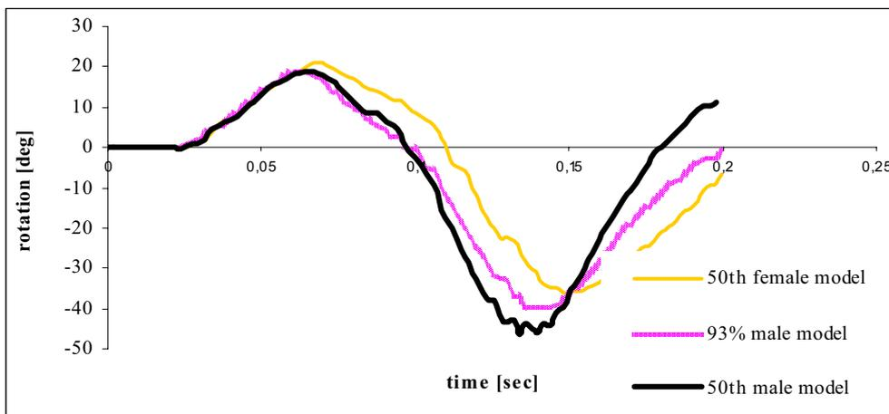
Figure 4 Head rotation relative to C3
