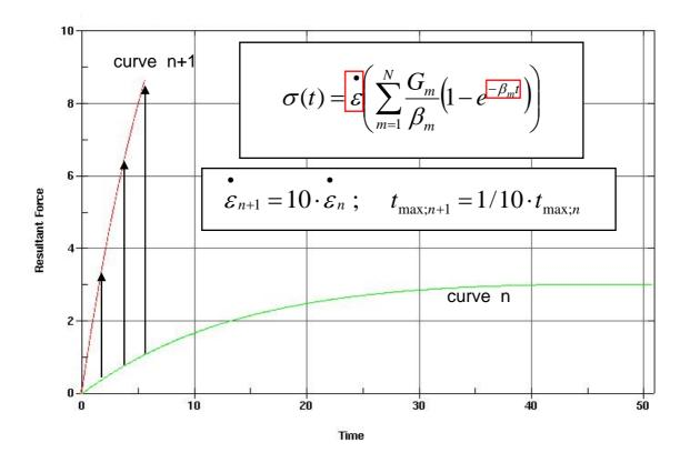
Figure 4: The equation  $\sigma(t)$  represents the viscous stress contribution derived from equation (2) with  $\dot{\varepsilon} = const$ . The arrows illustrate the linear mapping of viscous stress from curve n to curve n+1. For both curves the maximal strain is approximately 10%.
