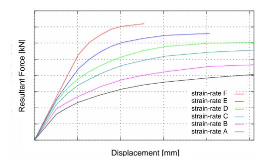
Figure 1: HDPE tension tests [6] with different strain rates; 5mm elongation corresponds to approximately 10% strain; strain rates vary from 2.0e-3 to 1.5e+2 [1/s]
