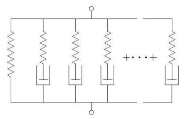
Figure 2: Generalized Maxwell model used in LS-DYNA (\*MAT\_OGDEN\_RUBBER). A non-linear spring is placed in series with up to six Maxwell elements. For incompressible materials only deviatoric strains are possible so that only the shear moduli, Gi, are considered.
