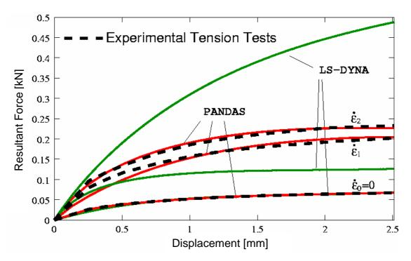
Figure 3: The capability of the visco-elastic formulations in LS-DYNA and PANDAS to capture tension tests with different constant strain-rates,  $\dot{\varepsilon}_2 = 10 * \dot{\varepsilon}_1$ . 2.5mm elongation corresponds to approximately 10% strain (only half of the specimen is considered)
