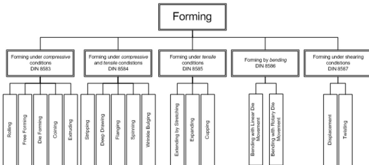
Figure 1: Subdivision of manufacturing processes according to DIN 8582
