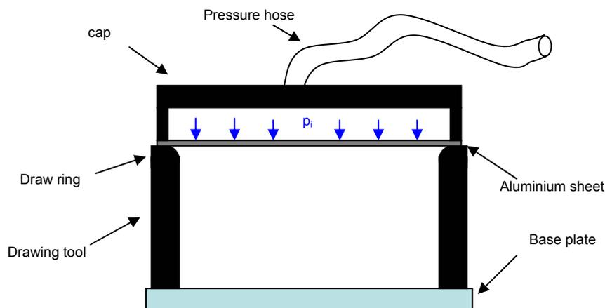
Figure 4: The concept of the experimental tool for the warm metal forming process
