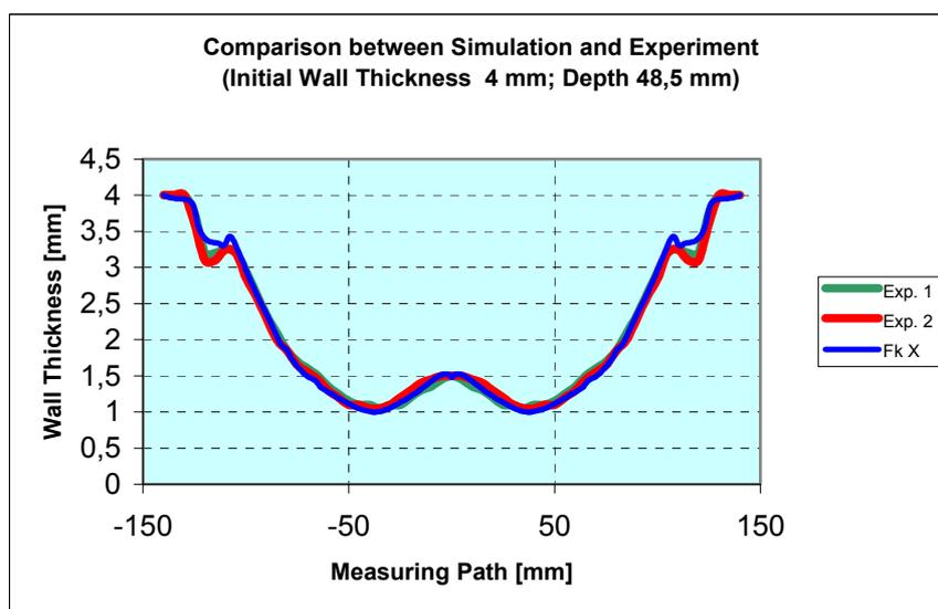
Figure 7: Comparison between the FEA simulation and the experimental wall thickness
