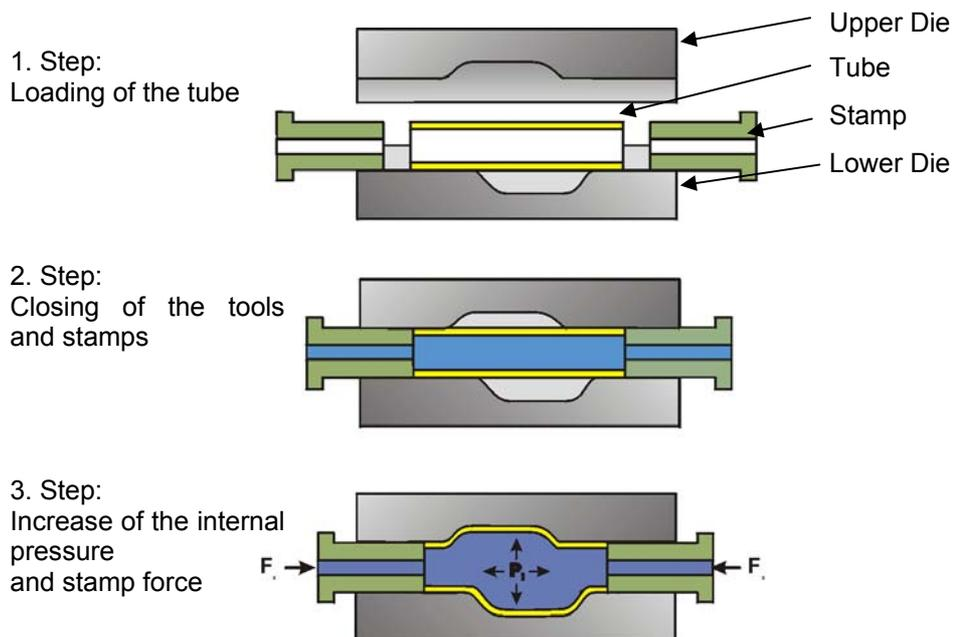
Figure 3: Operation sequence of the hydroforming process of a tube
