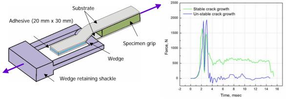
Figure 5: impact peel test and results for a crash stabilized and a non-stabilized adhesive
