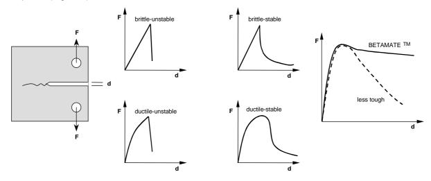
Figure 2: Adhesive CTS: crack initiation and propagation of different adhesive types
