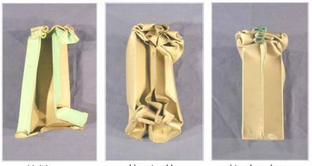
a) brittle epoxy b) spot-welds c) toughened epoxy Figure 3: Test results of dynamic drop-tower tests on a double hat section profile using a brittle adhesive, spot-welds and the crash stable BETAMATE 1496
