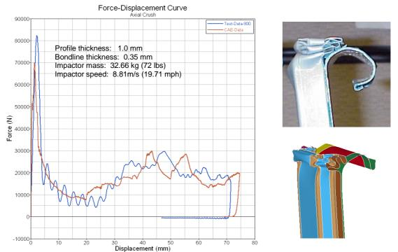
Figure 9: Force deflection results for the axial crush of a hat section closed by bonding with a steel plate
