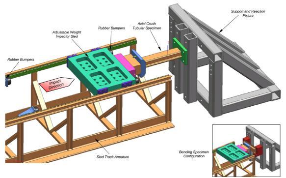
Figure 8: Test setup for the adhesive model application tests for axial crush and for a bending impact (small picture)
