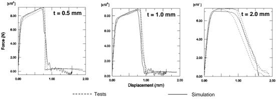
Figure 4: Experimental results for thick lap shear specimen tests of a crash stable adhesive and the simulation response using a detailed Gurson type material model, see Wocke [2], [3].
