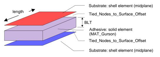
Figure 7: Macro-element approach – Connecting the adhesive representing solid element to the substrate representing mid-plane shells
