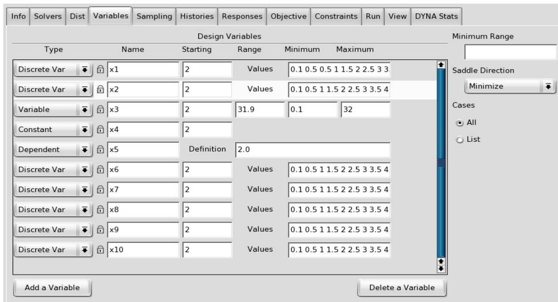
Fig 2: The variables panel showing the specification of discrete variables
