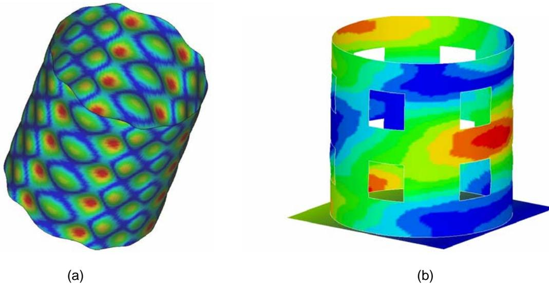
Fig 1: Geometric perturbations of a cylinder based on (a) harmonic functions and (b) Karhunen-Loève imperfections
