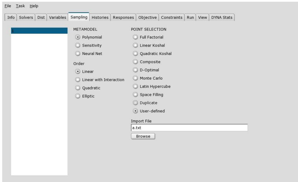
Fig. 9: The user-defined sampling option allows the importing of experimental design tables
