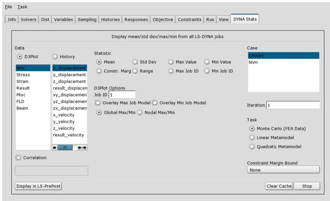
Fig. 3: The DYNA Statistics panel. The panel is used to investigate the variation of d3plot results and LS-OPT histories. The procedure includes tight integrated with LS-PREPOST visualization. Instability analysis and display of probabilistic (six-sigma) safety margins are also possible.
