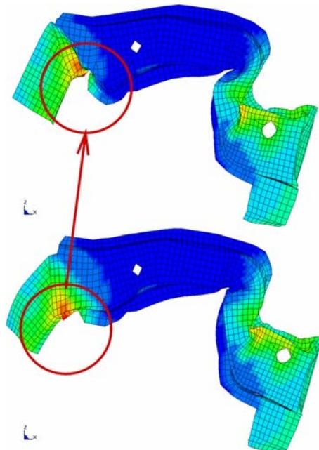
Fig. 4: Standard deviation of displacement residuals superimposed on outlier deformed states.
