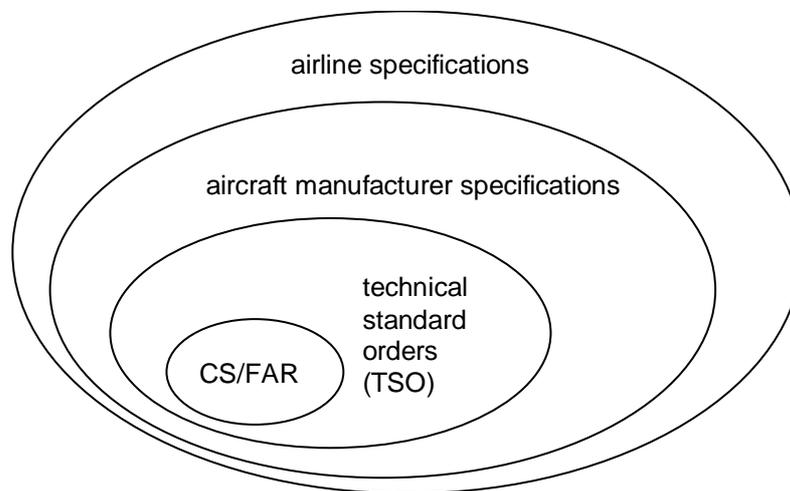
**Fig. 2:** Overview of relevant regulations for passenger seat development
