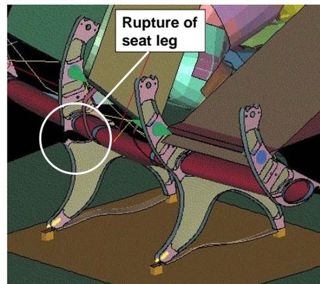
Fig. 25: Seat leg rupture in the 16g forward load case
