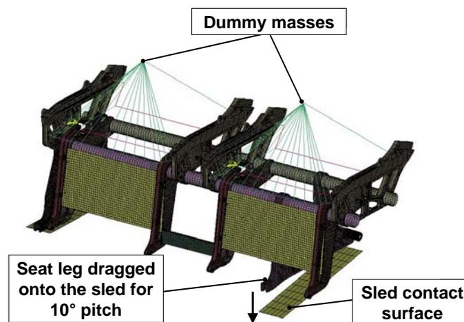
Fig. 21: Pre-deformation of the BC seat
