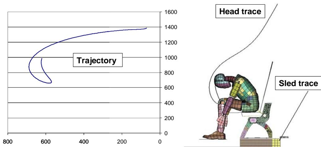
Fig. 23: Traces and trajectory for a single head node, processed in LS-PrePost and MS-Excel
