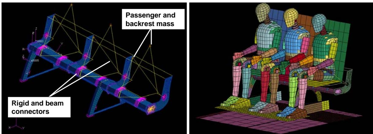
Fig. 11: AECS finite element model: MSC Nastran (left) and LS-Dyna (right)
