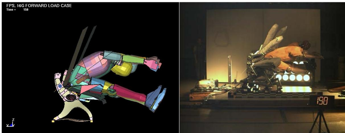
Fig. 24: 16g forward test of the FPS: LS-Dyna calculation (left) and hardware test (right)
