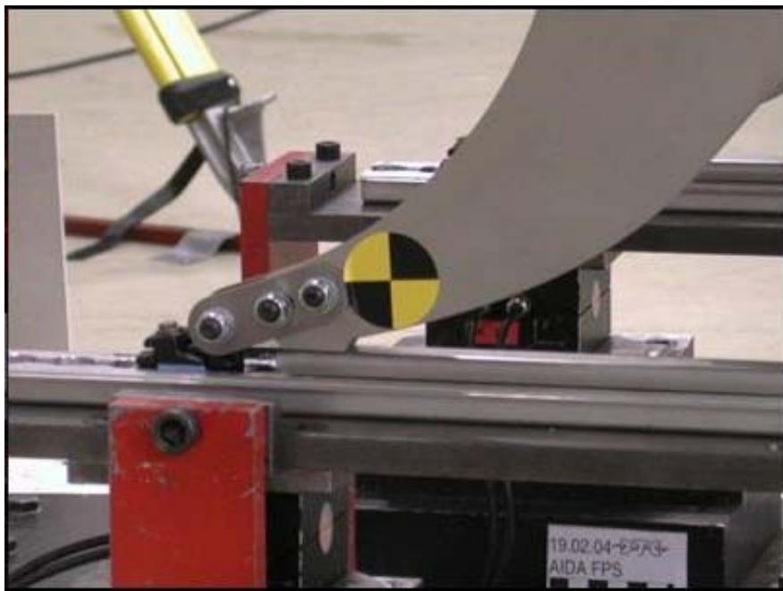
**Fig. 7:** Double stud for the seat attachment on the aircraft seat track
