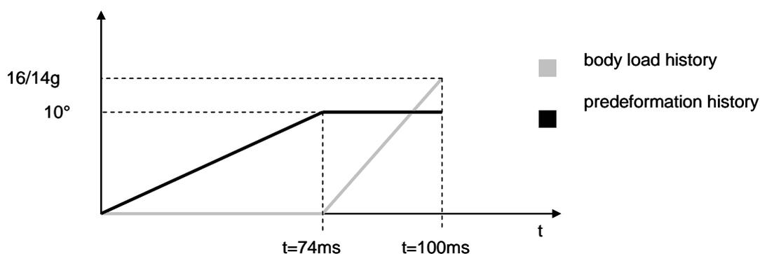
Fig. 22: History of synchronous pre-deformation and crash loading in an explicit calculation for the BC seat
