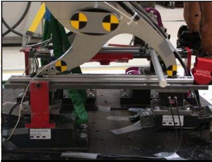
**Fig. 6:** Seat attachment on the aircraft seat tracks
