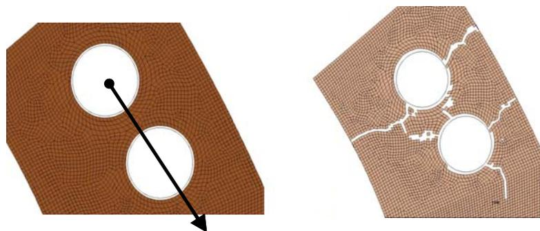
Fig. 18: Prescribed (assumed) bolt displacement  $u(t) \sim t$  in direction of arrow (left) and initial crack propagation (right)
