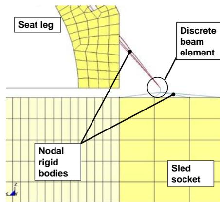
**Fig. 14:** Substitute element for rear seat leg attachment
