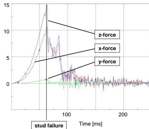
**Fig. 15:** Force components in the discrete beam element (left rear leg) for AECS forward load case in kN
