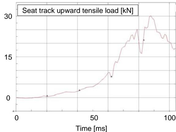
**Fig. 12:** Sled socket upward load (sae1000 filtered) for the FPS forward load case
