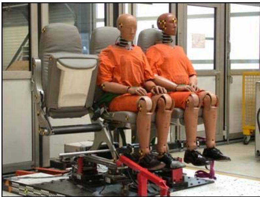
Fig. 5: 16g forward structural test setup for seat certification
