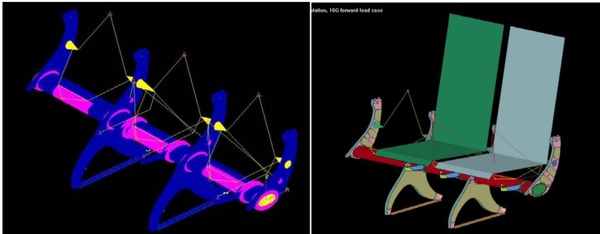
Fig. 10: FPS finite element model: MSC Nastran (left) and LS-Dyna (right)
