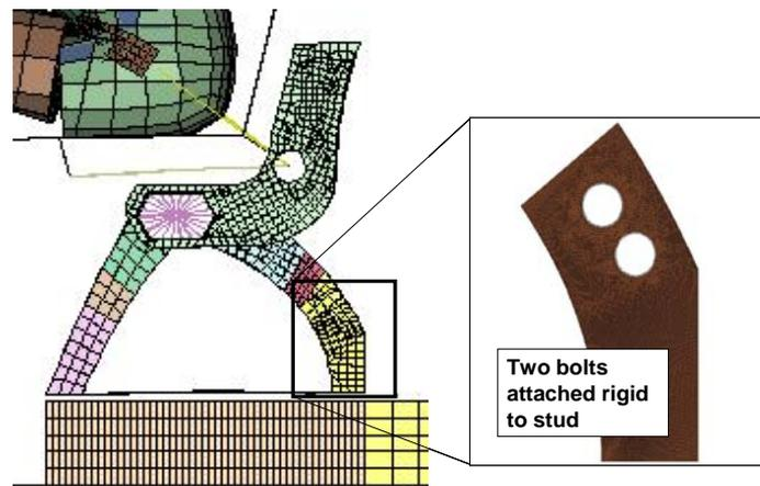
Fig. 16: Deformation element making use of two rigid bolts
