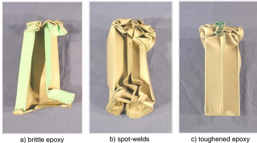
Figure 3: Test results of dynamic drop-tower tests on a double hat section profile using a brittle adhesive, spot-welds and the crash stable BETAMATE 1496
