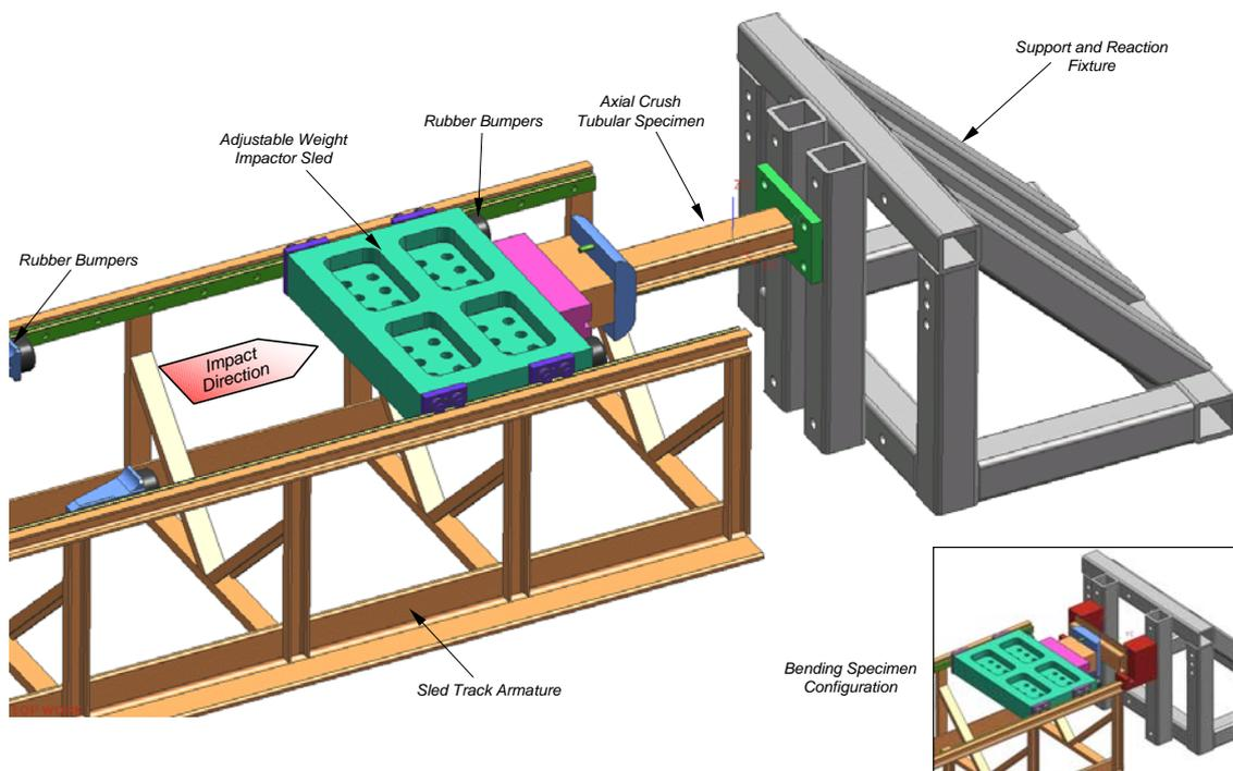
Figure 8: Test setup for the adhesive model application tests for axial crush and for a bending impact (small picture)
