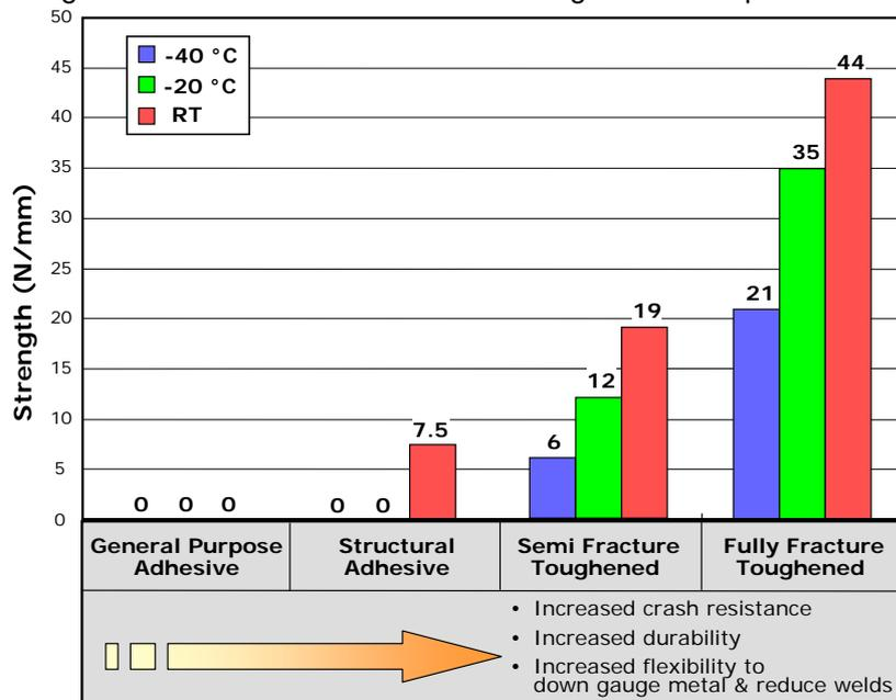
Figure 6: Impact peel strength of different adhesives including low temperature behavior
