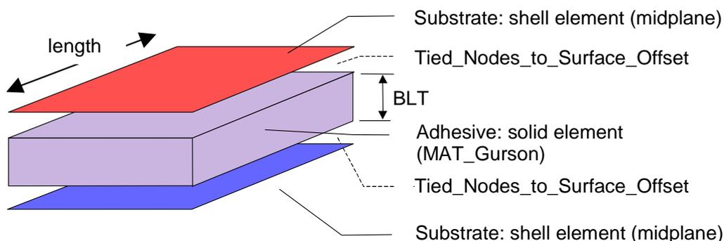
Figure 7: Macro-element approach – Connecting the adhesive representing solid element to the substrate representing mid-plane shells
