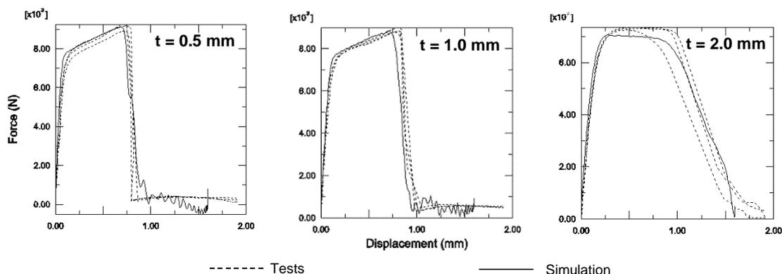
Figure 4: Experimental results for thick lap shear specimen tests of a crash stable adhesive and the simulation response using a detailed Gurson type material model, see Wocke [2], [3].
