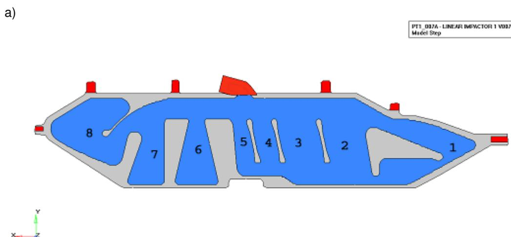
Figure 1: a) Curtain airbag. Blue- airbag chambers 1-8, grey – connecting fabric, red – fixation.
