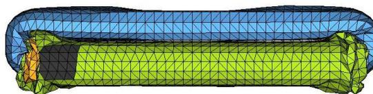
Figure 6: DKAB vent hole modelling for CPM simulation
