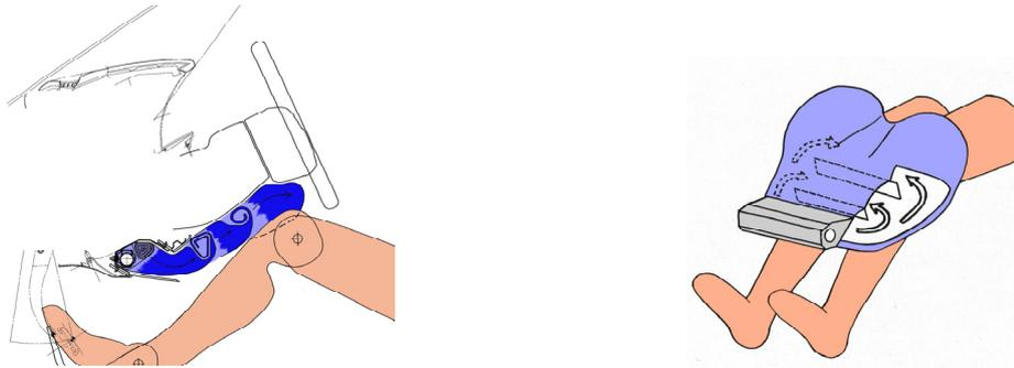
(a) Deployment along dummy leg contour
