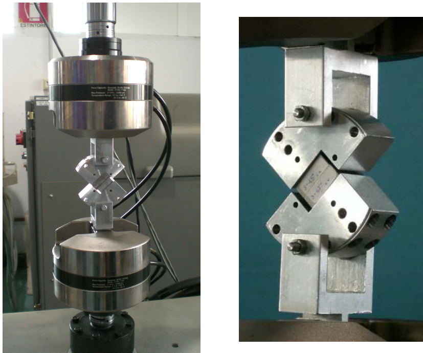
Figure 1: The devices used for the tests on the rivets (inclination angle 45°)
