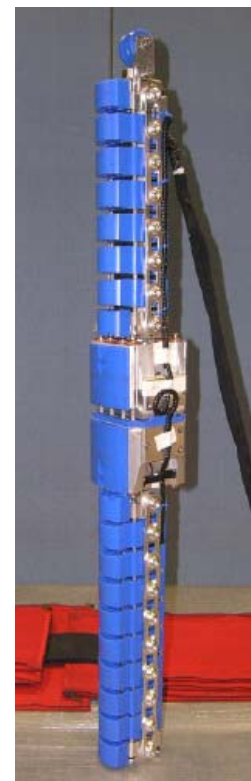
Figure 2: Flex-GT internal structure: LS-DYNA model and a physical impactor
