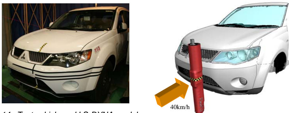
Figure 14: Test vehicle and LS-DYNA model
