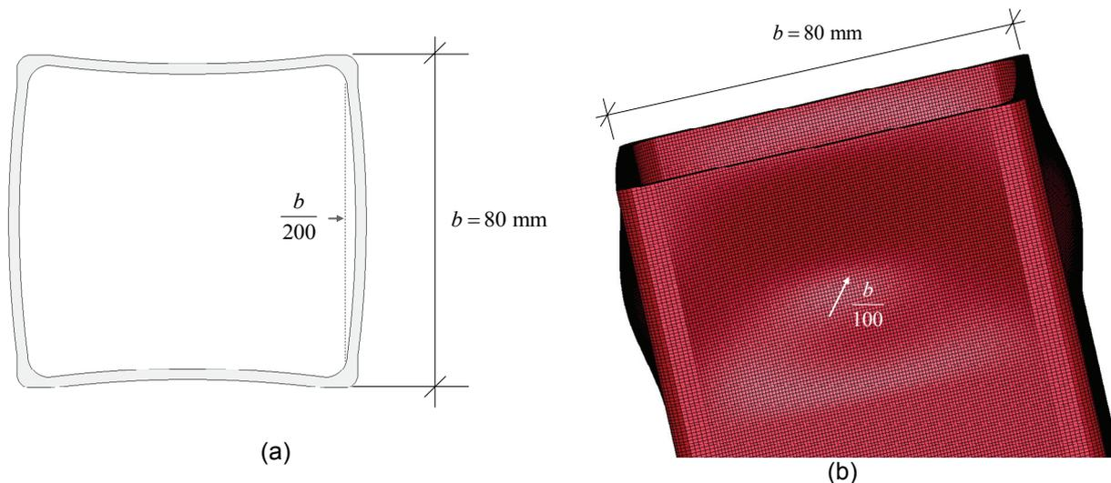
Figure 1. (a) Cross-section with amplified imperfections; (b) Illustration of trigger
