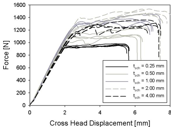
Figure 2: Measured force-displacement curves of TDCB tests - specimen type 1
