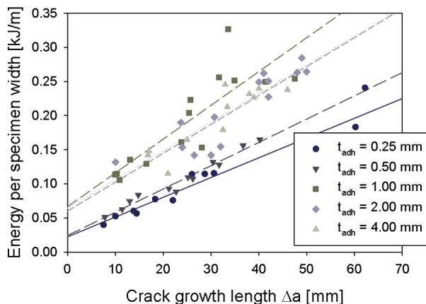
Figure 3: TDCB specimen type 2:  $W_{tot}$  vs.  $\Delta a$
