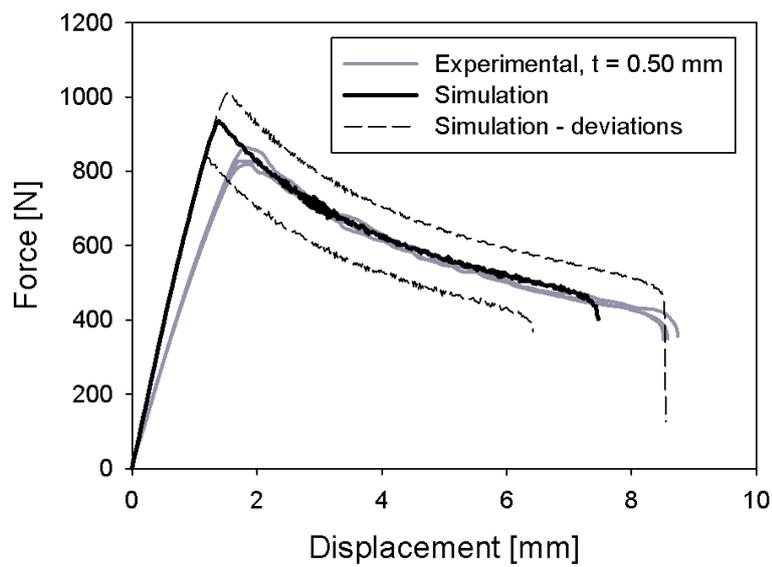
Figure 10: ATDCB tests: comparison between experimental and numerical data,  $t_{adh} = 0.5$  mm
