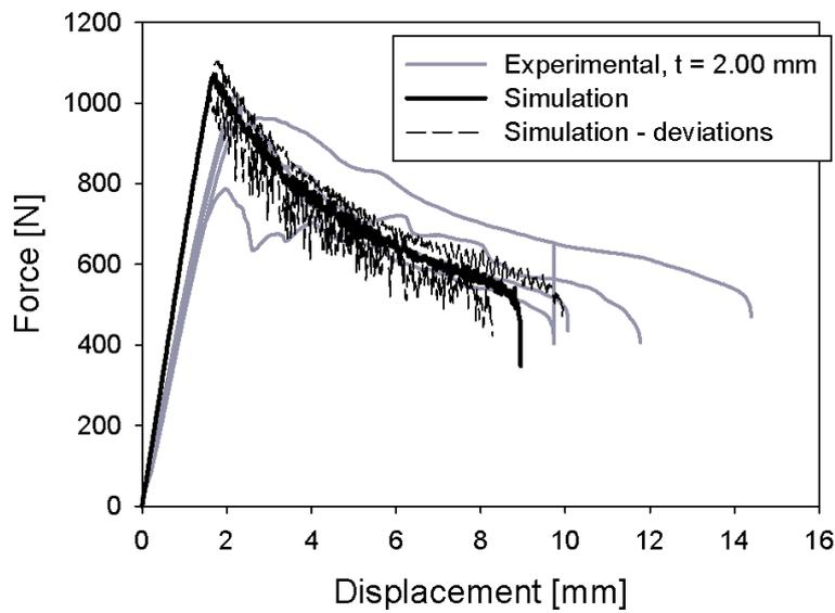
Figure 12: ATDCB tests: comparison between experimental and numerical data,  $t_{adh} = 2.0\text{ mm}$
