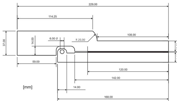
Figure 5: Dimensions of the ELSJ specimen
