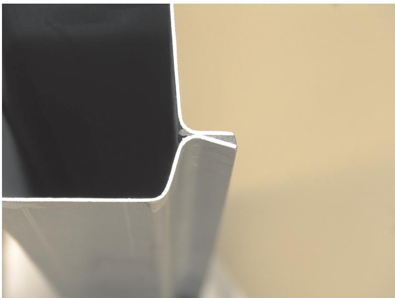
Figure 14: Crash box: Detail of bonded flange connection with adhesive layer of varying thickness
