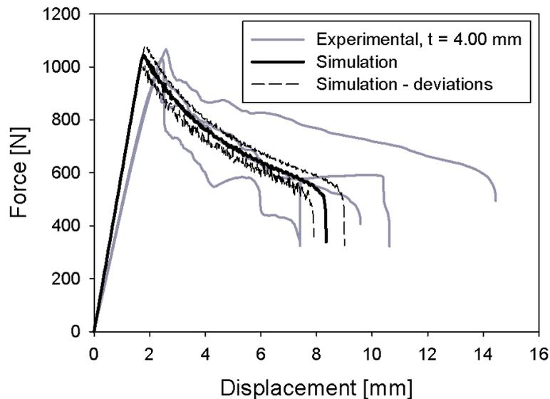
Figure 13: ATDCB tests: comparison between experimental and numerical data,  $t_{adh} = 4.0$  mm
