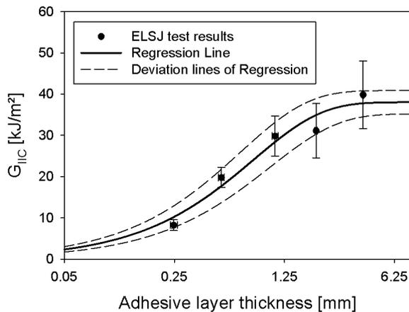
Figure 7: Critical energy release rate  $G_{IIc}$  vs. adhesive layer thickness  $t_{adh}$
