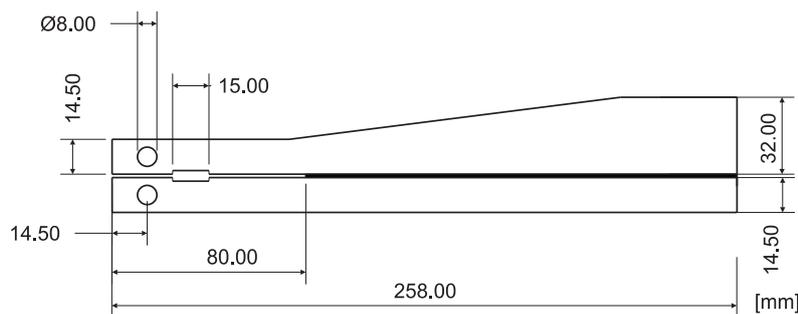
Figure 8: Dimensions of an ATDCB specimen
