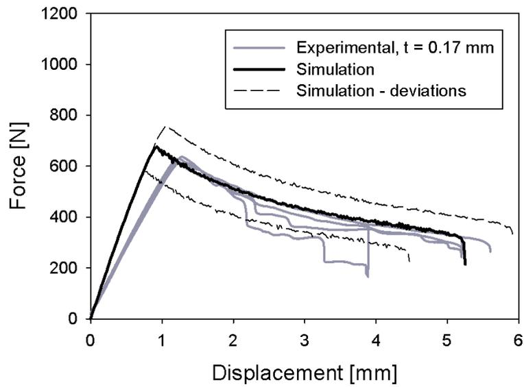
Figure 9: ATDCB tests: comparison between experimental and numerical data,  $t_{adh} = 0.17$  mm
