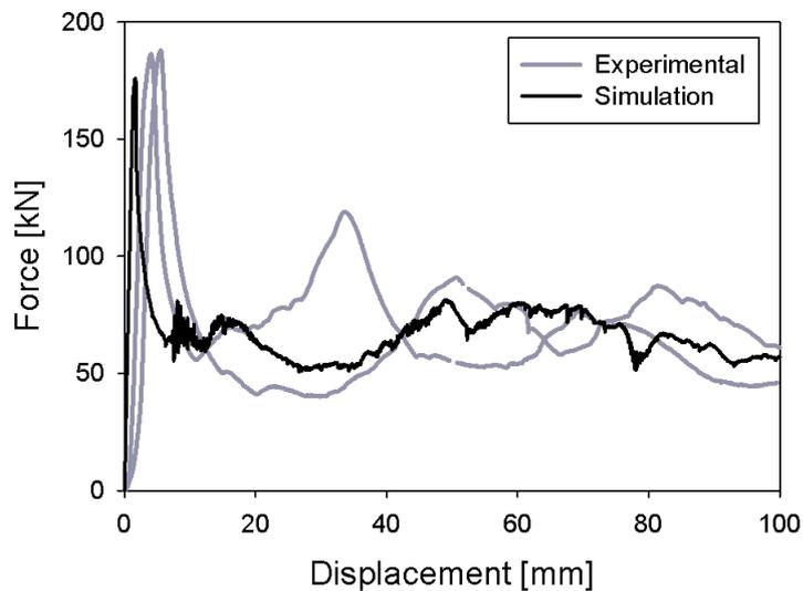
Figure 15: Crash box tests: Experimental and numerical force-displacement-curves
