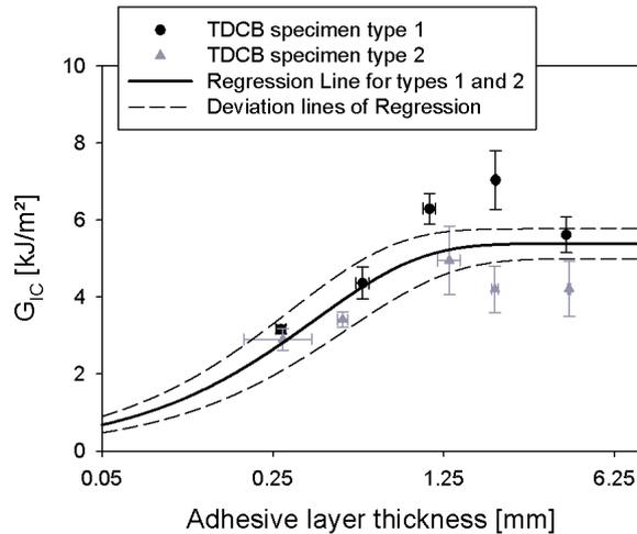
Figure 4: Critical energy release rate  $G_{IC}$  vs. adhesive layer thickness  $t_{adh}$
