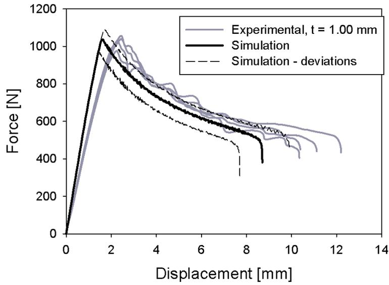
Figure 11: ATDCB tests: comparison between experimental and numerical data,  $t_{adh} = 1.0\text{ mm}$
