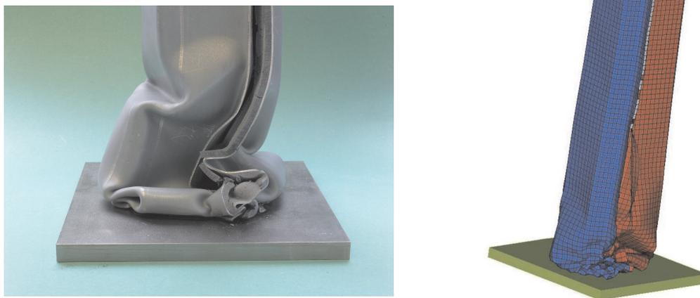
Figure 16: Crash box tests: Comparison of deformed shapes (left: experimental, right: simulation)
