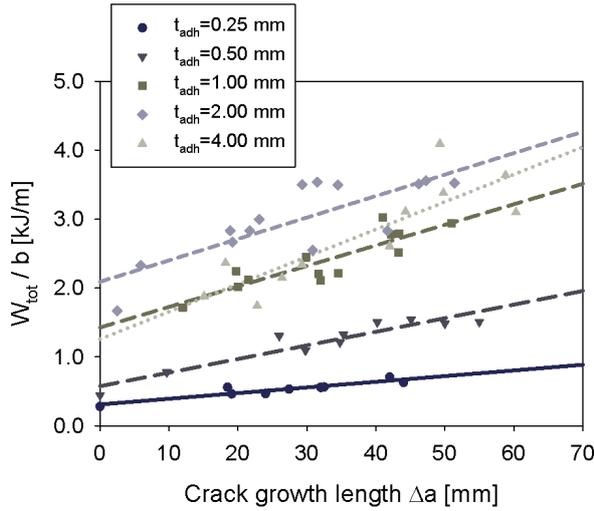
Figure 6: ELSJ tests:  $W_{tot}$  vs.  $\Delta a$
