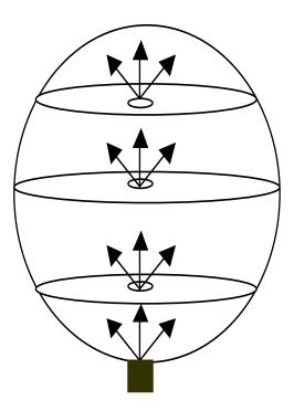
Fig.8: Multiple Chambered Airbag
