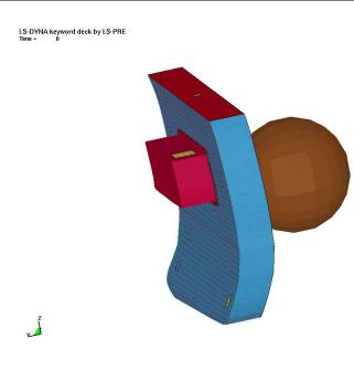
Fig.5: Rigid Ball Impact onto a Side Door
