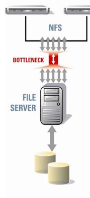
NAS Network Attached Storage. Serial I/O bottleneck.
