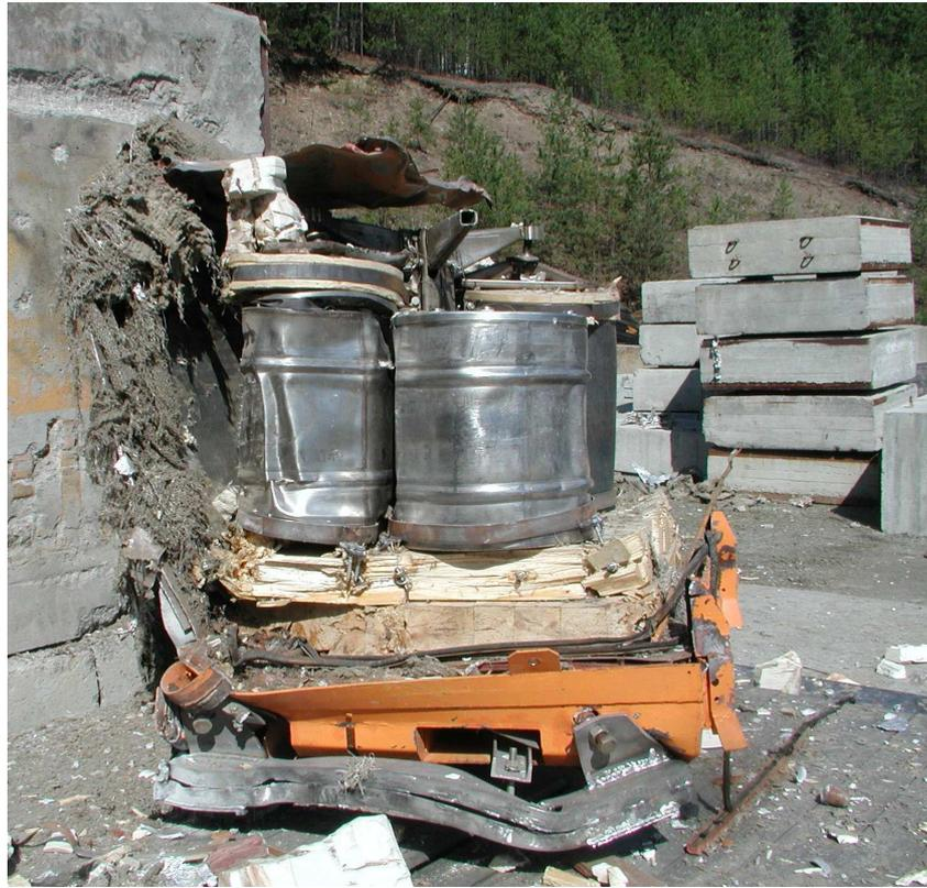
Fig. 10 Appearance of packages in TPB content after experiment
