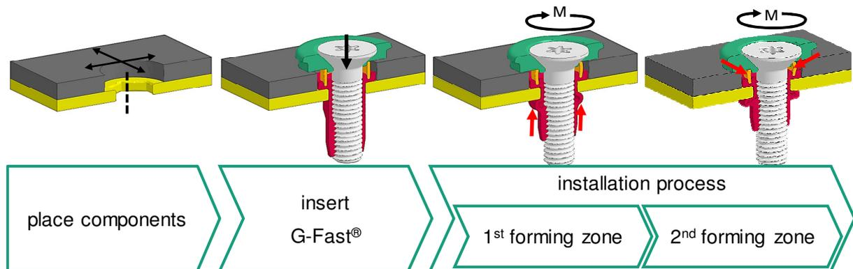
Fig.5: Installation process of the blind rivet nut screw system
