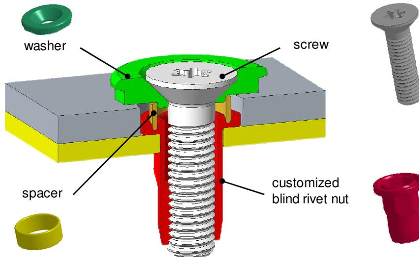
Fig.4: Cross section and 3D-parts of a blind rivet nut screw system
