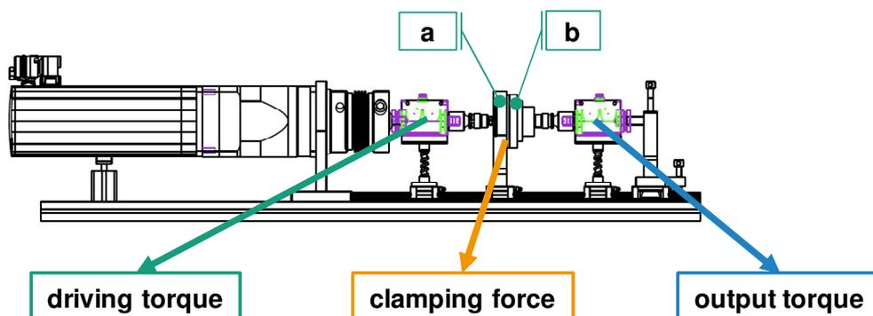
Fig.7: Test setup according to DIN EN ISO 16047:2013
