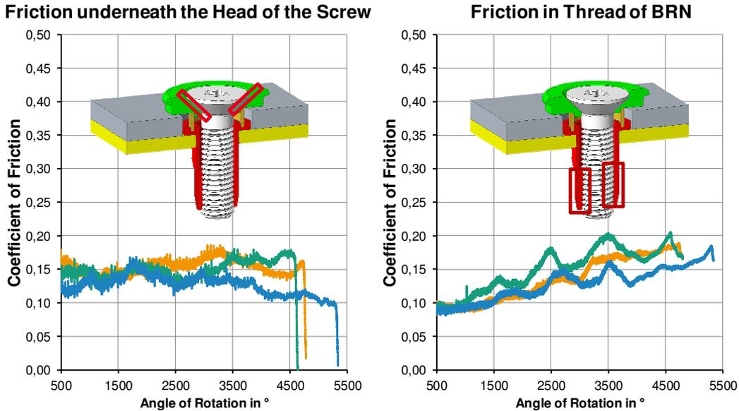
Fig.8: Results of friction properties of blind rivet nut part of the BRNS and head of the screw
