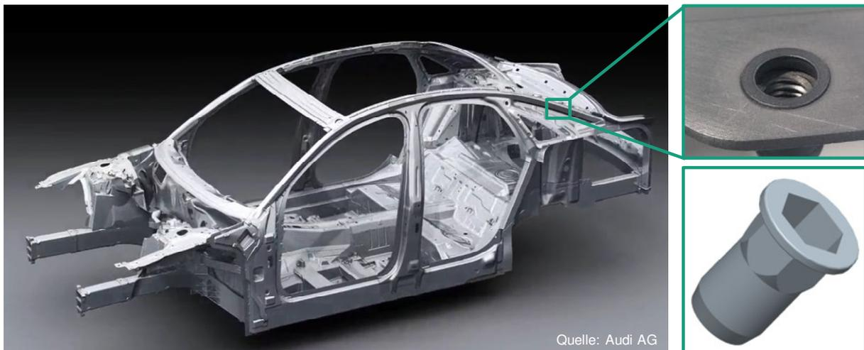
Fig.1: Blind rivet nut in a car body, Audi Space Frame, Audi A8
