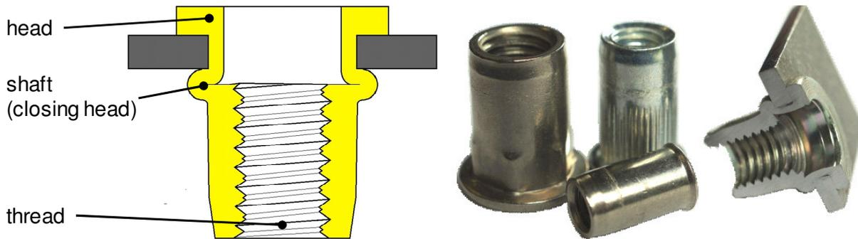
Fig.2: Structure of a blind rivet nut and various BRNs
