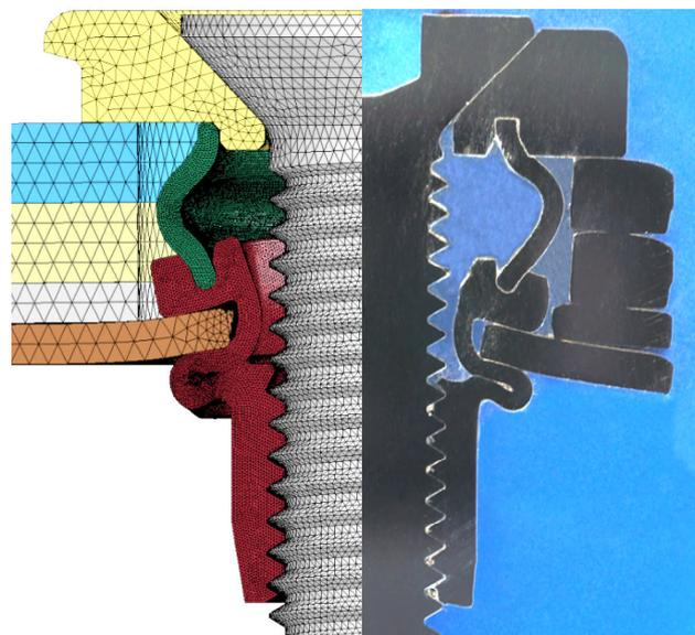
Fig.10: Result for a specific BRNS Configuration
