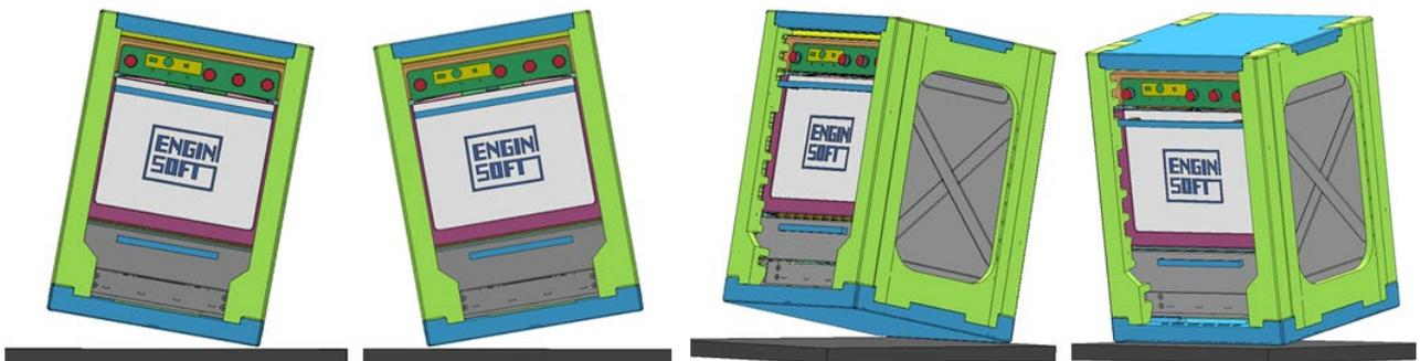
Fig.4: Impact sequence – right, left, rear and front, respectively.
